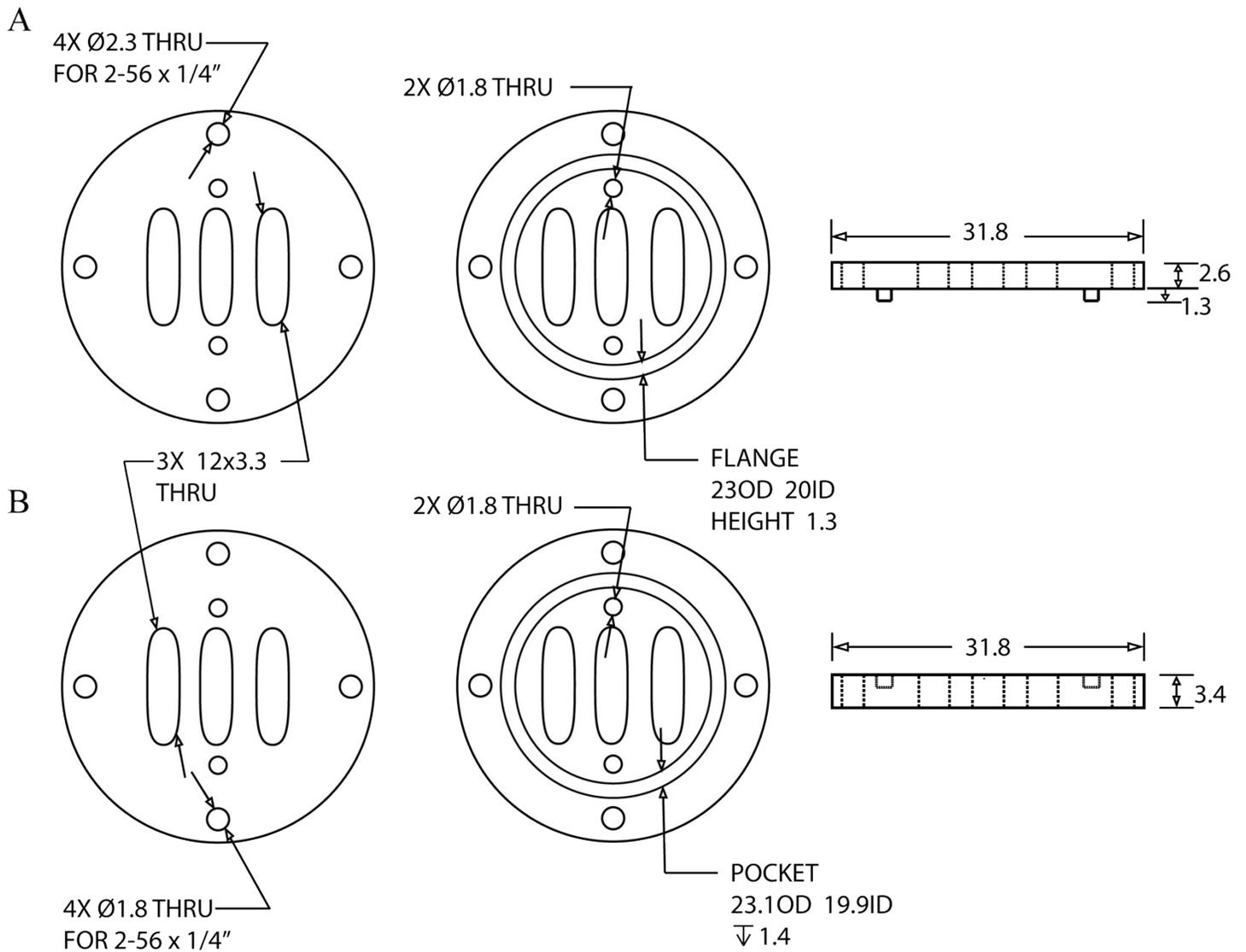
**Figure S3.** Detailed schematic showing each side of the A) top and B) bottom halves of the stainless steel holder used in the paper-based chemotaxis assay. Each holder contained three 12 x 3.3 mm channels, four (2.3 mm) holes for combining both halves with four (2-56 x 1/4 in.) screws, and two (1.8 mm) holes for alignment purposes during assay assembly. All values are in units of millimeters unless otherwise indicated.
