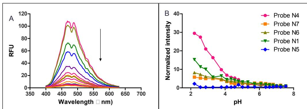
Figure S3. A: Fluorescent emission spectra changes of probe N4 (10 μM) in Britton-Robinson buffer at different pH values; B: Fluorescent intensity (normalized based on the last point which is seen as 1) changes of probe N1, N4-7 at their maximum wavelength, 460 nm for probe N4, 6, 7 (excited at 355 nm), 396 nm for probe N1, (excited at 355 nm), 545 nm for probe N5, (excited at 440 nm) with pH values.
