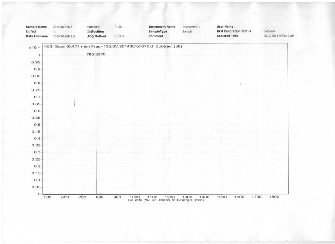
Figure S24. ESI-MS spectra of probe N7
