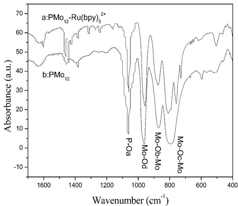
FTIR spectra of  $\text{PMo}_{12}\text{-Ru(bpy)}_3^{2+}$  (curve a) and  $\text{PMo}_{12}$  (curve b)
