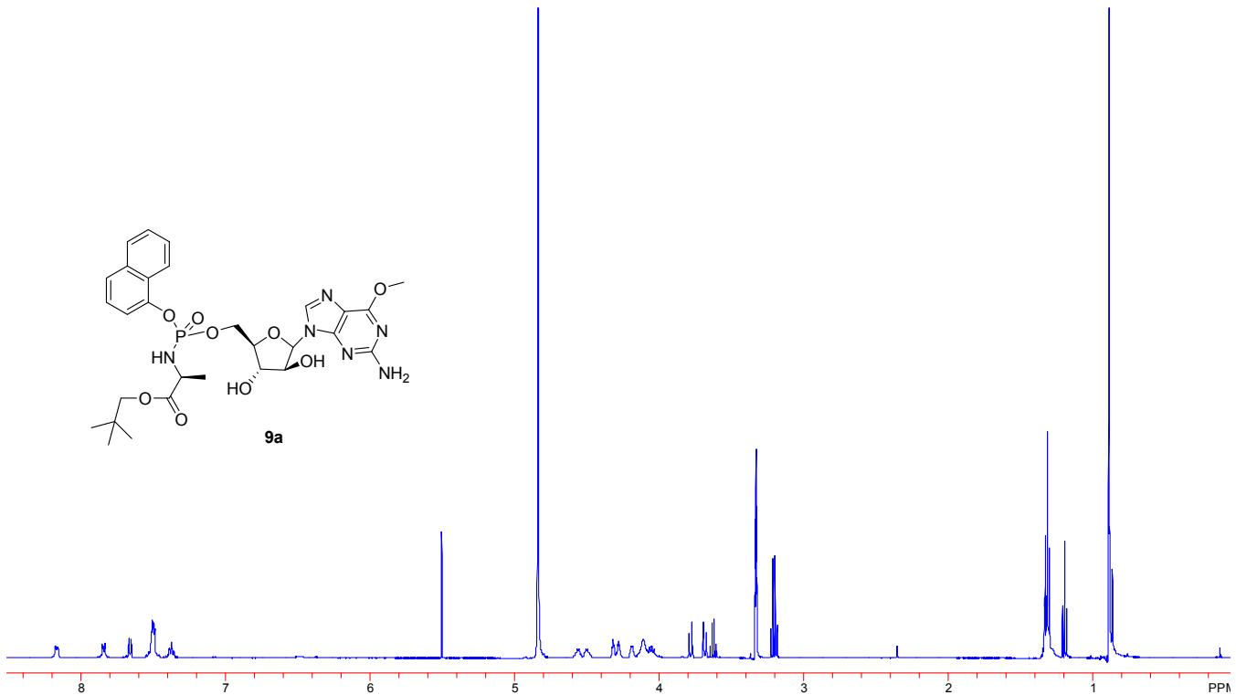
**Fig.52.**  $^1\text{H}$ NMR ( $\text{CD}_3\text{OD}$ , 500 MHz) of 2-amino-6-methoxy-9-( $\beta$ -D -arabinofuranosyl) purine 5'-O-[ $\alpha$ -naphthyl-(2,2-dimethylpropoxy-L -alaninyl)] phosphate **9a**.
