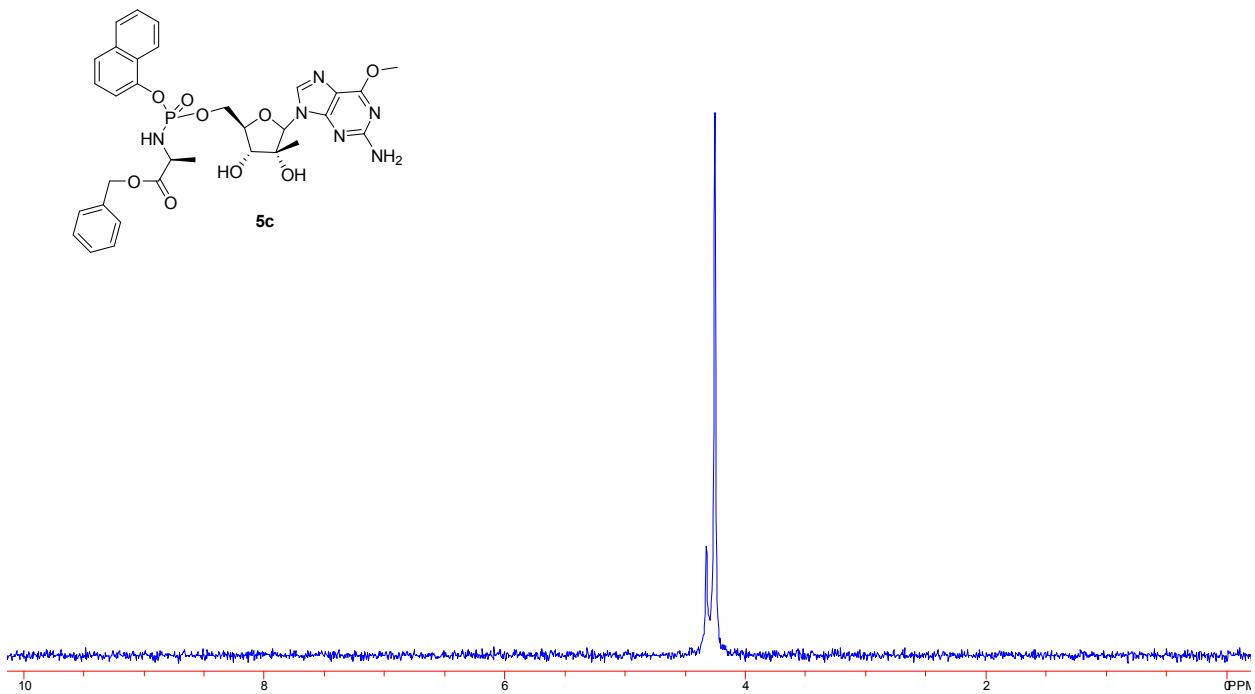
**Fig.30.**  $^{31}\text{P}$ NMR ( $\text{CD}_3\text{OD}$ , 202 MHz) of 2-amino-6-methoxy-9-(2'-C-methyl- $\beta$ -D-ribofuranosyl)purine 5'-O-[ $\alpha$ -naphthyl-(benzyloxy-L-alaninyl)] phosphate **5c** ( $R_p : Sp$  dr 1:4.9).
