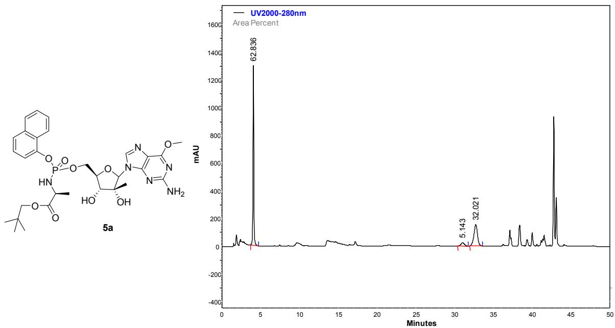
**Fig.5.** HPLC trace of **5a**, crude reaction mixture (Entry 3 Table 1).
