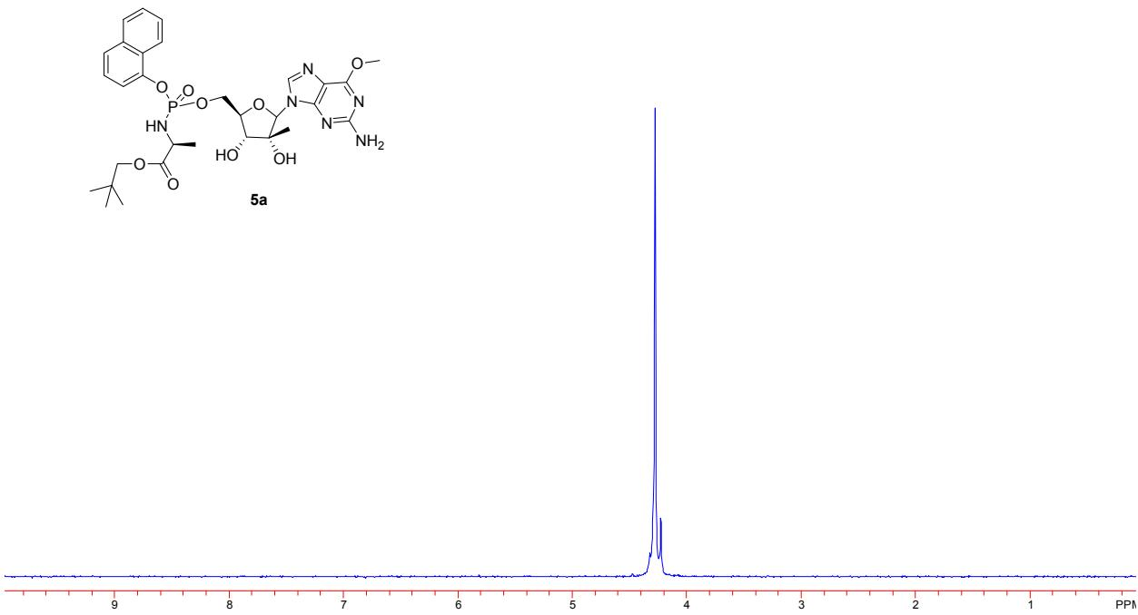
**Fig.16.** <sup>31</sup>PNMR ( $\text{CD}_3\text{OD}$ , 202 MHz) of 2-amino-6-methoxy-9-(2'-C-methyl-  $\beta$ -D -ribofuranosyl) purine 5'-O-[ $\alpha$ -naphthyl-(2,2-dimethylpropoxy-L-alaniny)] phosphate **5a** ( $R_p : S_p$  dr 1.2:8.8).
