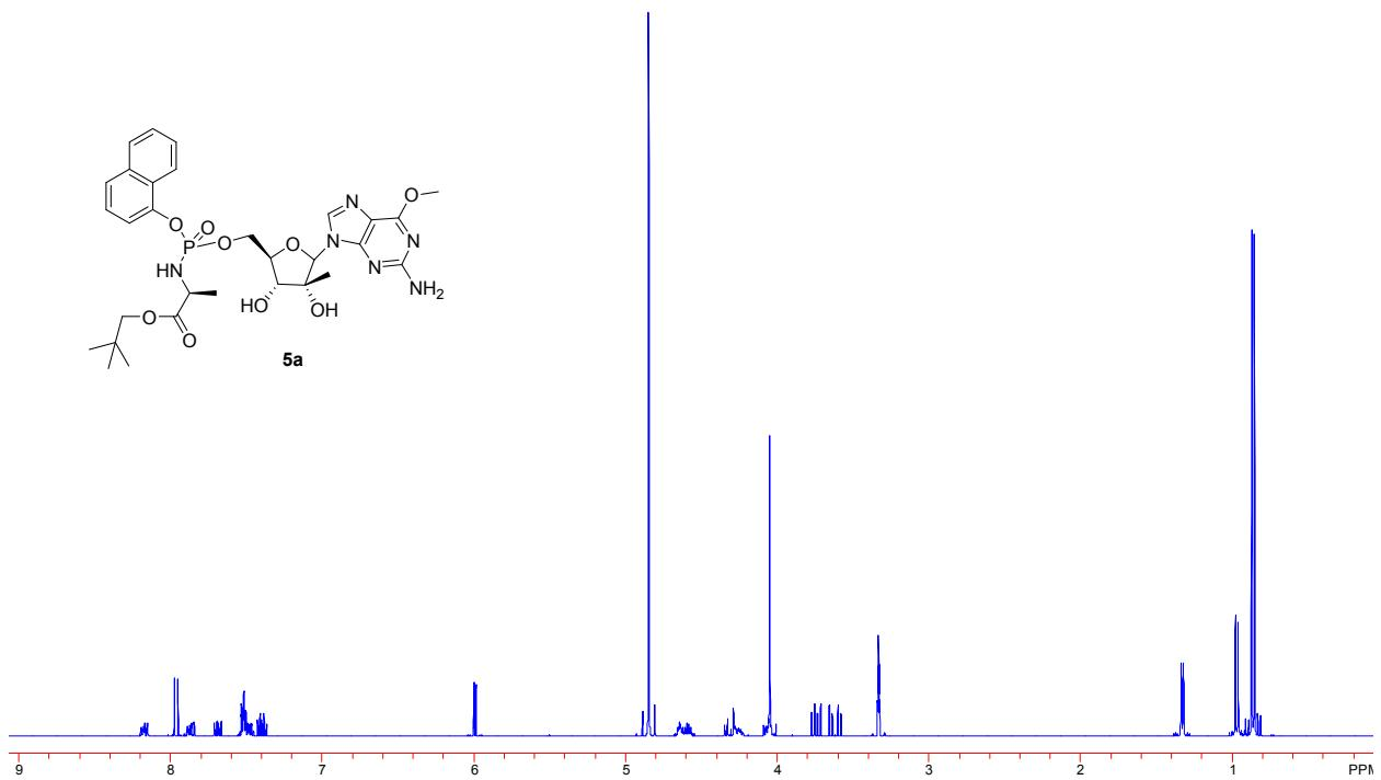
**Fig.3.** <sup>1</sup>HNMR ( $\text{CD}_3\text{OD}$ , 500 MHz) of 2-amino-6-methoxy-9-(2'-C-methyl- $\beta$ -D-ribofuranosyl) purine 5'-O-[ $\alpha$ -naphthyl-(2,2-dimethylpropoxy-L-alaninyl)] phosphate **5a** ( $R_p:\text{Sp dr } 1:1$ ).
