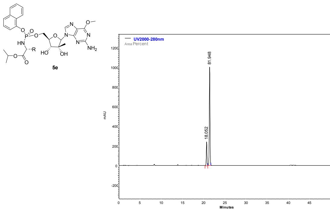
**Fig.42.** HPLC trace of 2-amino-6-methoxy-9-(2'-C-methyl- $\beta$ -D-ribofuranosyl)purine 5'-O-[ $\alpha$ -naphthyl-(isopropoxy-L-alaninyl)]phosphate **5e** ( $R_p : Sp$  dr 1:4.5).
