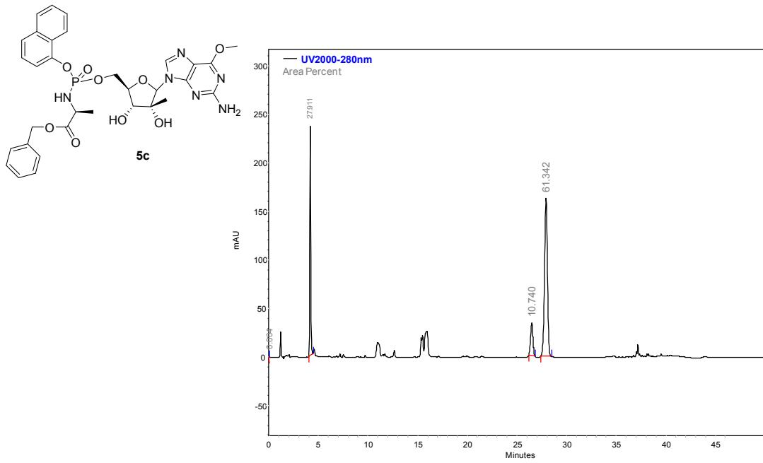
**Fig.28.** HPLC trace of **5c**, Crude reaction mixture (Entry 3, Table 2).
