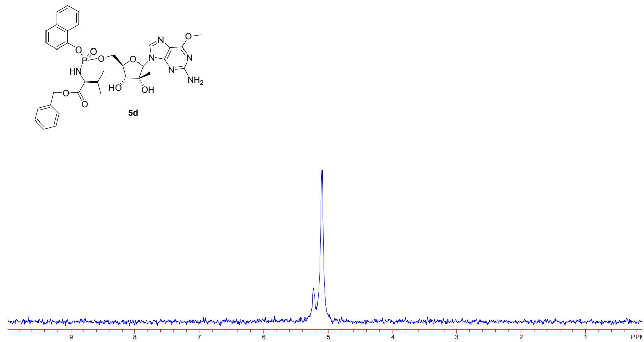
**Fig.34.**  $^{31}\text{P}$ NMR ( $\text{CD}_3\text{OD}$ , 202 MHz) of 2-amino-6-methoxy-9-(2'-C-methyl-  $\beta$ -D -ribofuranosyl)purine 5'-O-[ $\alpha$ -naphthyl-(benzyloxy-L-alaninyl)]phosphate **5d** ( $R_p : Sp$  dr 1:5).
