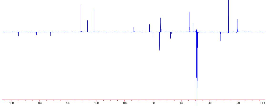
**Fig.26.**  $^{13}\text{C}$  Pendant NMR ( $\text{CD}_3\text{OD}$ , 125 MHz) of 2-amino-6-methoxy-9-(2'-C-methyl- $\beta$ -D-ribofuranosyl)purine 5'-O-[phenyl-(2,2-dimethylpropoxy-*L*-alaninyl)]phosphate **5b** ( $R_p : Sp$  dr 1:4.3).
