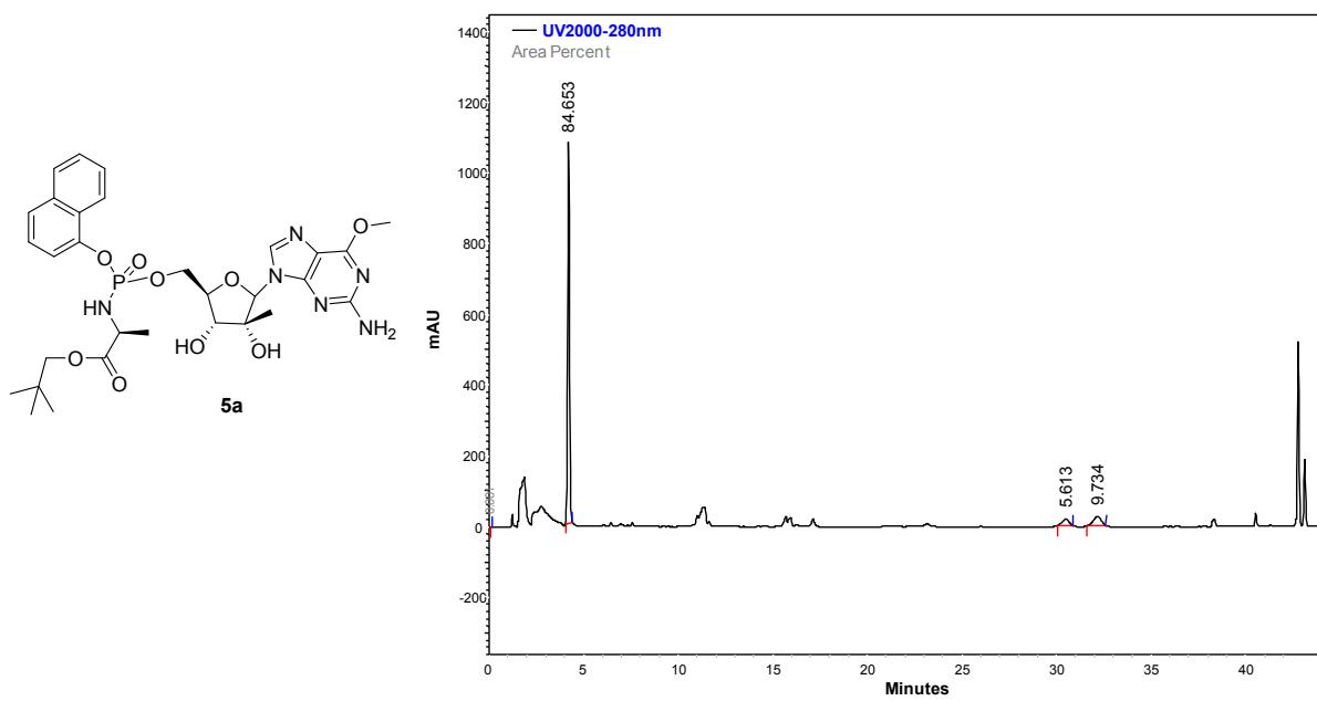
**Fig.9.** HPLC trace of **5a**, crude reaction mixture (Entry 11 Table 1).
