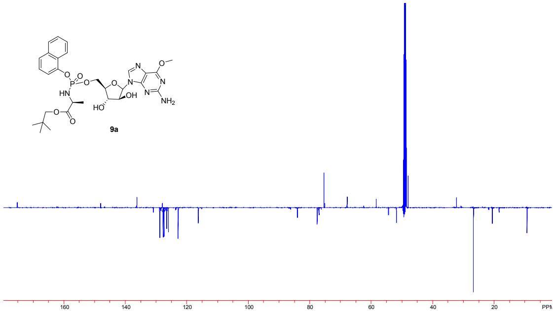
**Fig.53.**  $^{13}\text{C}$  Pendant NMR ( $\text{CD}_3\text{OD}$ , 125 MHz) of 2-amino-6-methoxy-9-( $\beta$ -D -arabinofuranosyl) purine 5'-O-[ $\alpha$ -napthyl-(2,2-dimethylpropoxy-L-alaninyl)] phosphate **9a**.
