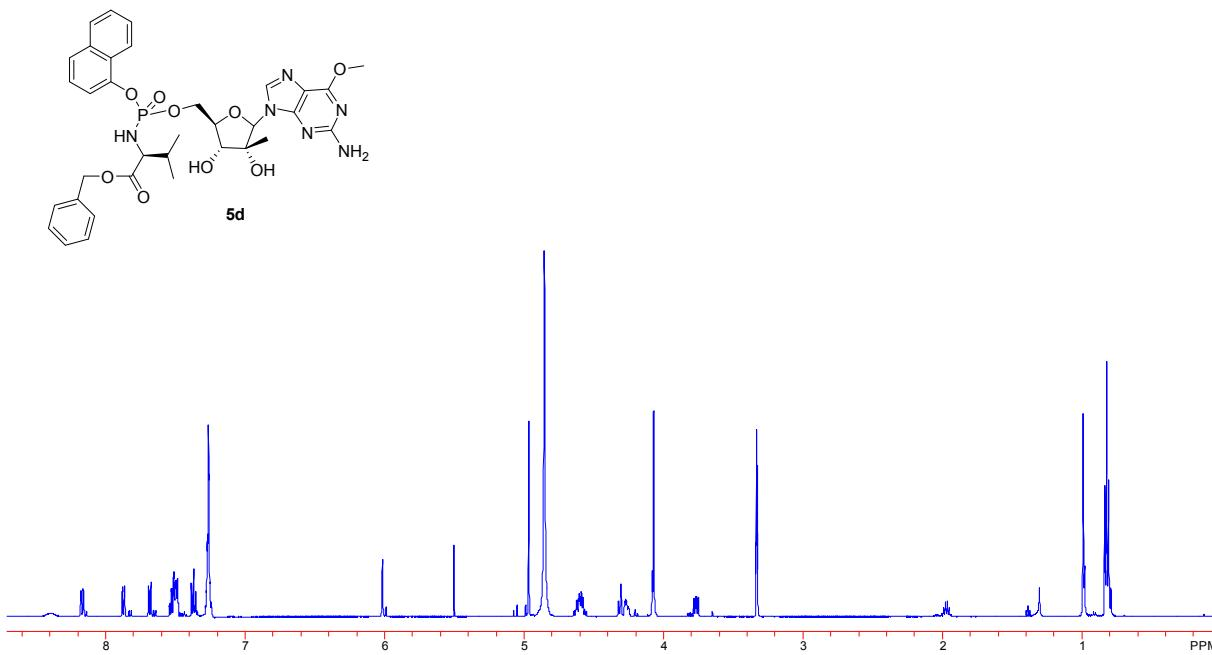
**Fig.35.** <sup>1</sup>HNMR (CD<sub>3</sub>OD, 500 MHz) of 2-amino-6-methoxy-9-(2'-C-methyl-β - D -ribofuranosyl)purine 5'-O-[α-naphthalyl-(benzyloxy-L-alaninyl)]phosphate **5d** (Rp : Sp dr 1:5).
