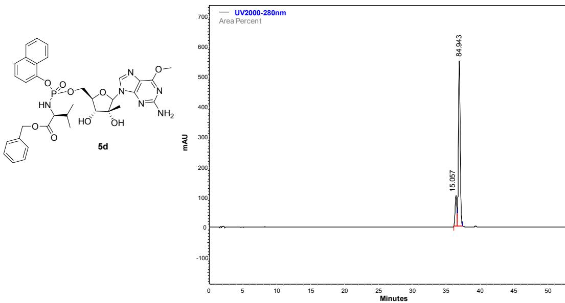
**Fig.37.** HPLC trace of 2-amino-6-methoxy-9-(2'-C-methyl- $\beta$ -D-ribofuranosyl)purine 5'-O-[ $\alpha$ -naphthyl-(benzyloxy-L-alaninyl)]phosphate **5d** ( $R_p$  : Sp dr 1:5).
