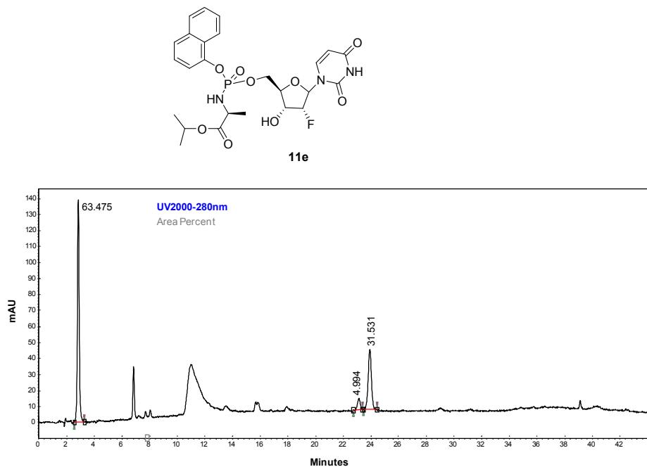
**Fig.60.** HPLC trace of **11e**, crude reaction mixture (Entry 8, table 3).
