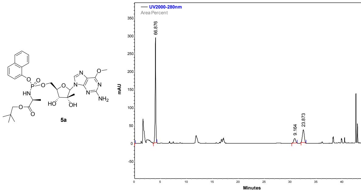
**Fig.12.** HPLC trace of **5a**, crude reaction mixture (Entry 15 Table 1).
