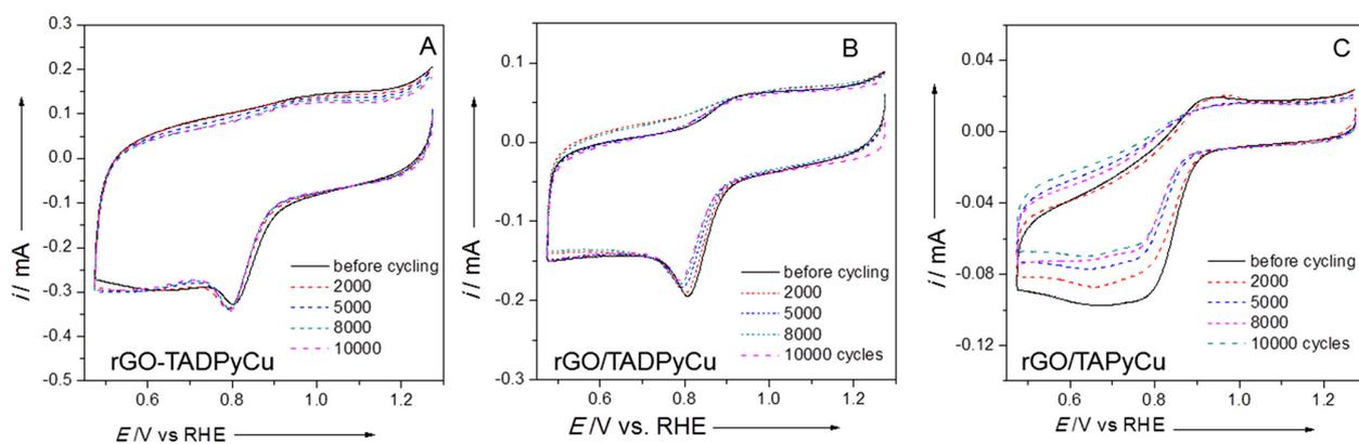
**Figure S10** Cyclic voltammograms of rGO-TADPyCu (A), rGO/TADPyCu (B), and rGO/TAPyCu (C) in  $O_2$ -saturated 0.1 M KOH solution. The first, 2000<sup>th</sup>, 5000<sup>th</sup>, 8000<sup>th</sup>, and 10000<sup>th</sup> curves were shown, respectively. Scan rate,  $50 \text{ mVs}^{-1}$ .
