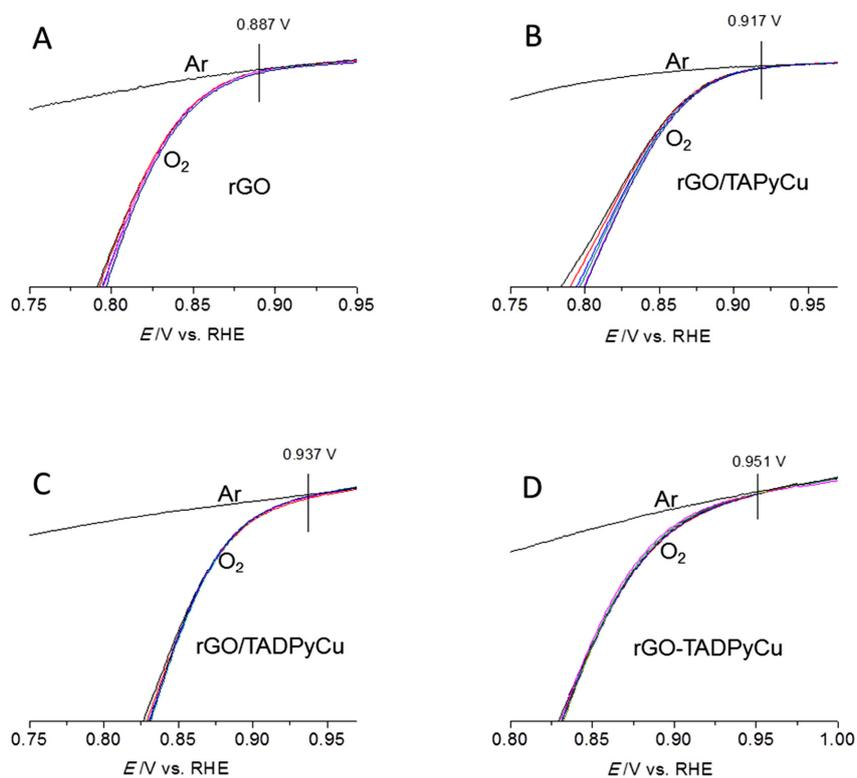
**Figure S8** The onset potential for ORR (A) rGO, (B) rGO/TAPyCu, (C) rGO/TADPyCu, (D) rGO-TADPyCu. The  $E_{\text{onset}}$  is defined here as the potential where the current deviates from that of the background under Ar atmosphere.
