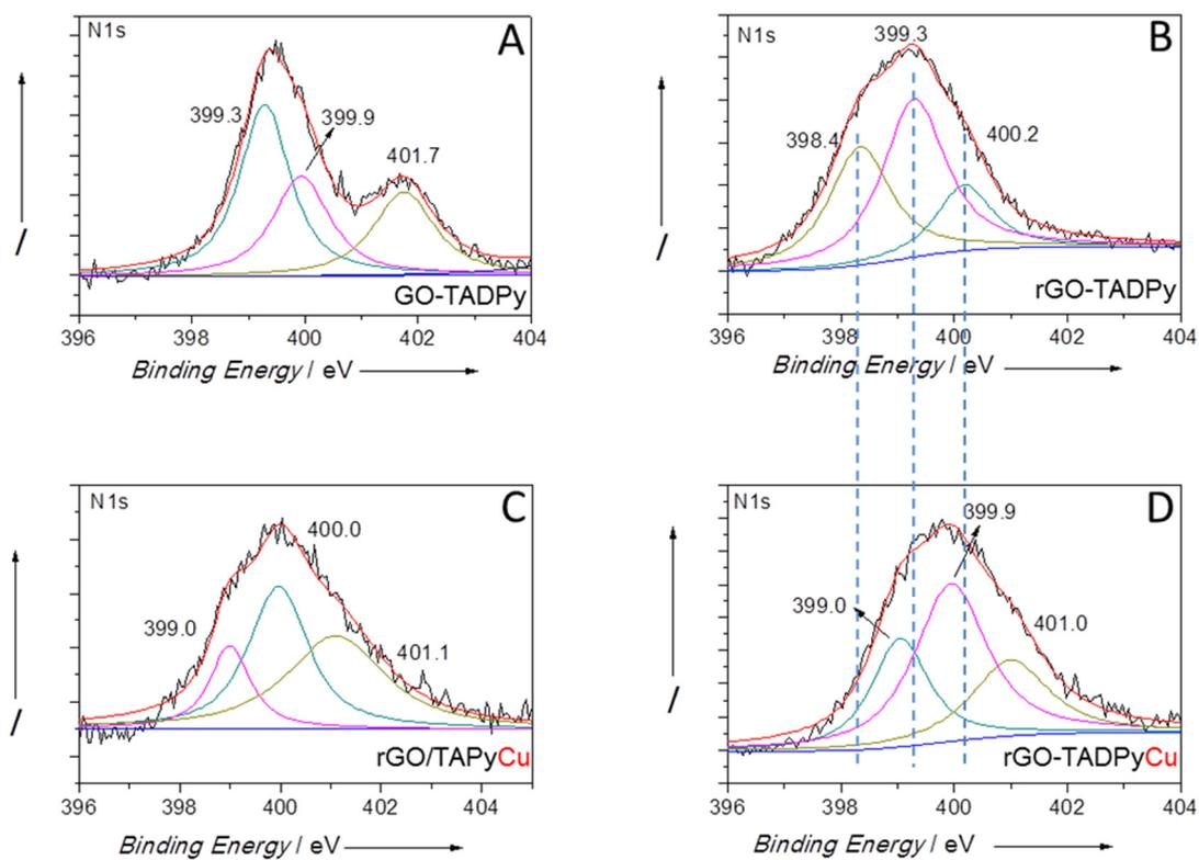
**Figure S3** High resolution XP N1s spectra of GO-TADPy (A), rGO-TADPy (B), rGO/TAPyCu (C), and rGO-TADPyCu (D).
