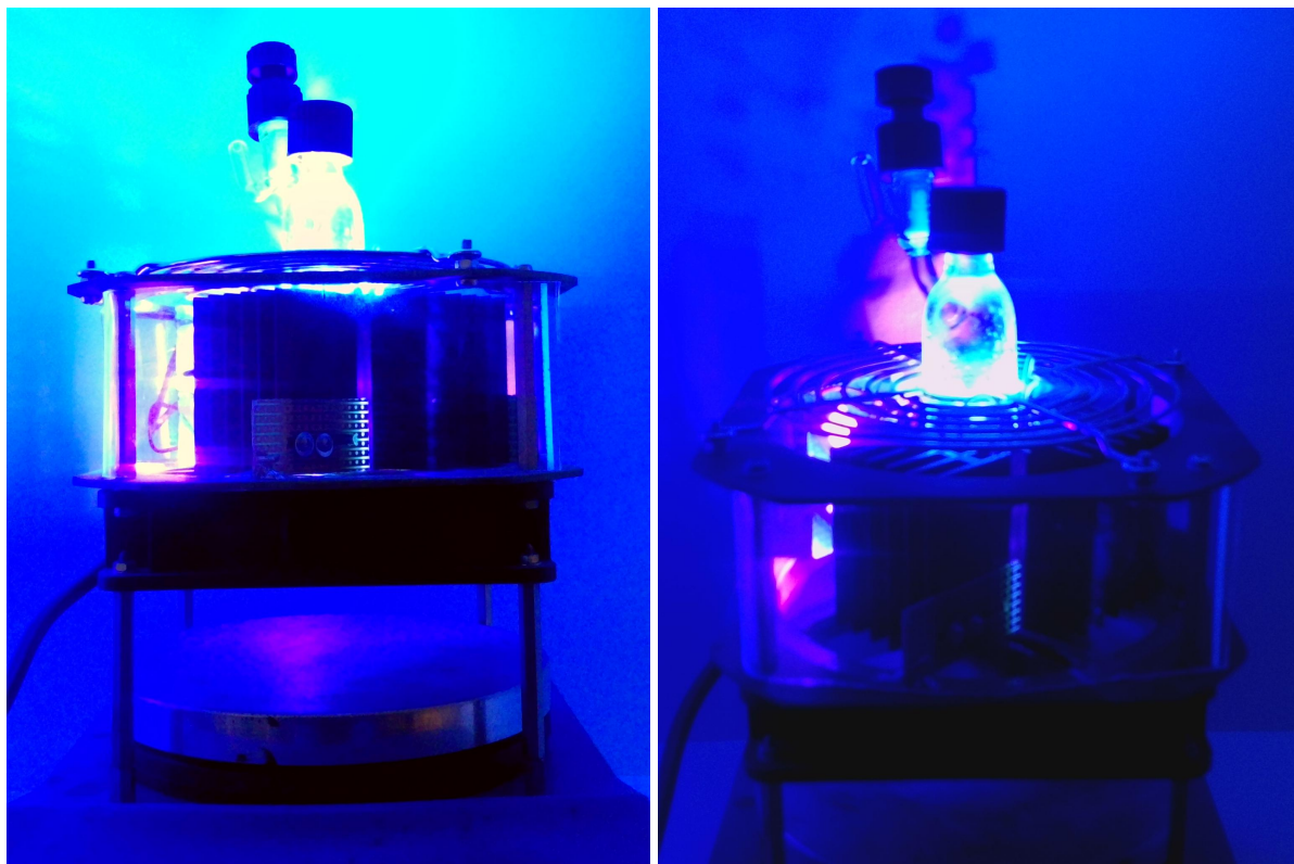
Figure S59: Front view of the switched on apparatus on magnetic stirrer with reaction mixture in Schlenk tube (cyan fluorescence of 2 occurs).
