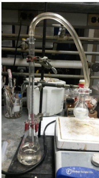
Figure S3: Gas volume change measurement setup. (graduated pipet immersed in mineral oil)
