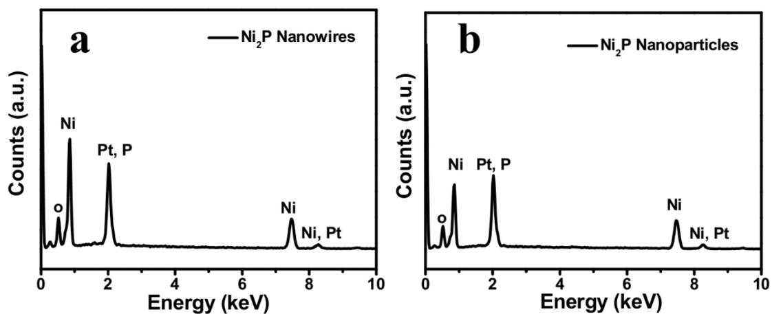
**Figure S2.** (a) EDX spectrum of the as-prepared Ni<sub>2</sub>P nanowires and the atom ratio of Ni and P is 33.74:17.77. (b) EDX spectrum of the as-prepared Ni<sub>2</sub>P nanoparticles and the atom ratio of Ni and P is 42.37:20.55.
