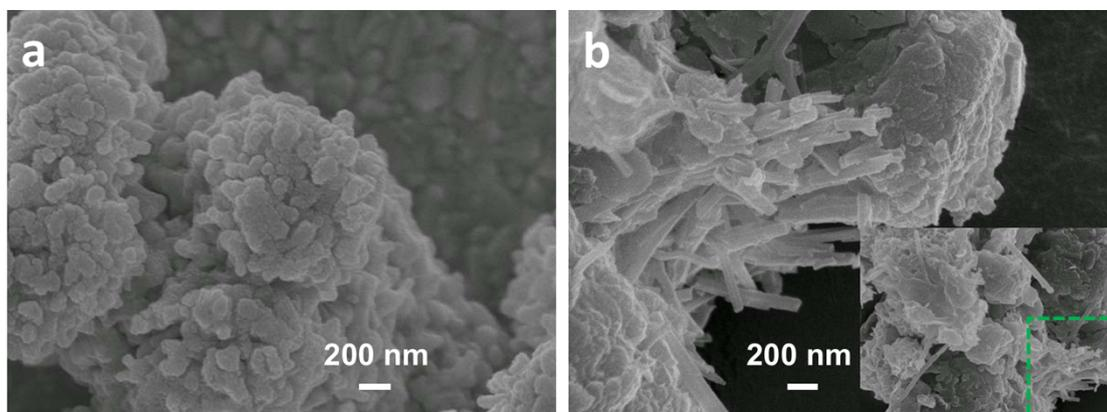
**Figure S4.** SEM images of NiO<sub>x</sub> derived from Ni<sub>2</sub>P nanoparticles and nanowires after bulk electrolysis for 5 h under an applied potential of 1.60 V (vs.RHE).
