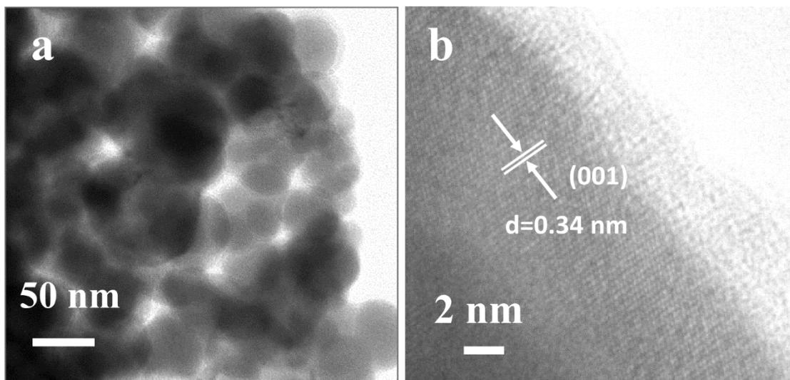
**Figure S1.** (a) TEM image of Ni<sub>2</sub>P nanoparticles; (b) HR-TEM image of Ni<sub>2</sub>P nanoparticles.
