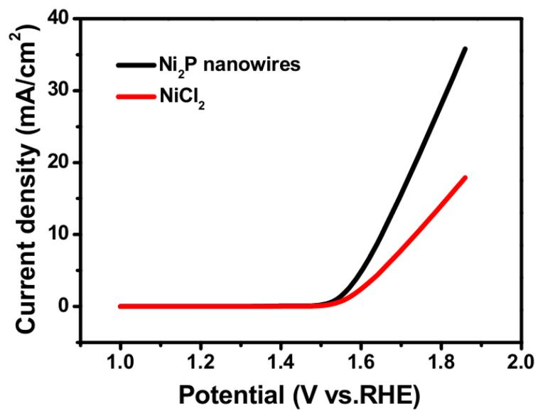
**Figure S3.** Linear sweep voltammetry (LSV) scans of water oxidation catalyst derived from different precursors in 1.0 M KOH. Black plot: Ni<sub>2</sub>P nanowires, red plot: NiCl<sub>2</sub>.
