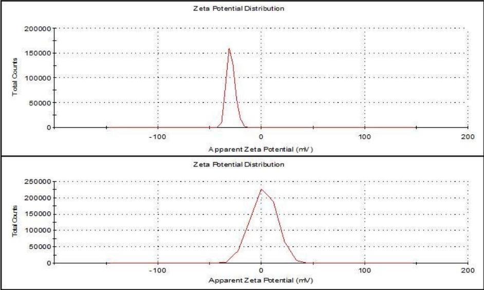
Figure S7: zeta potential measurements in PBS before (upper panel) and after (lower panel) the coating of AuSi with silane-PEG-NH<sub>2</sub>.
