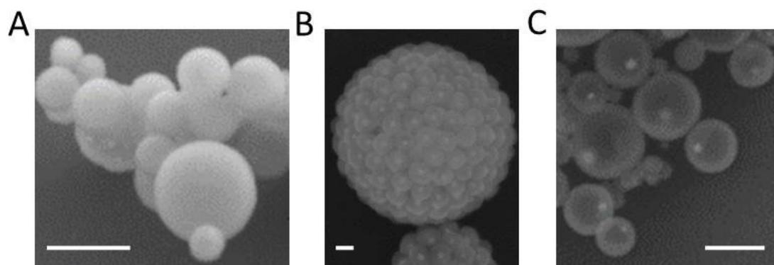
Figure S4: SEM images of AuSi (A) and calcinated AuSi (B, C). Scalebars 100 nm.
