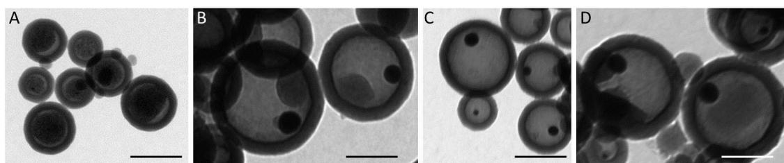
Figure S5: TEM images of AuSi (A) and calcinated AuSi (B, C,D). Scalebars 100 nm (A, C), and 50 nm (B, D).
