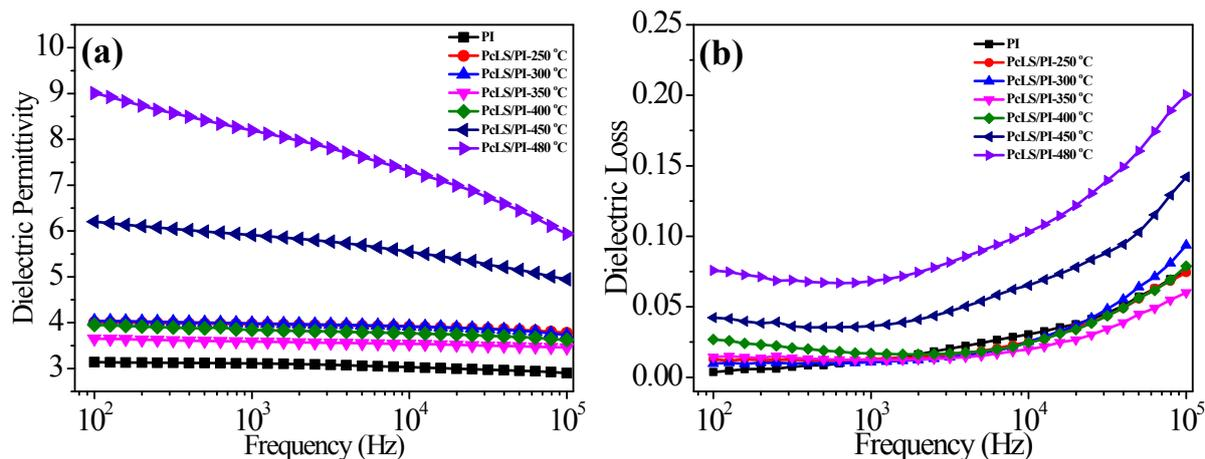
**Figure S7** Frequency dependent dielectric permittivity (a) and dielectric loss (b) of the PcLS/PI composite film derived from the PAN/PI film containing 25 wt% PAN under different high temperature treatment.
