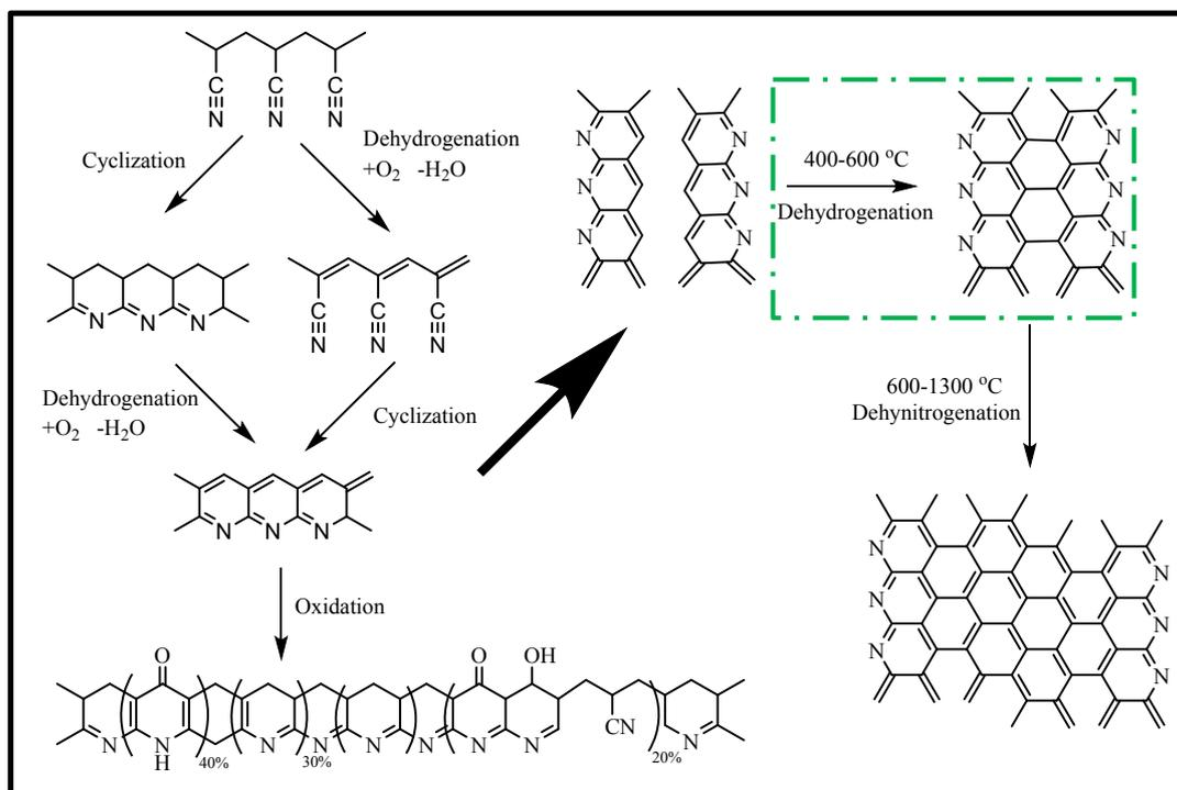
**Figure S2** The preparation of carbon fibers from PAN, which generally includes three procedures: stabilization, carbonization, and graphitization. The high temperature treated at 400-600 °C will yield the polycondensed ladder structures (PcLS).
