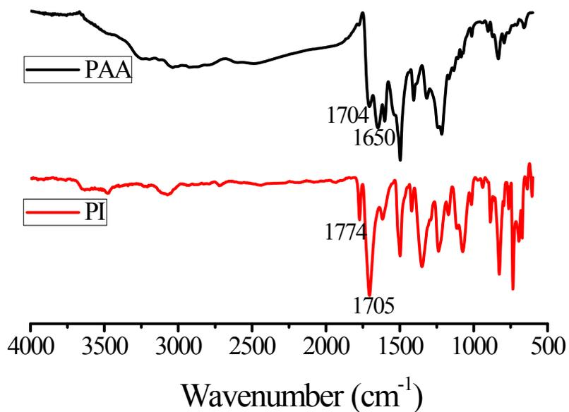
**Figure S5** FT-IR spectrum of neat PAA and PI film obtained under 480 °C treatment.
