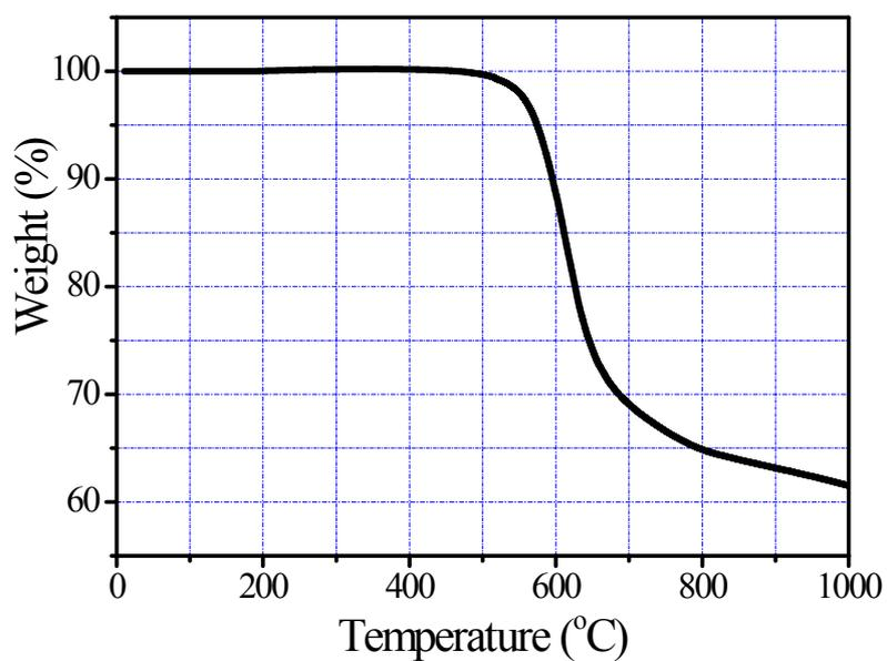
**Figure S6** TGA curves of neat PI film obtained under 480 °C treatment.
