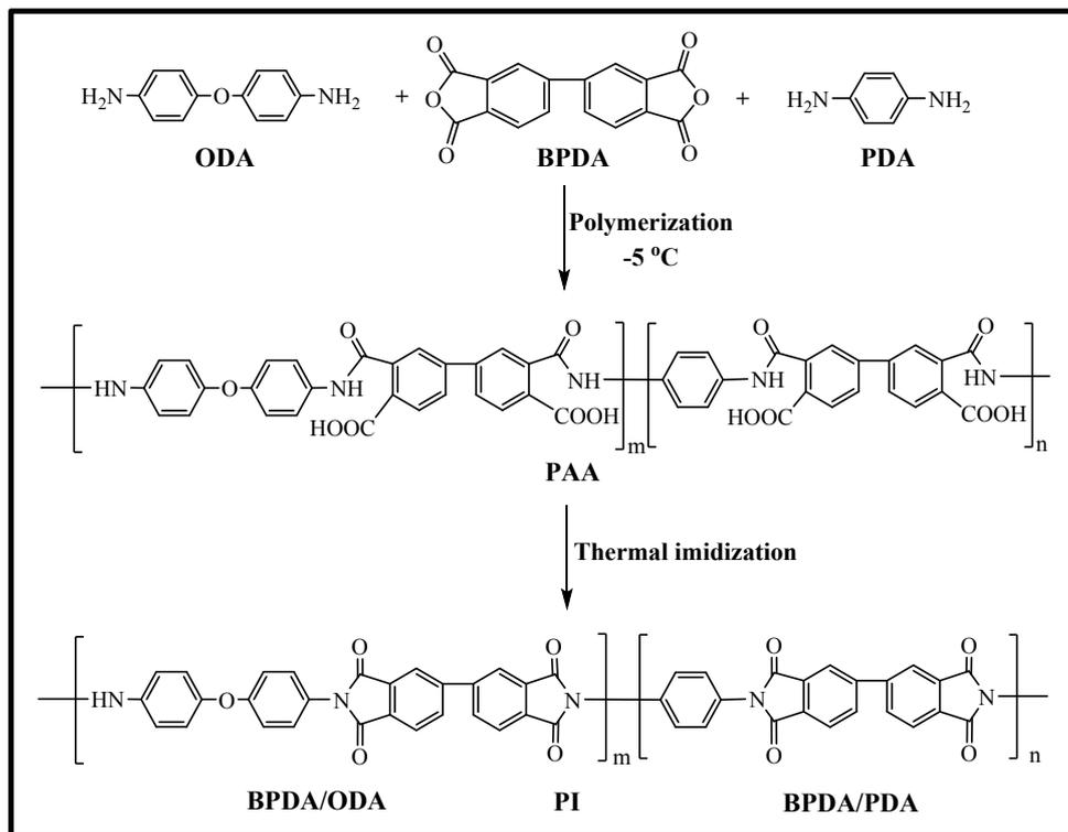
**Figure S3** Schematic diagram of the synthesis of polyimide (BPDA/PDA/ODA) by polycondensation between BPDA and diamines, ODA and PDA.
