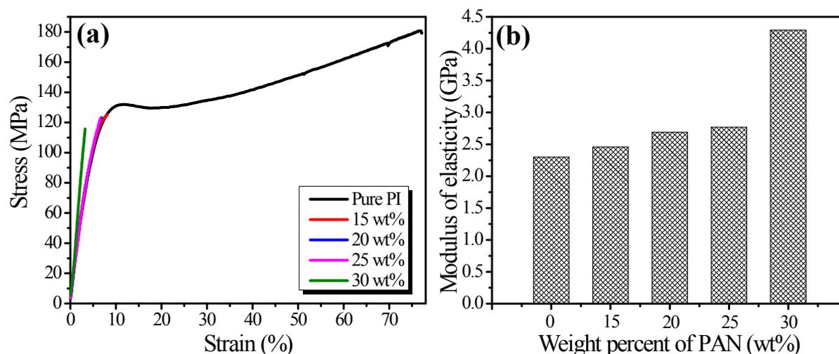
**Figure S8** (a) Typical stress–strain curves of mechanical properties of the PcLS/PI composite films with different PAN content in the PAN/PAA precursor. (b) Histogram comparison of elastic modulus of the PcLS/PI composite films.
