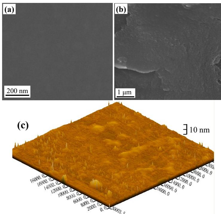
**Figure S4** SEM images of the surface (a) and cross section (b) of the PcLS/PI composite film. (c) AFM image of the surface of the PcLS/PI composite film.
