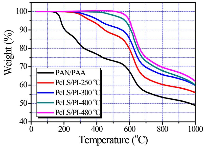
**Figure S9** TGA curves of the fabricated PAN/PI film and PcLS/PI composite films obtained from different temperature treatment.
