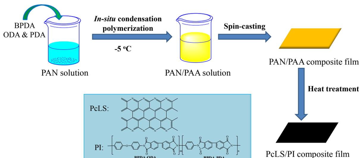
**Figure S1** Schematic procedure for the preparation of PcLS/PI composite film.
