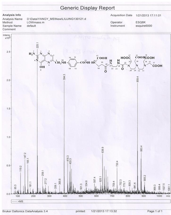
Figure S12. ESI-MS of FA-EDA-DTPA. (m/z): [M + H]<sup>+</sup> 859.4.
