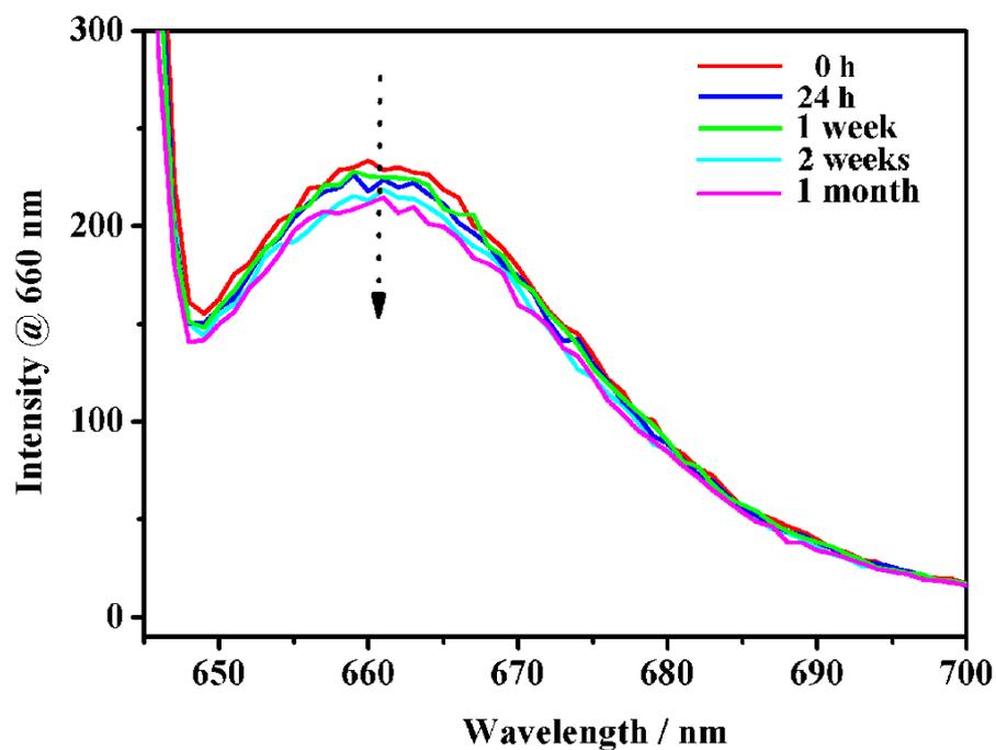
Figure S4. Fluorescence spectra of **1** at different time periods within one month. Ex = 620 nm, Em = 660 nm, belonging to Cy5.
