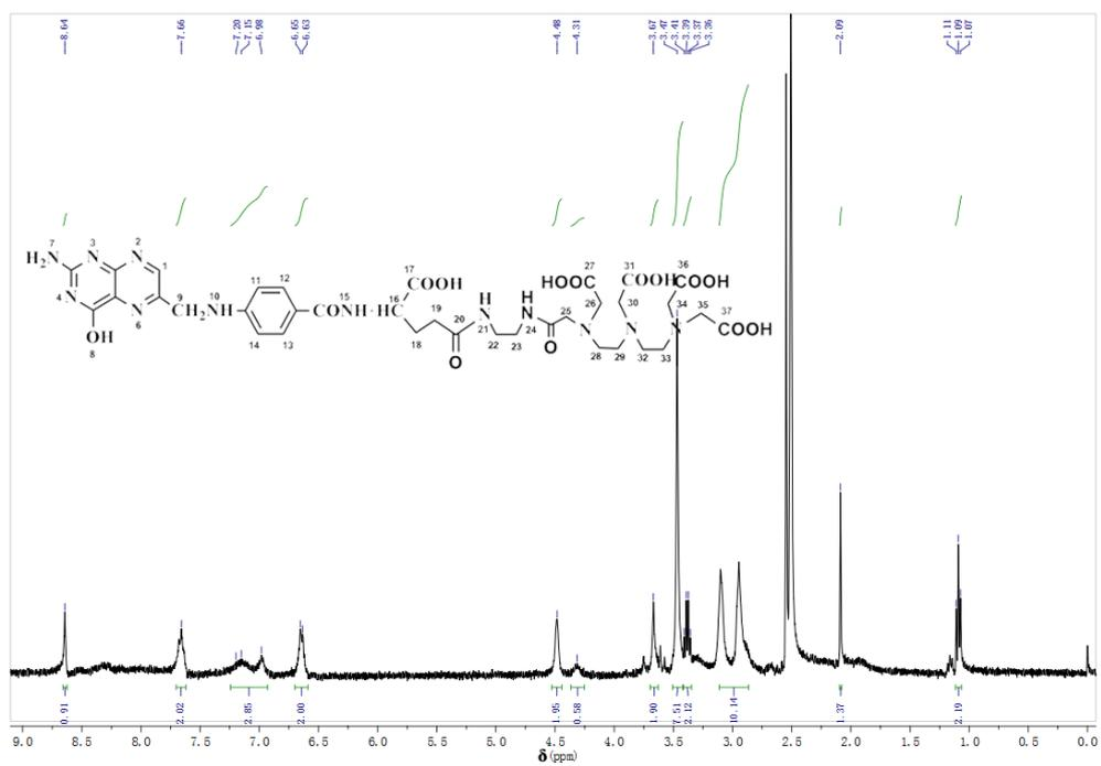
Figure S13. <sup>1</sup>H NMR Spectrum of FA-EDA-DTPA.
