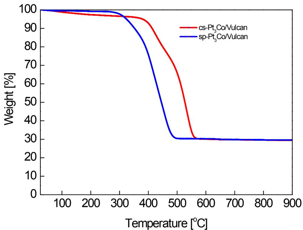
Figure S8. TGA analysis of the sp-Pt<sub>3</sub>Co/Vulcan and cs-Pt<sub>3</sub>Co/Vulcan is indicating that the Pt loading of sp- and cs-Pt<sub>3</sub>Co catalysts is 30%.
