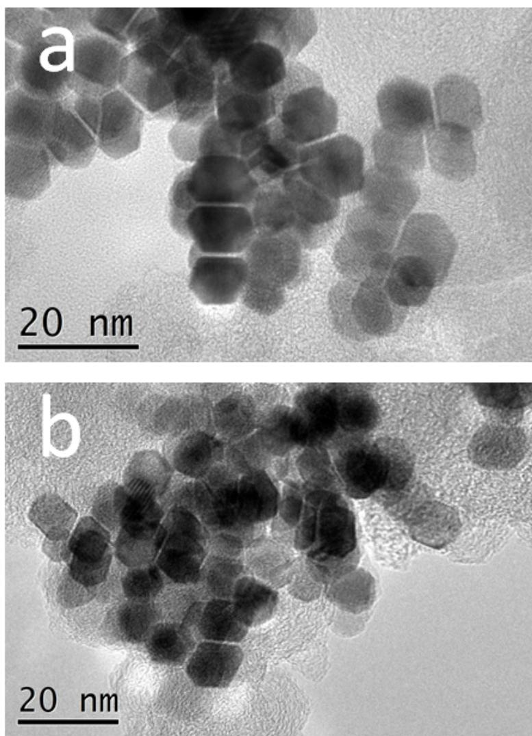
Figure S11. TEM images of  $cs\text{-Pt}_3\text{Co}$  decorated on Vulcan XC-72 support before (a) and after (b) 5000 cyclic voltammetry sweeps
