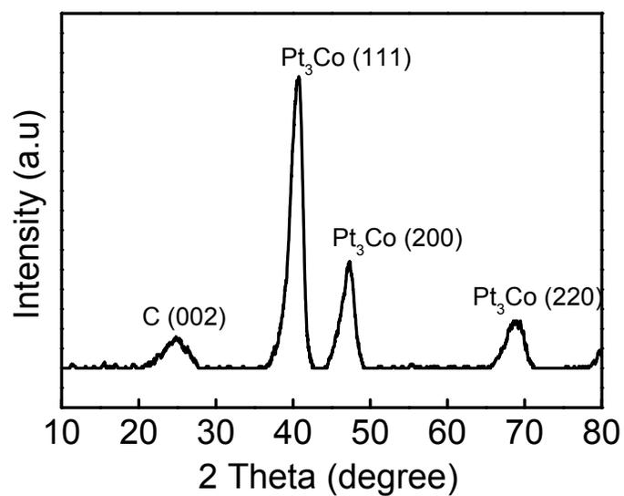
Figure S3. XRD pattern of the as-prepared cs-Pt<sub>3</sub>Co catalyst decorated on Vulcan XC-72R
