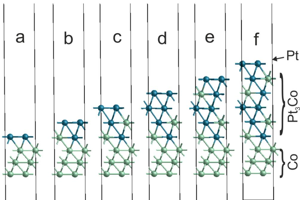
Figure S13 Pt<sub>3</sub>Co supercell with three bottom slabs as a cobalt core, a Pt<sub>3</sub>Co intermediate region (except in (a)), and a pure Pt monolayer at the top layer. (a) contains just Co and the Pt monolayer, while systems in (b-f) exhibit from 1 up to 5 Pt<sub>3</sub>Co slabs as a shell, with their respective Pt monolayer at the top.
