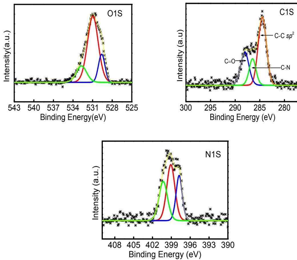
Figure S2. High-resolution XPS spectrum of C, O, and N in the cs-Pt<sub>3</sub>Co nanocrystals
