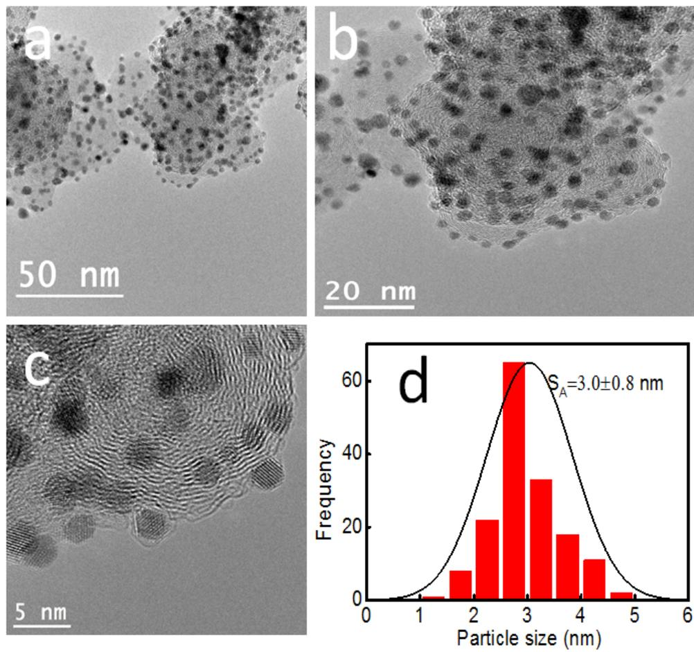
Figure S6. TEM images (a, b, and c) of sp-Pt<sub>3</sub>Co/Vulcan in different magnification and their particle size distribution (d)
