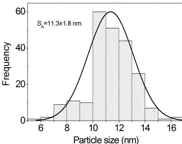
Figure S1. Size distribution of the cs-Pt<sub>3</sub>Co nanoparticles.
