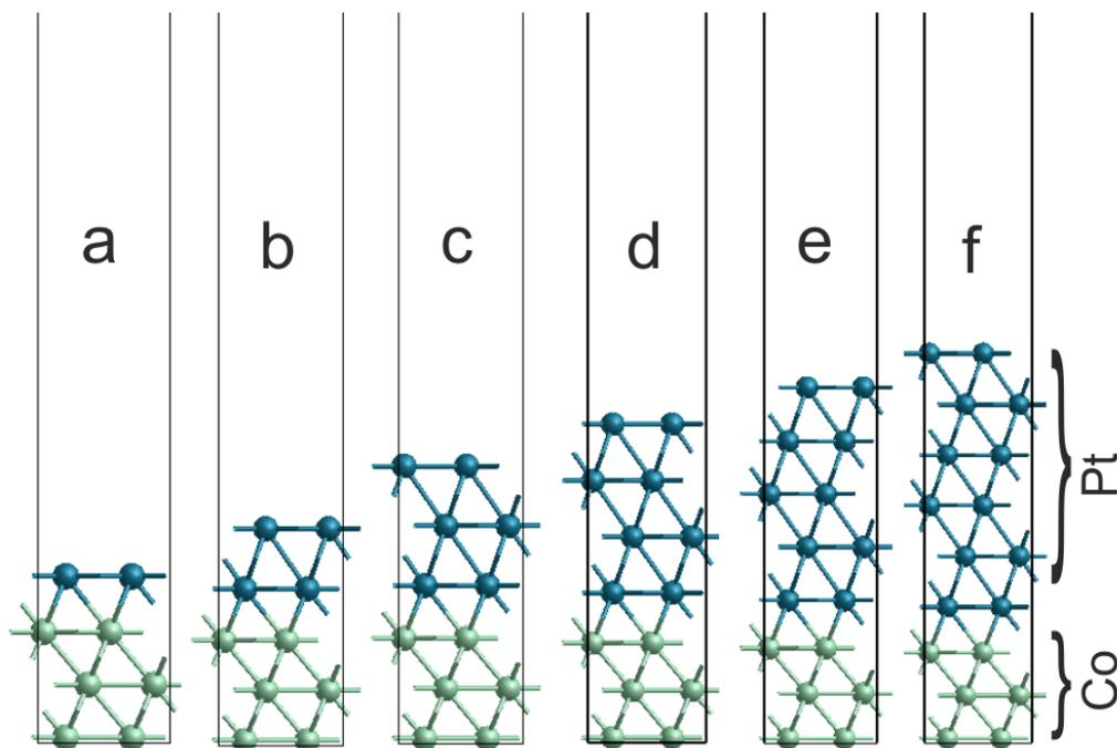
Figure S12 Pt-Co supercell with three bottom slabs as a cobalt core. In (a-f) systems with 1 up to 6 Pt slabs as a shell are shown.
