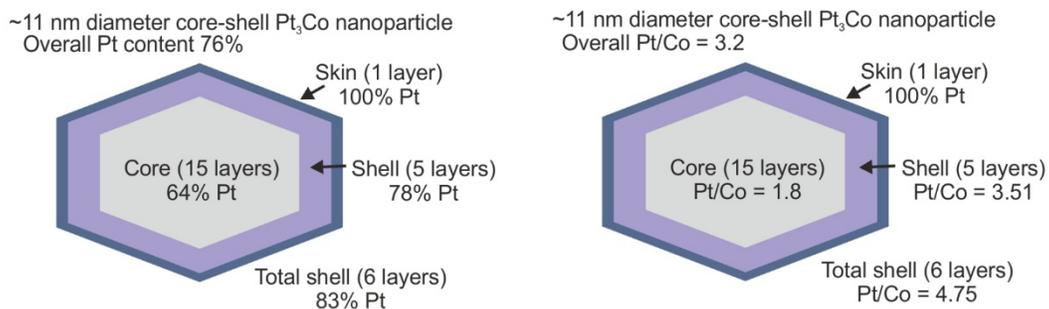
Figure S5. Description of Pt composition along the cs-Pt<sub>3</sub>Co nanoparticle according to EDS, XPS, and the average particle size. Pt content is indicated by At% in the left side. Right side the Pt/Co ratio is indicated.
