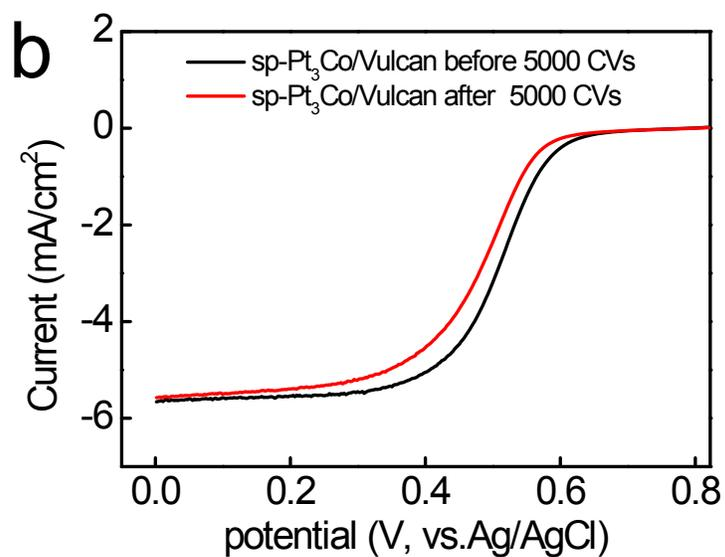
Figure S10 the polarization curves of Pt/Vulcan (a) and sp-Pt<sub>3</sub>Co/Vulcan before (black) and after 5000 CVs in the sweep range 0.32-0.72 V in O<sub>2</sub>-saturated 0.1 M HClO<sub>4</sub> solution. Rotating speed: 1600 r.p.m. scan rate: 0.05 V/s.
