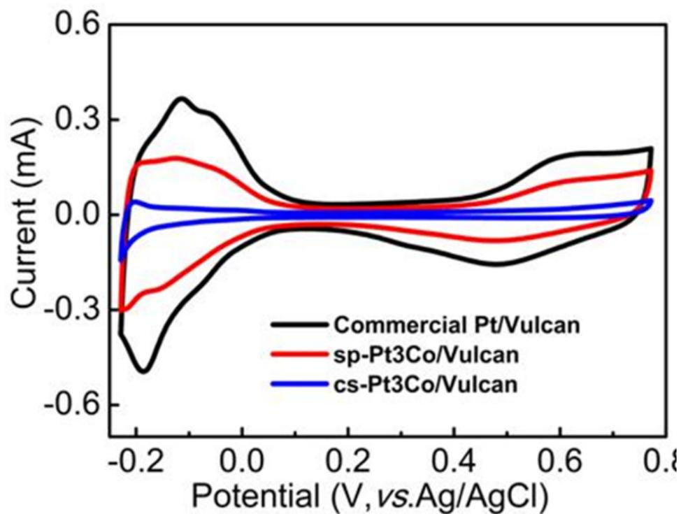
Figure S7. CVs of the different catalyst electrodes in argon-saturated 0.1 M HClO<sub>4</sub> solution at a scan rate of 0.05 V/s at room temperature.
