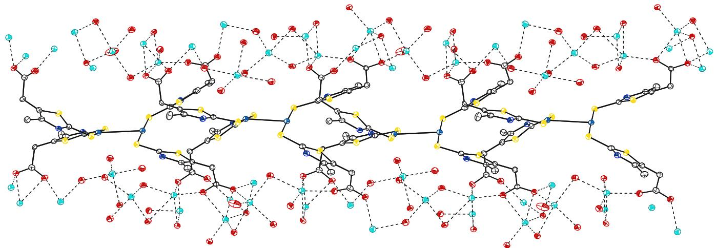
FIG. S3. A drawing of a portion of the structure of  $\text{Na}_3[\text{Au}(\text{mmta})_2]\cdot 6\text{H}_2\text{O}$  that shows the  $\pi - \pi$  stacking of the dimers along the  $b$  axis. Color code: Au - navy blue, S - yellow, O - red, N - blue, Na - cyan.
