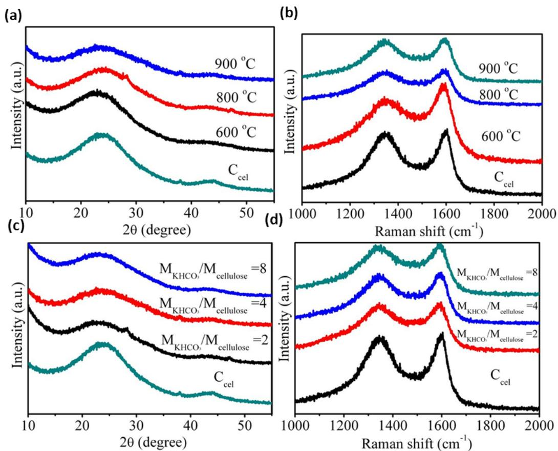
**Fig. S6** (a) XRD results and (b) Raman spectras using 514 nm excitation of  $C_{\text{cel-LE}}$  with different temperature and  $C_{\text{cel}}$ ; (c) XRD results and (d) Raman spectras using 514 nm excitation of simples calcined at  $900^\circ\text{C}$  with different mass ratio of  $\text{KHCO}_3$  to cellulose.
