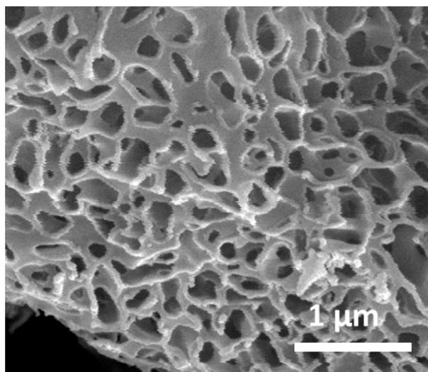
**Fig. S11** SEM image of product synthesized by pyrolyzed the mixture of  $\text{NaHCO}_3$  and cellulose as the same procedure as  $\text{C}_{\text{cel-LE}}$ .
