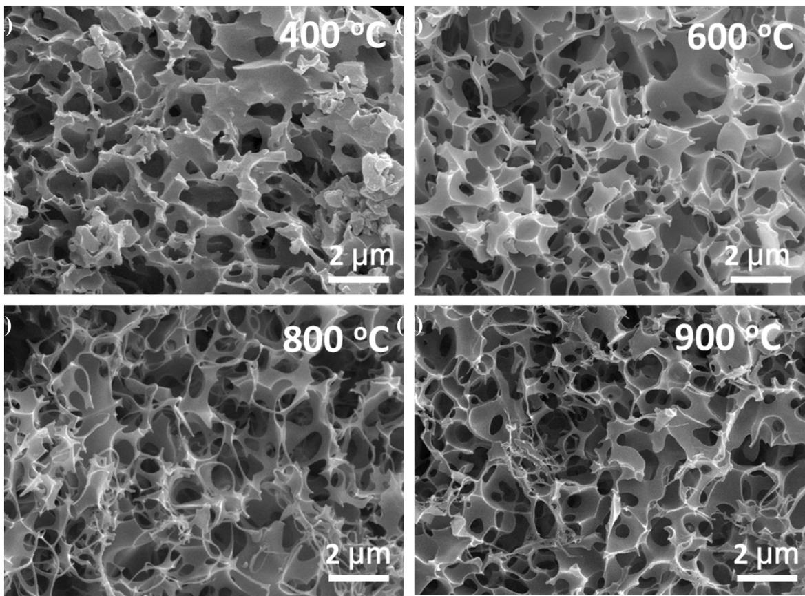
**Fig. S4** SEM images of  $C_{\text{cel-LE}}$  of different temperature (a) 400 °C, (b) 600 °C, (c) 800 °C, (d) 900 °C.
