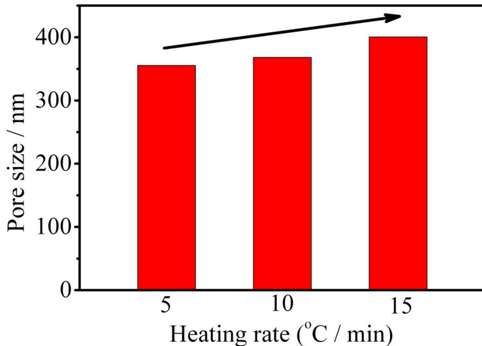
**Fig. S9** The average size of macropore of the as-prepared porous carbon material calcined at 400 °C with different heat rate.
