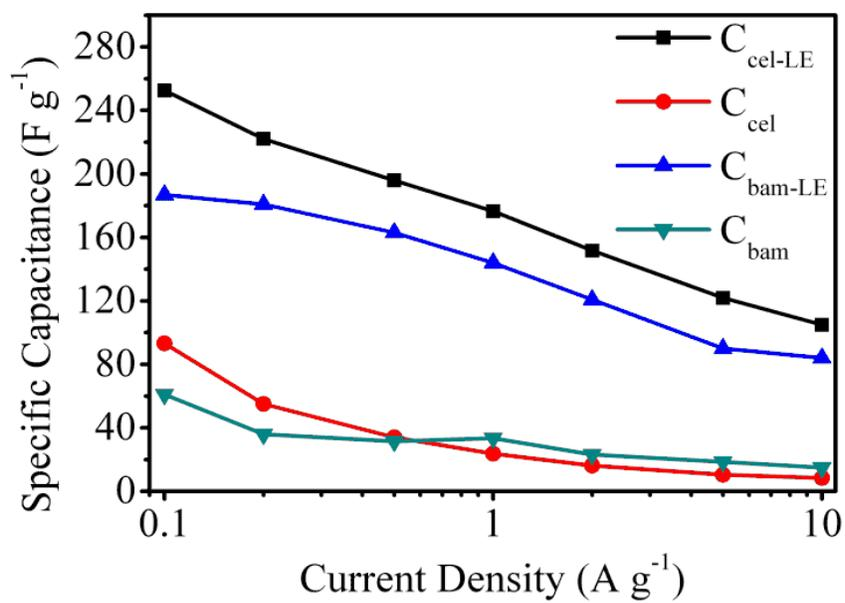
**Fig. S14** The specific capacitance of  $C_{\text{cel-LE}}$ ,  $C_{\text{cel}}$ ,  $C_{\text{bam-LE}}$  and  $C_{\text{bam}}$  as a function of current density ranging from 0.1 to 10 A g<sup>-1</sup>
