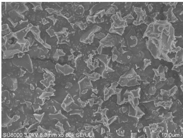
**Fig. S10** SEM image of the product derived from mixture of  $K_2CO_3$  and cellulose undergoing pyrolysis at 400 °C.
