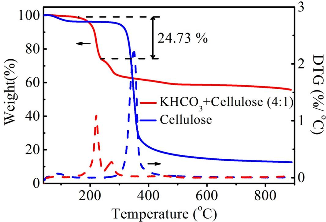
**Fig. S8** TGA results for the mixture of KHCO<sub>3</sub> and cellulose (4:1) (red) and cellulose (blue). KHCO<sub>3</sub> decompose through reaction 1. The TGA was measured at 15 °C / min under the atmosphere of N<sub>2</sub>.
