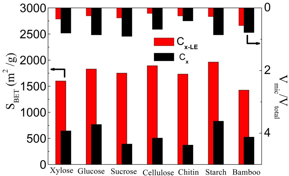
**Fig. S7** The specific surface areas and  $V_{\text{mic}}/V_{\text{total}}$  of the  $C_x$  and  $C_{x\text{-LE}}$  where x stands for the carbon precursor.
