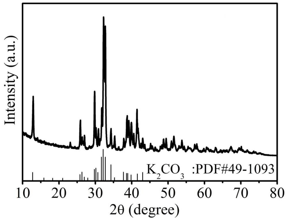
Fig. S3 the XRD spectrum of  $C_{cel-LE}$  before washing with HCl.
