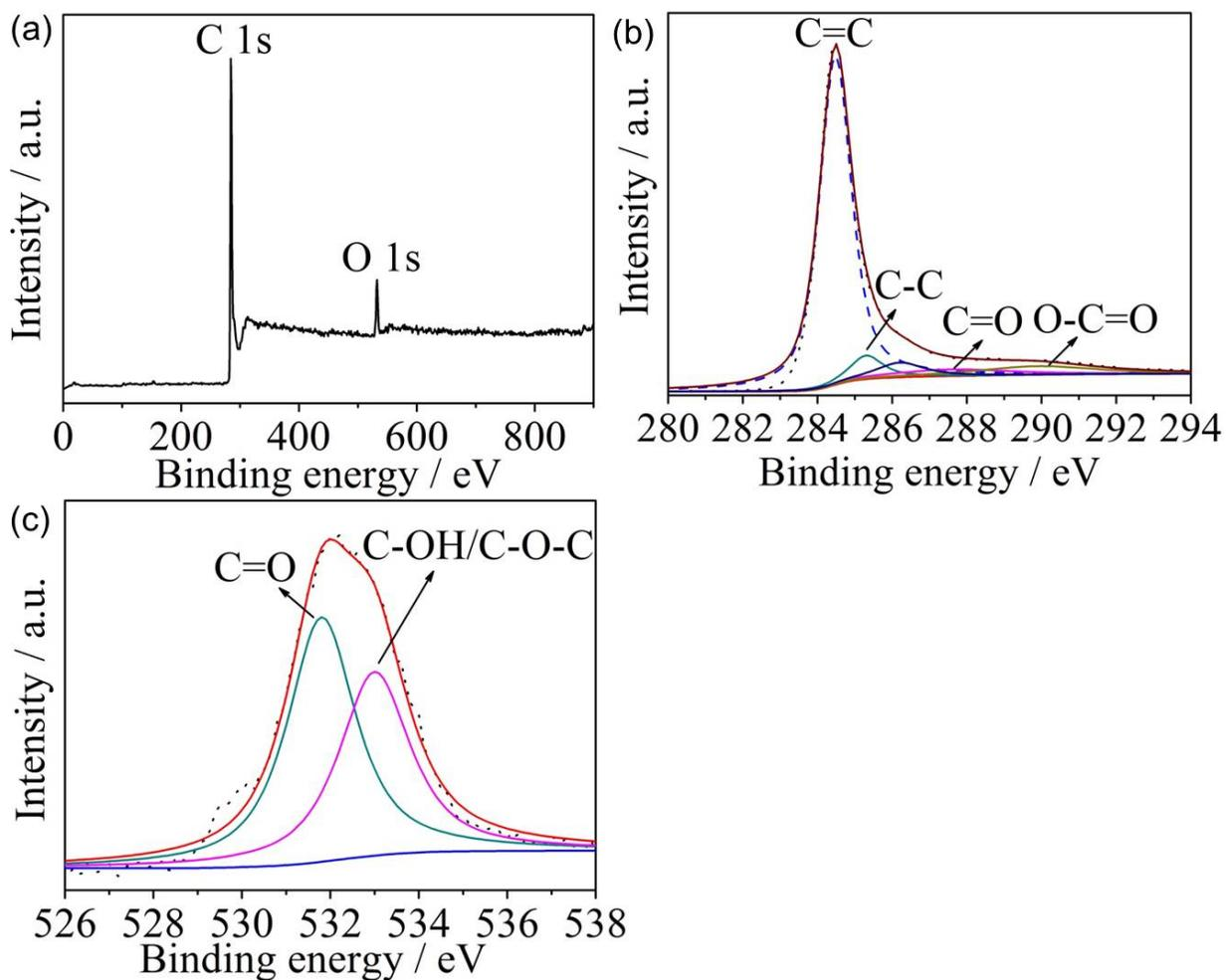
Fig. S12 (a) XPS, (b) C 1s, (c) O 1s spectra of  $C_{\text{cel-LE}}$ .
