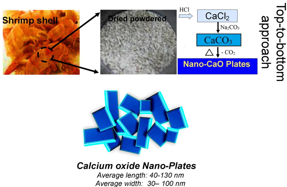
Figure S1. Schematic illustration of CaO nano-plates fabricated from Shrimp shells
