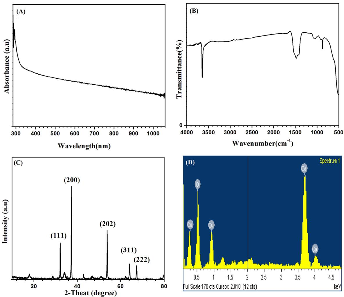
**Figure S3.** Characterization of CaO (A) UV-Visible spectrum (B) FT-IR Spectrum (C) XRD pattern (D) EDXS pattern
