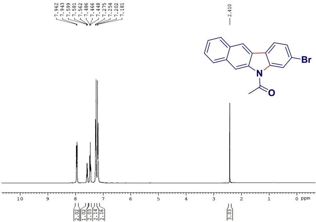
Fig. S61: <sup>1</sup>H NMR spectrum of 1-(3-bromo-benzo[b]carbazol-5-yl)-ethanone
