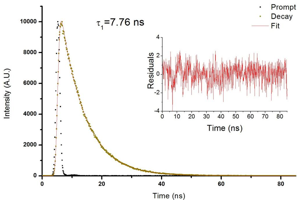
**Figure S14** Time resolved fluorescence decay of **7** in  $\text{CHCl}_3$  with the excitation source at  $\lambda_{\text{exc}}=490$  nm while monitored at  $\lambda_{\text{em}}=725$  nm. Inset: residual values after fitting.
