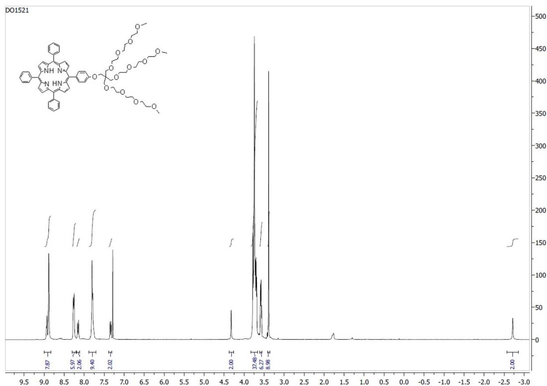
Figure S12  $^1\text{H}$  NMR spectrum of **7** (Bruker 300 MHz spectrometer,  $\text{CDCl}_3$ ).
