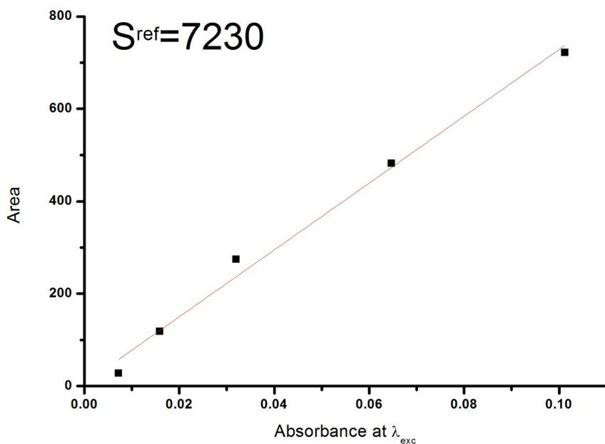
**Figure S17** Plot of the integrated area under the  $^1\text{O}_2$  emission spectrum vs the absorbance at  $\lambda_{exc}=420$  nm for various solution of phenalene in  $\text{CHCl}_3$ . The slope  $S^{ref}$  was used for the determination of  $\Phi_\Delta$  the singlet oxygen generation quantum yield according to equation (1).
