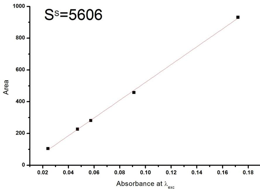
**Figure S16** Plot of the integrated area under the  $^1\text{O}_2$  emission spectrum vs the absorbance at  $\lambda_{exc}=420$  nm for various solution of compound 7 in  $\text{CHCl}_3$ . The slops  $S^S$  was used for the determination of  $\Phi_\Delta$  the singlet oxygen generation quantum yield according to equation (1).
