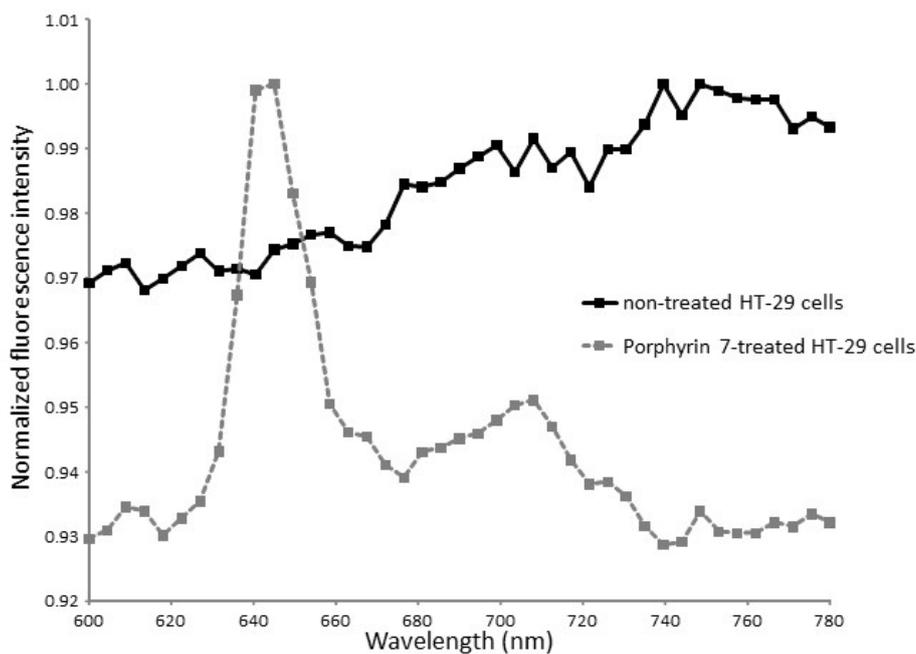
**Figure S18** Wide field fluorescence emission spectra of non-treated HT-29 cells (black) and porphyrin 7 treated HT-29 cells (grey). Spectra were acquired at 514 nm and fluorescence emission was recorded between 600 and 780 nm with a step size of 4.5 nm. The fluorescence intensity was normalized relatively to the maximum of each spectrum. The fluorescence emission spectra of treated cells showed the specific spectrum of the porphyrin 7 while the non-treated HT-29 spectrum is linear.
