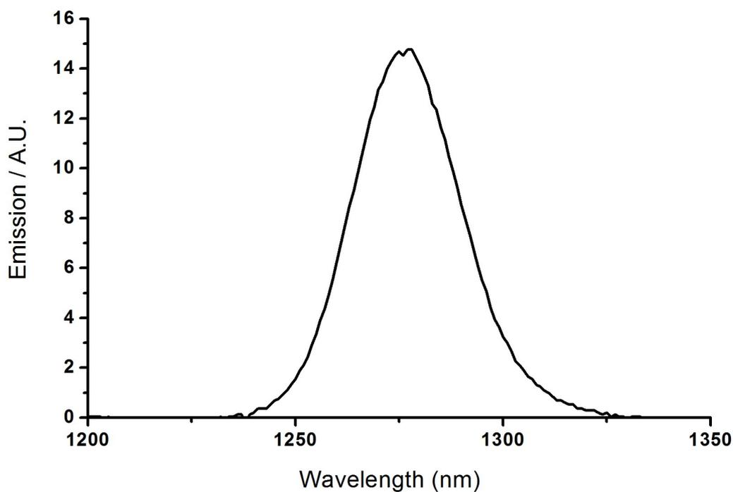
**Figure S15** Singlet oxygen phosphorescence signal measured after excitation at  $\lambda_{\text{exc}}=420$  nm.
