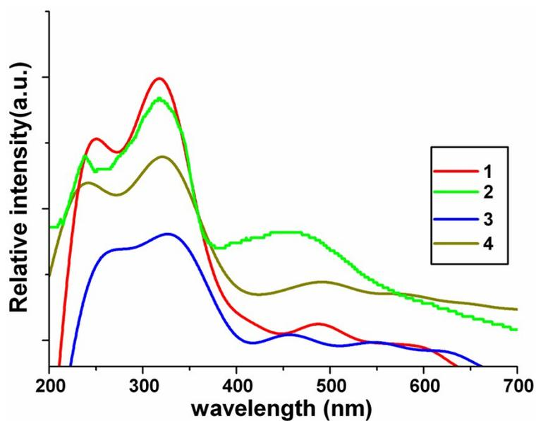
**Fig. S3** The UV-vis absorption spectra for **1–4** in the solid state at room temperature
