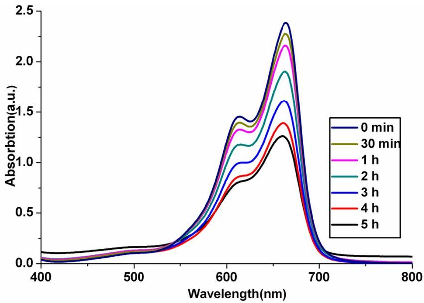
Fig. S7 UV-Vis absorption spectra of the MB solutions degraded by 4 under UV irradiation at different time intervals.
