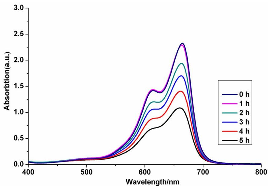
Fig. S6 UV-Vis absorption spectra of the MB solutions degraded by **3** under UV irradiation at different time intervals.
