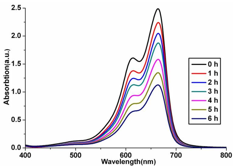
**Fig. S4** UV-Vis absorption spectra of a MB solution degraded without catalysts under UV irradiation at different time intervals
