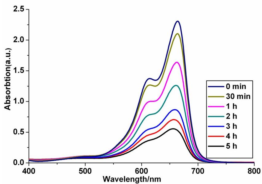
Fig. S5 UV-Vis absorption spectra of the MB solutions degraded by **1** under UV irradiation at different time intervals.
