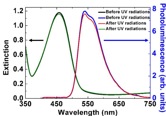
**Figure S1.** Extinction and photoluminescence spectra of F8BT before (black and blue curves) and after (green and red curves) the interference ablation.
