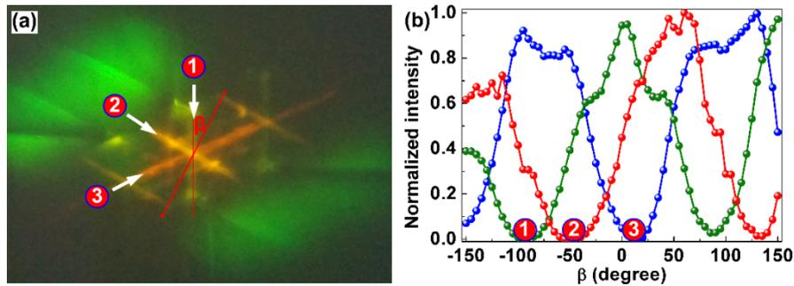
**Figure S5.** (a) Enlarged view of the laser spot.  $\Phi$ ,  $\mathcal{Q}$ , and  $\mathcal{S}$  identify the emission wavelengths of the 355 nm, 360 nm, and 365 nm cavity, respectively. The red solid line denotes the polarization
