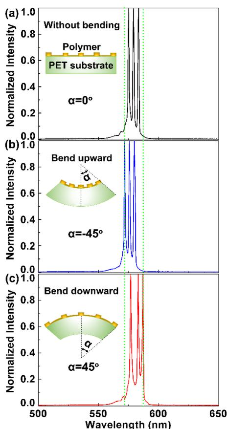
**Figure S6.** Measured spectra of the polymer laser (a) without bending, (b) with bending upward, and (c) with bending downward, where  $h_1=20$  mm,  $h_2=18$  mm and  $t=400$   $\mu\text{m}$ .
