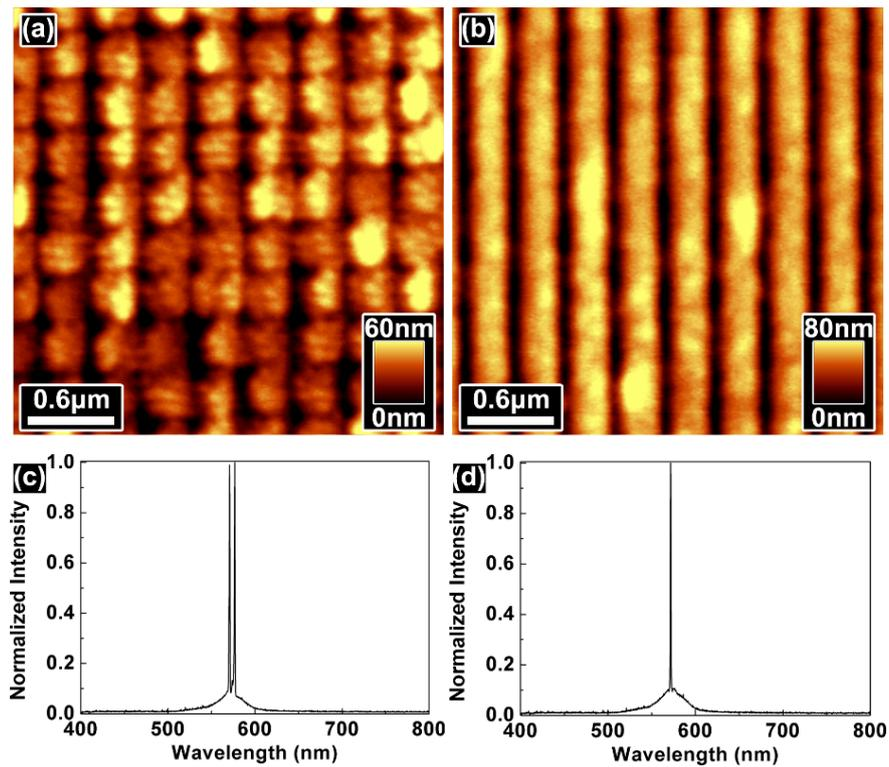
**Figure S3.** AFM images of polymer lasers based on (a) double-grating and (b) single-grating structures. The periods of two gratings in (a) are 355 nm and 360 nm, respectively. The period of the grating in (b) is 355 nm. Measured laser output spectra of (c) double-grating and (d) single-grating structures.
