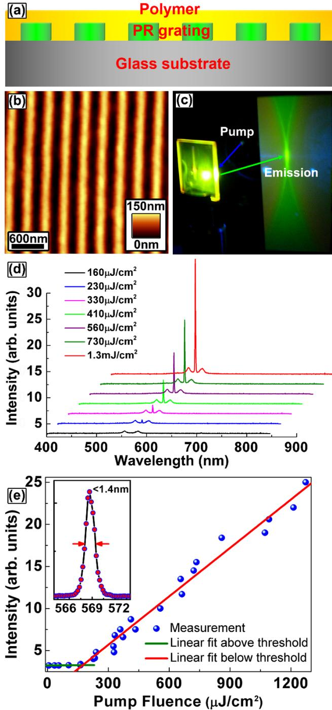
**Figure S2.** (a) The conventional design of the polymer laser with the active medium coated on top of the PR grating. (b) The AFM image of the grating. (c) The photograph of the operating polymer laser. (d) The spectra of the laser radiation at different pump fluence. (e) Output of the polymer laser as a function of the pump fluence, showing a pump threshold of about  $170 \mu\text{J}/\text{cm}^2$ . The linewidth of the laser output is less than  $1.4 \text{ nm}$  as shown in the inset.
