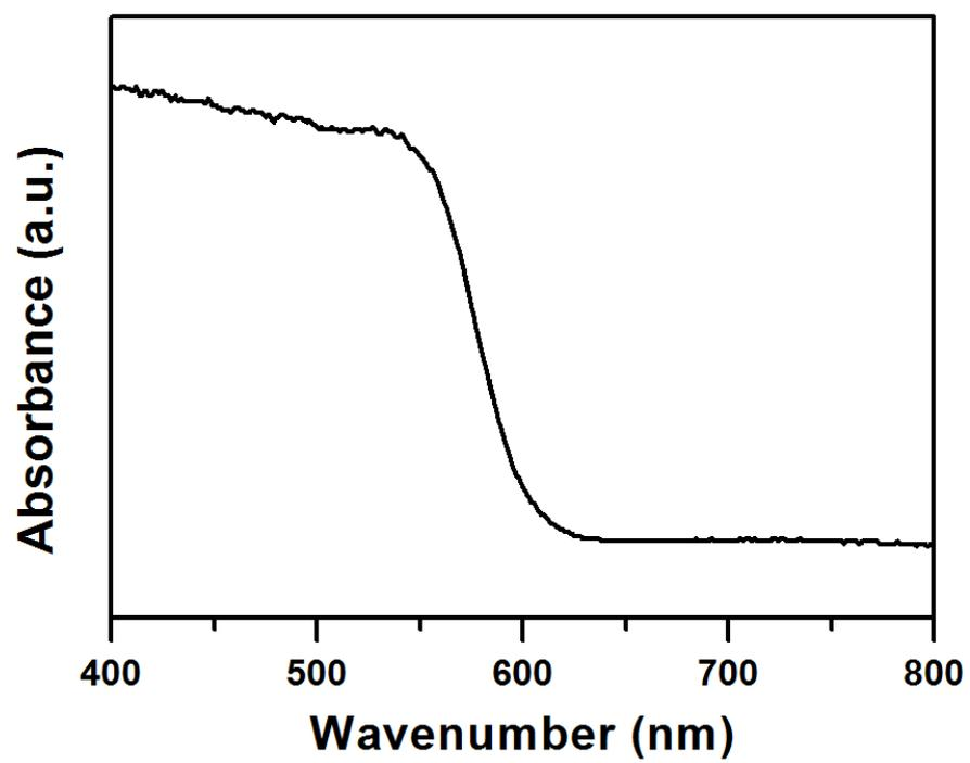
**Figure S2.** UV-Vis absorption spectrum of the Ta<sub>3</sub>N<sub>5</sub> NTAs.
