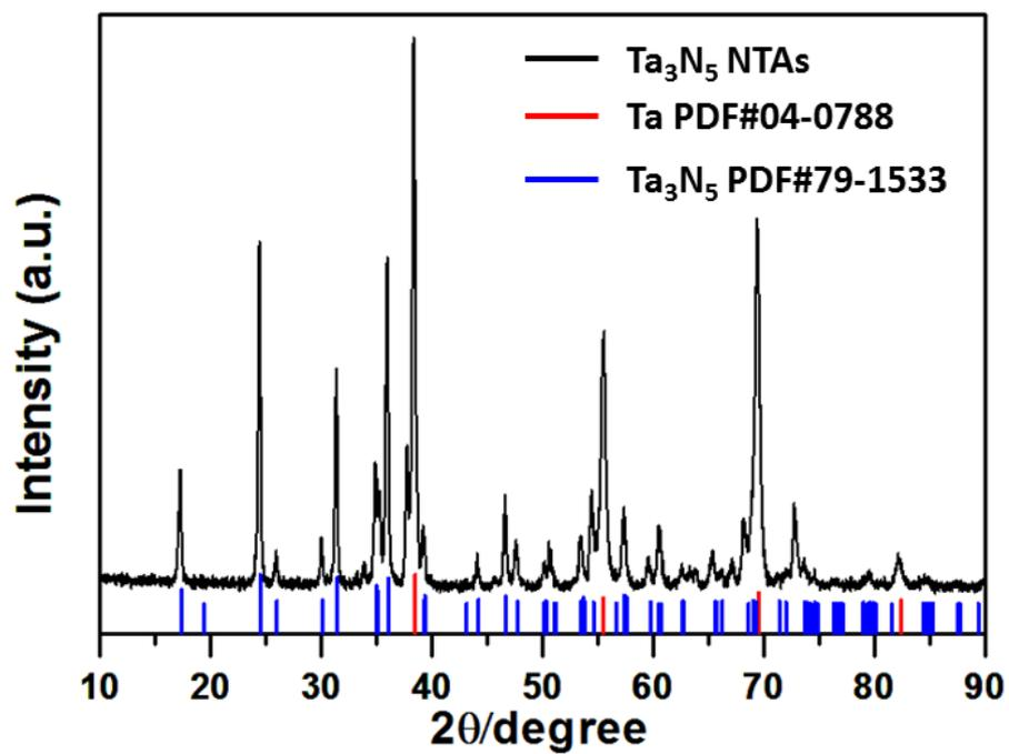
Figure S3. XRD pattern of the Ta<sub>3</sub>N<sub>5</sub> NTAs.
