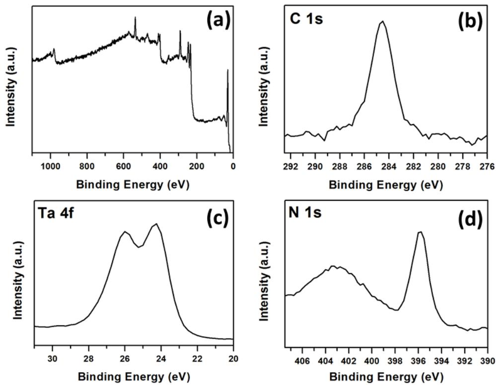
**Figure S4.** XPS spectra of (a) survey scan; (b) C 1s; (c) Ta 4f and (d) N 1s recorded from Ta<sub>3</sub>N<sub>5</sub> NTAs.
