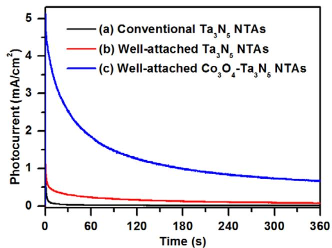
**Figure S6.** I-t curves of Ta<sub>3</sub>N<sub>5</sub> NTAs at 1.23 V vs. RHE: (a) Ta<sub>3</sub>N<sub>5</sub> NTAs synthesized by the conventional one-step anodization method; (b) Well-attached Ta<sub>3</sub>N<sub>5</sub> NTAs synthesized by the improved two-step anodization method (5 min, 25 V) and (c) Co<sub>3</sub>O<sub>4</sub> co-catalyst loaded Ta<sub>3</sub>N<sub>5</sub> NTAs in (b).
