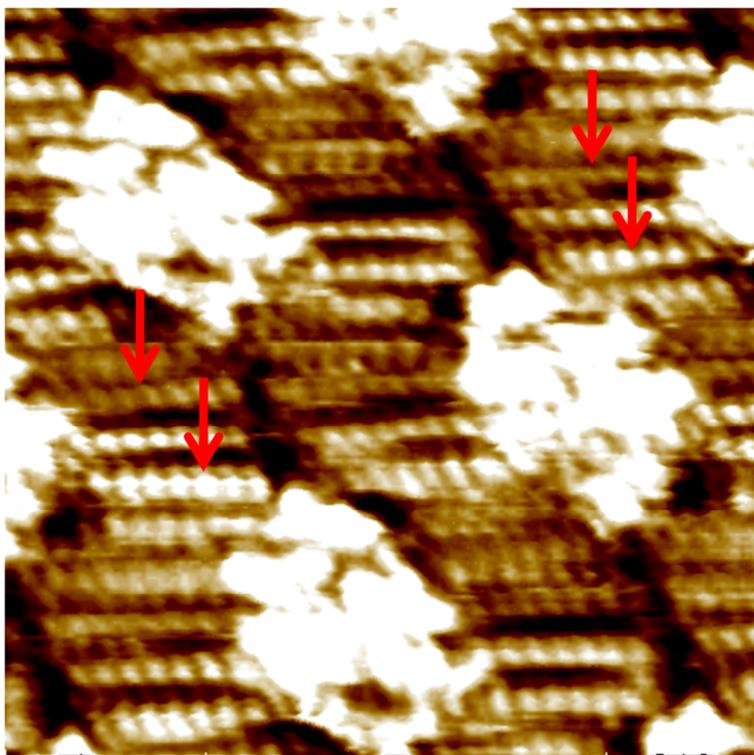
**Fig. S1** Higher-resolution STM image of hexamer pattern of HPF self-assembled adlayer in hexadecane ( $5.5 \times 10^{-7} \text{ mol L}^{-1}$ ) on HOPG surface, in which the coadsorbed solvents are indicated by the red arrows. Scan area:  $10 \times 10 \text{ nm}^2$ .
