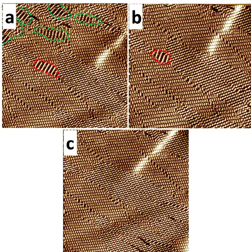
**Fig. S7** Large-scale STM images show that the homochiral close-packed hexamer and linear patterns transform into the multimer structure step by step by continuous scanning in pentadecane. Tunneling parameters:  $I_t = 568$  pA,  $V_b = 723$  mV. Scan area:  $200 \times 200$  nm<sup>2</sup>.
