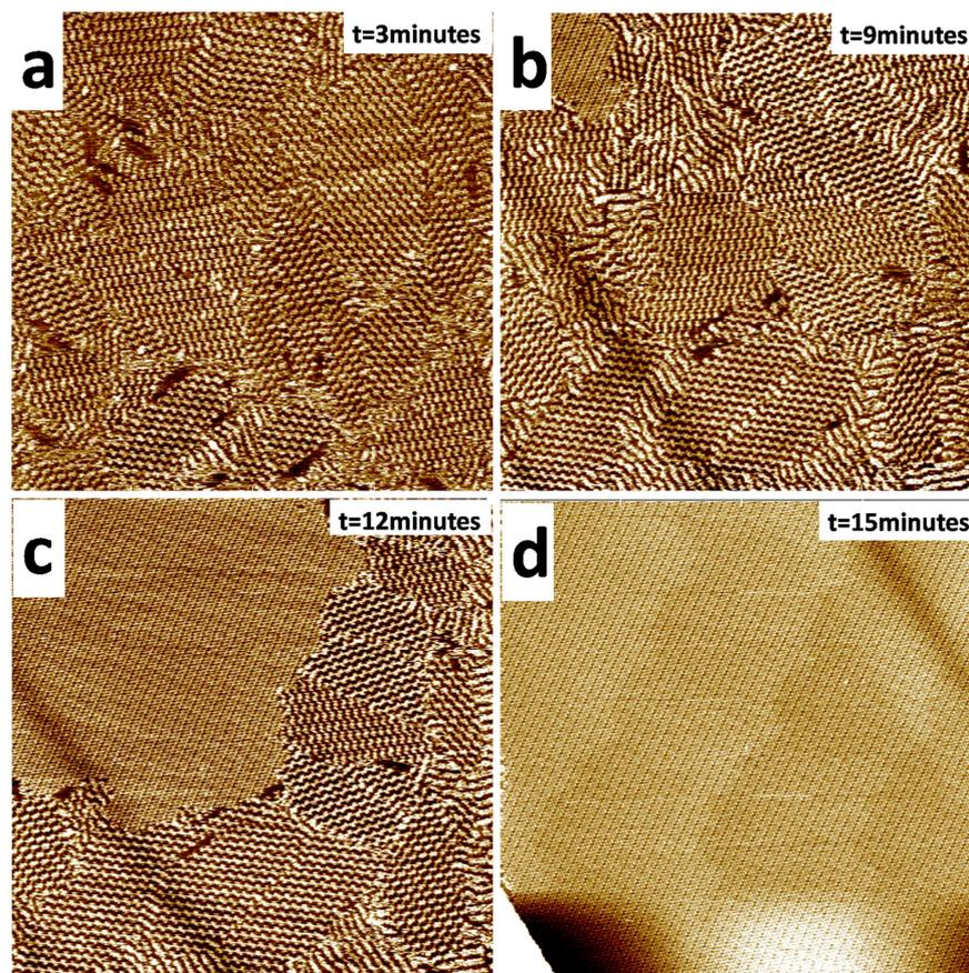
**Fig. S9** Large-scale STM images show that the multimer pattern can change into zigzag pattern in no time in tridecane. Tunneling parameters:  $I_t = 466$  pA,  $V_b = 574$  mV. Scan area:  $200 \times 200$  nm<sup>2</sup>.
