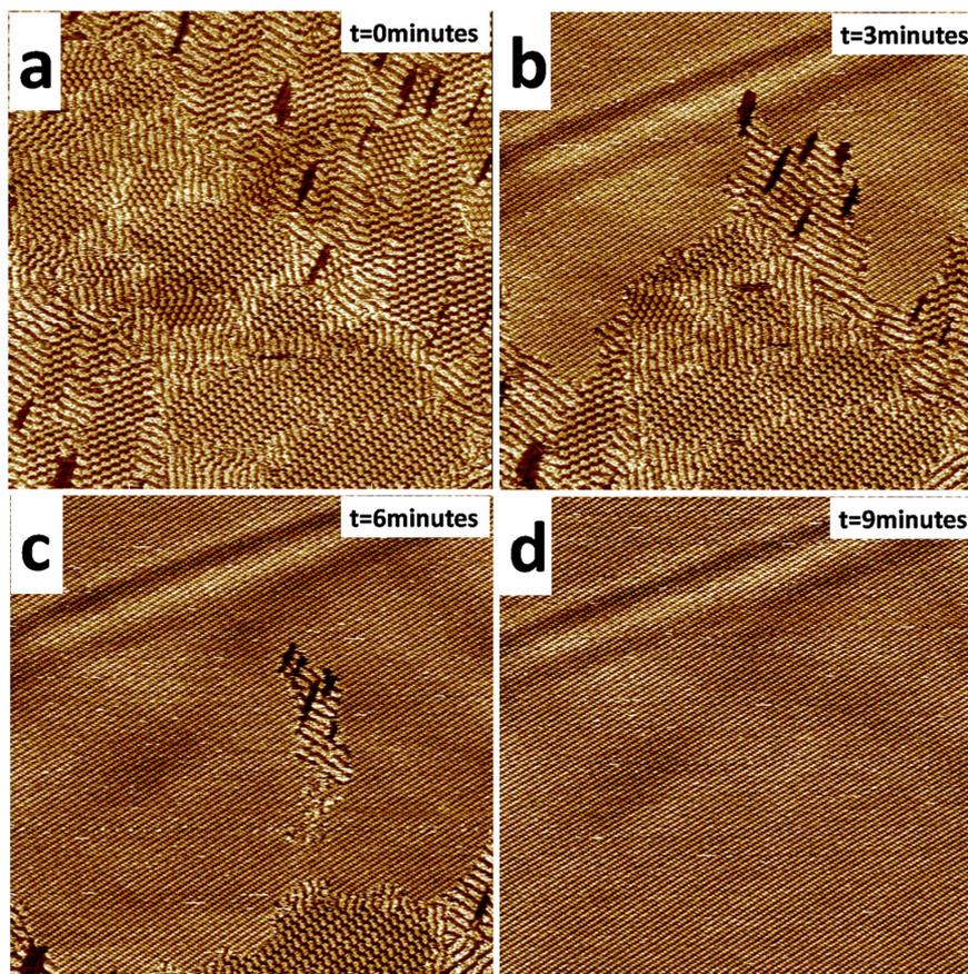
**Fig. S10** Large-scale STM images show that the close-packed hexamer and multimer patterns can convert into the zigzag pattern in high-speed in dodecane. Tunneling parameters:  $I_t = 485\text{pA}$ ,  $V_b = 717\text{ mV}$ . Scan area:  $200 \times 200\text{ nm}^2$ .
