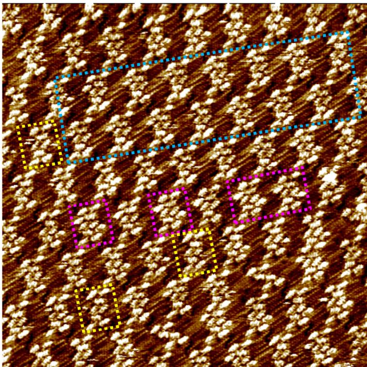
**Fig. S4** STM image of HPF self-assembly in hexadecane ( $5 \times 10^{-5}$  mol L<sup>-1</sup>) showing the multimer structure with three elementary structural units (8-, 9-, and 10-fold rings) composed. The yellow, blue, and pink dashed rectangles indicate the three kinds of multimer structures. No more than three continuous octamer or decamer are observed in the STM images. Tunneling parameters:  $I_t = 485$  pA,  $V_b = 665$  mV. Scan area:  $30 \times 30$  nm<sup>2</sup>.
