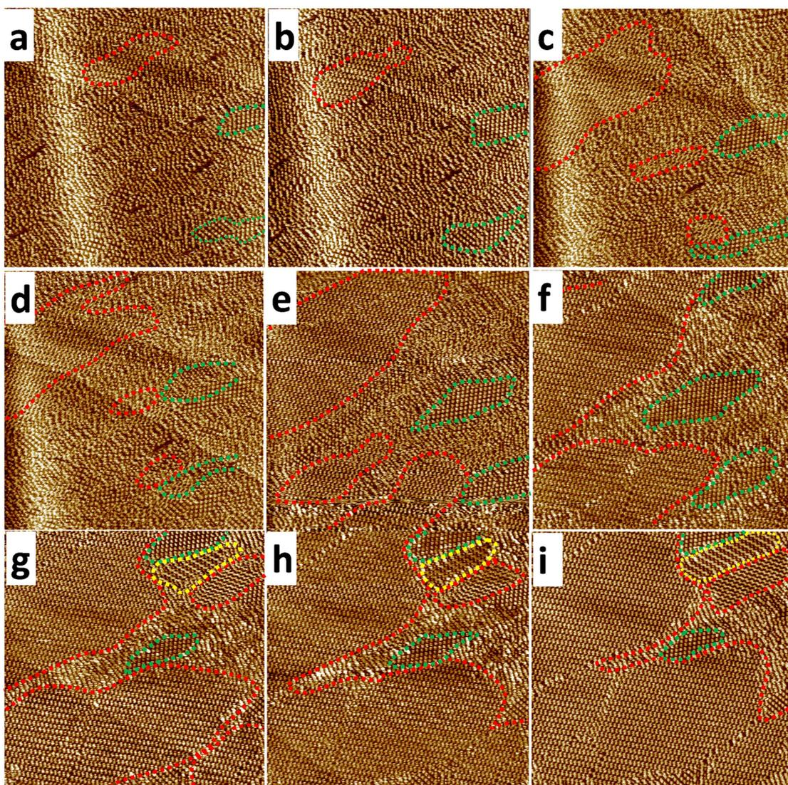
**Fig. S5** Large-scale STM images reveal that three well-organized chiral structures gradually transform into nonchiral multimer structure in hexadecane by consecutive scanning for more than three hours. Tunneling parameters:  $I_t = 545$  pA,  $V_b = 755$  mV. Scan area:  $200 \times 200$  nm<sup>2</sup>.
