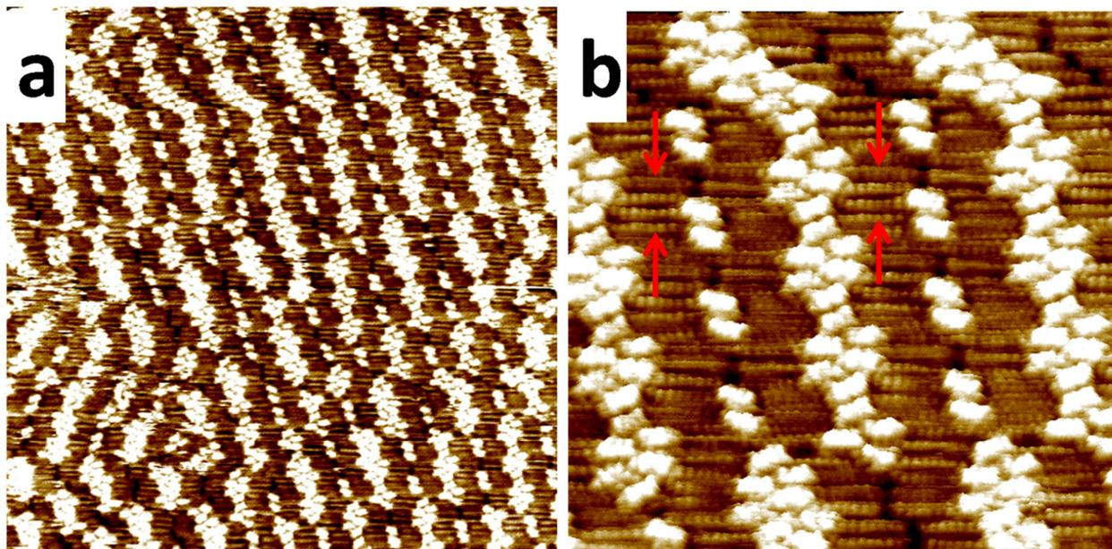
**Fig. S2** (a) Large-scale STM image of HPF self-assembly in hexadecane on HOPG surface showing the domain size for the alternate pattern is relatively small. Scan area:  $50 \times 50 \text{ nm}^2$ ; (b) High-resolution STM image of alternate pattern of HPF self-assembled adlayer in hexadecane ( $1.2 \times 10^{-6} \text{ mol L}^{-1}$ ) on HOPG surface, in which the coadsorbed solvents are indicated by the red arrows. Scan area:  $15 \times 15 \text{ nm}^2$ .
