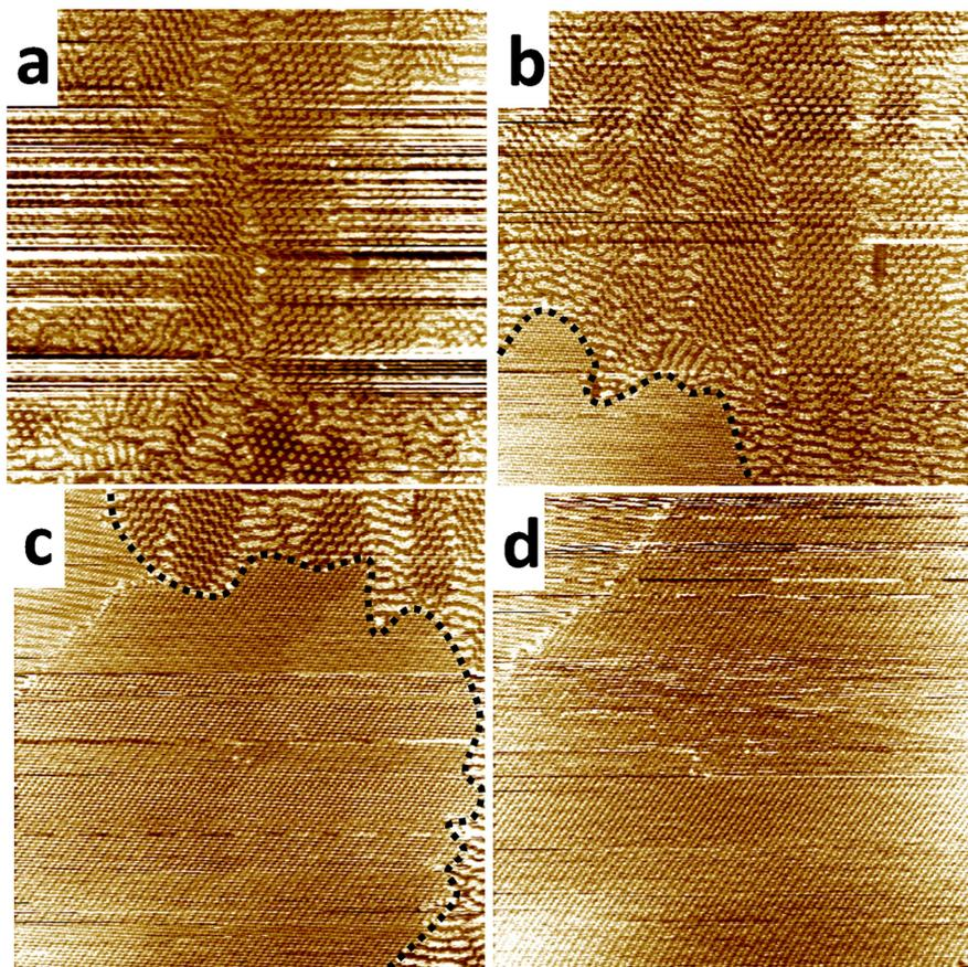
**Fig. S8** Large-scale STM images show that the multimer pattern can gradually transform into the zigzag pattern with the extension of scanning time in tetradecane. Tunneling parameters:  $I_t = 529$  pA,  $V_b = 705$  mV. Scan area:  $200 \times 200$  nm<sup>2</sup>.
