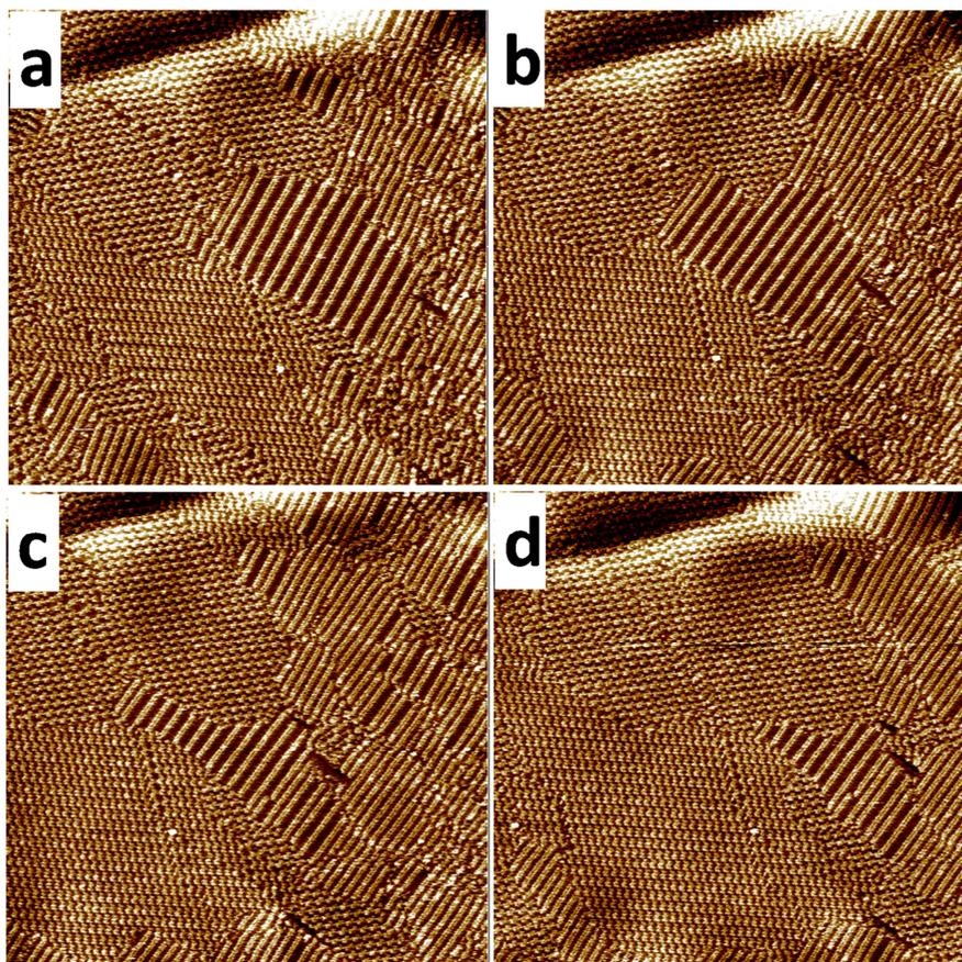
**Fig. S6** Large-scale STM images show that the linear pattern gradually transforms into the multimer structures with the extension of scanning time in pentadecane. Tunneling parameters:  $I_t = 443$  pA,  $V_b = 646$  mV. Scan area:  $200 \times 200$  nm<sup>2</sup>.
