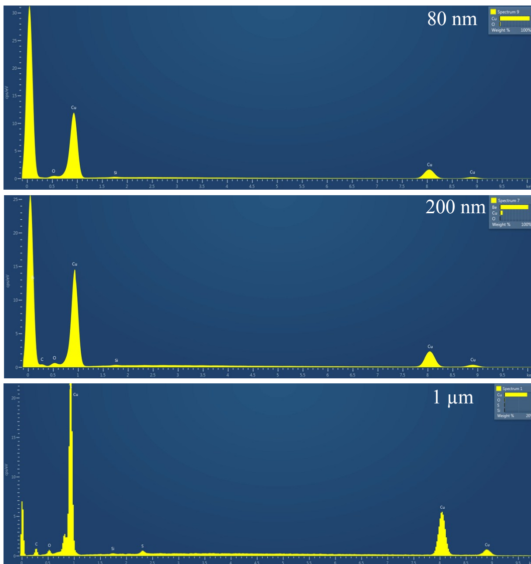
Figure S1. EDS spectra for the different samples synthesized with polycarbonate membranes having pore sizes of 80 nm, 200 nm and 1 μm, respectively.
