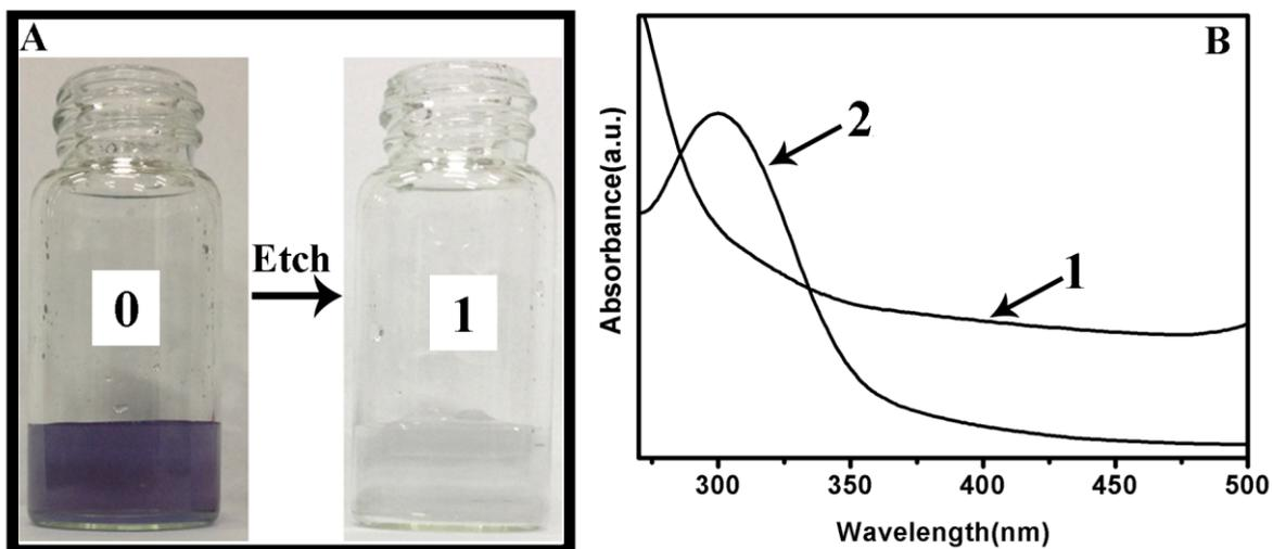
Fig. S8 The optical color of (A0) Au/Ag decahedra colloid and (A1) corresponding solution after complete etching; The UV-Vis spectra of HAuCl<sub>4</sub> (Curve 2 in Fig. 8B) and solution 1 in Fig. S8 A1 (Curve 1 in Fig. 8B).
