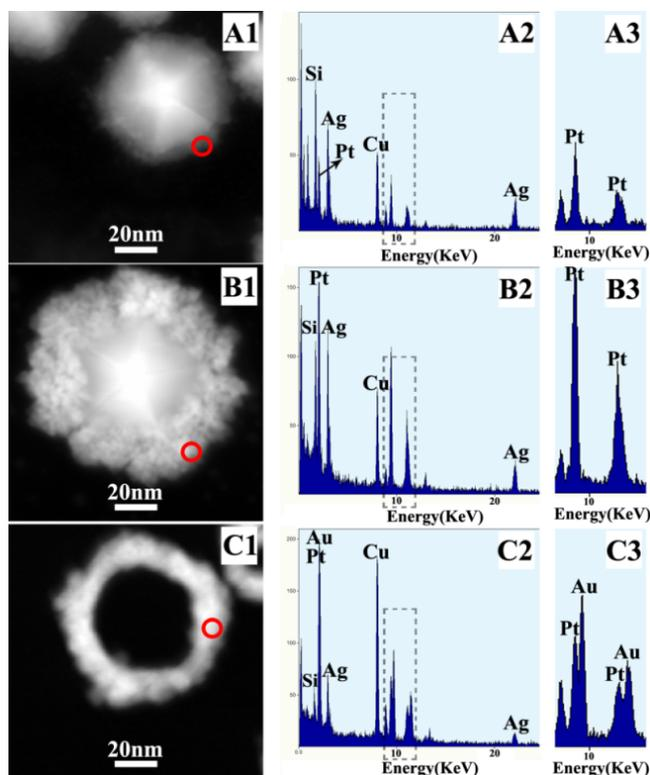
**Fig. S1** HAADF images and STEM-EDS analyses of products prepared using a standard synthesis of trimetallic nanorings after the reaction had proceeded for different times: (A1-A2) 30 min; (B1-B2) 60 min; (C1-C2) 120 min. A3, B3 and C3 are the enlarged images of areas marked by the dotted box in **Fig. S1A2**, **Fig. S1B2** and **Fig. S1C2** respectively.
