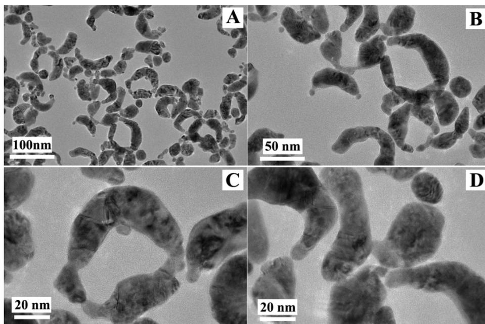
Fig. S3 (A-D) TEM and HRTEM images of products using a standard procedure of trimetallic nanorings except that the reaction time was 150 min.
