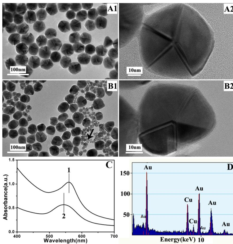
Fig. S5 TEM images of Au/Ag decahedra (A1-A2). (B1-B2) TEM images of products prepared using Au/Ag decahedra as seeds in a standard synthesis of trimetallic nanorings except that no  $\text{H}_2\text{PtCl}_6$  was added. (C) UV-Vis spectra of Au/Ag decahedra shown in Fig. S5A (Curve 1) and colloid shown in Fig. S5B (Curve 2). (D) EDS pattern of nanoparticles marked by the arrow in Fig. S5 B1.
