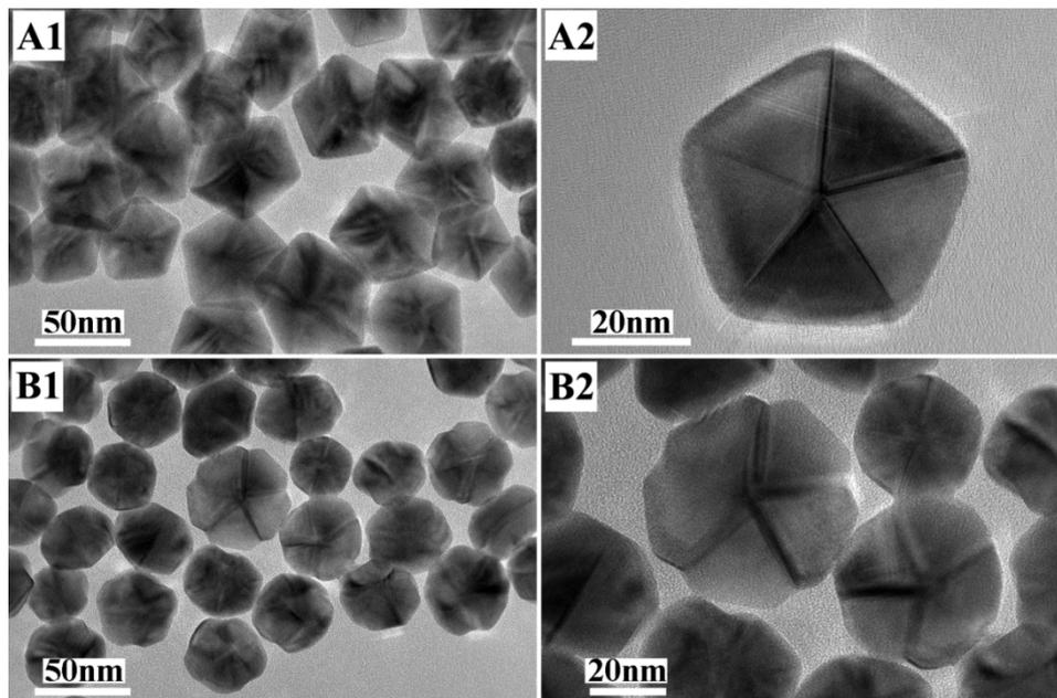
Fig. S6 TEM images of Au/Ag decahedra colloid and corresponding products prepared using a standard synthesis of trimetallic nanorings except that no AA and  $H_2PtCl_6$  were added (Reaction time was 12 h).
