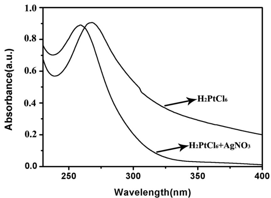
Fig. S9 UV-Vis spectra of H<sub>2</sub>PtCl<sub>6</sub> aqueous solution and mixture (H<sub>2</sub>PtCl<sub>6</sub> and AgNO<sub>3</sub>).
