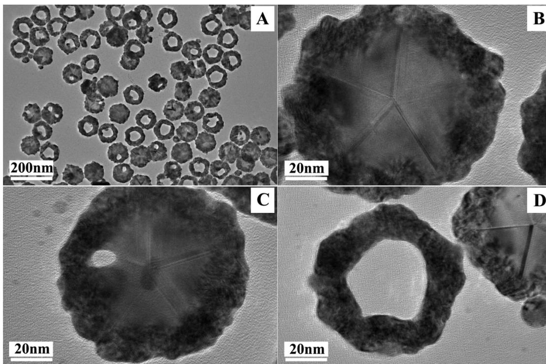
Fig. S2 (A-D) TEM images of products prepared using a standard procedure of trimetallic nanorings except that the reaction time was 90 min. This demonstrates that the etching on each decahedron is not uniform.
