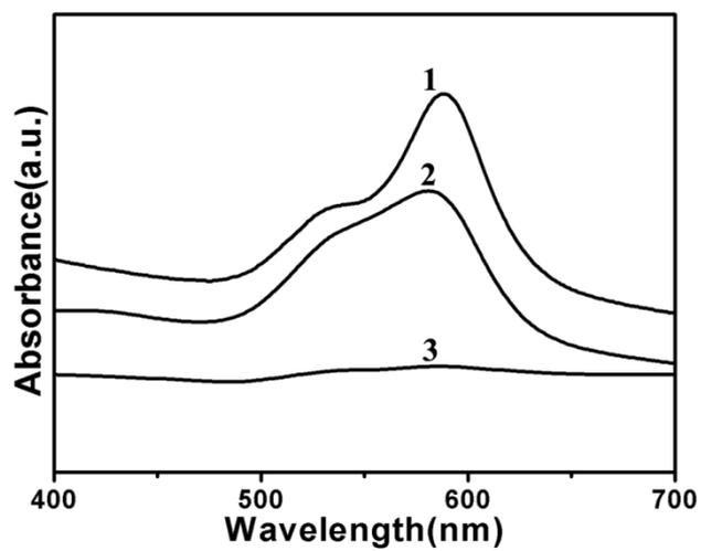
Fig. S7 UV-Vis spectra of Au/Ag decahedra colloid (Curve 1), colloid etched for 12 h in solution containing PVP as protecting agents (Curve 2), colloid etched for 150 min in solution containing PVP as protecting agents and 0.001 M  $H_2SO_4$  (Curve 3).
