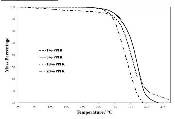
**Figure 1 :** TGA thermograms for the poly(CTFE-*alt*-iBVE) copolymers under air at 10 °C/min.
