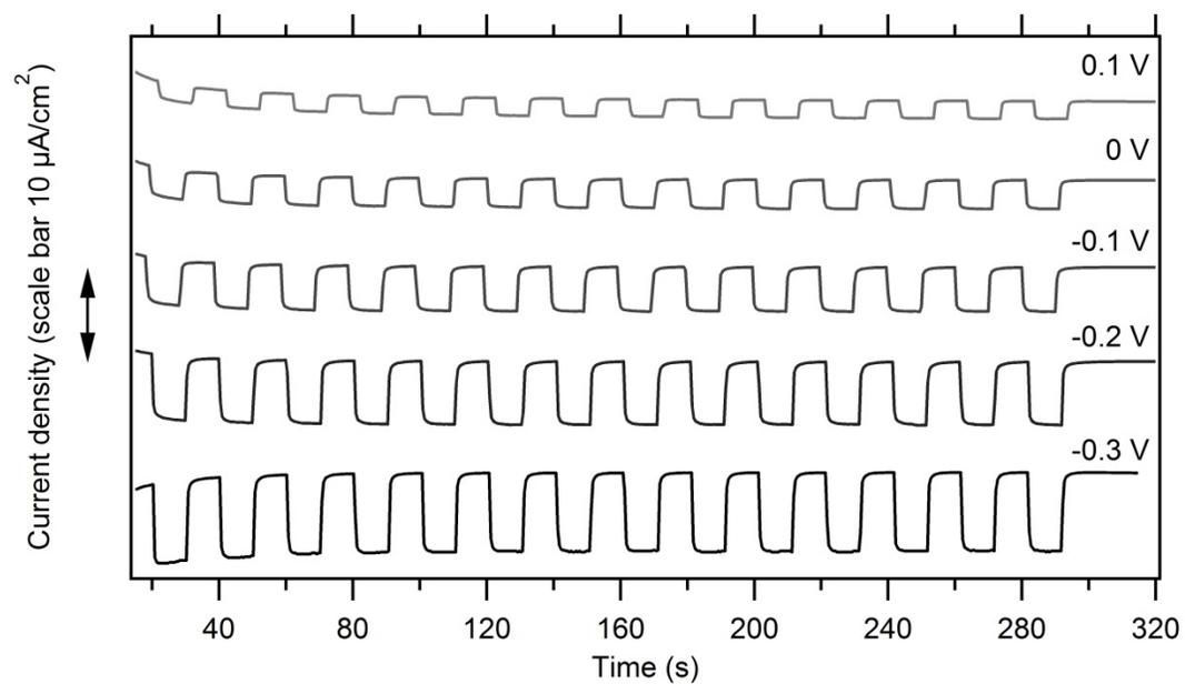
**Fig. S12** Chronoamperometric measurements of a diamond foam electrode sensitized with **BT-Rho** at different bias voltages. Chopped white light illumination ( $50 \text{ mW}/\text{cm}^2$ ; simulated AM 1.5G solar spectrum). Electrolyte solution: 5 mM methyl viologen in 0.1 M  $\text{Na}_2\text{SO}_4$ . The applied bias voltages (vs. Ag/AgCl) are indicated in annotations.
