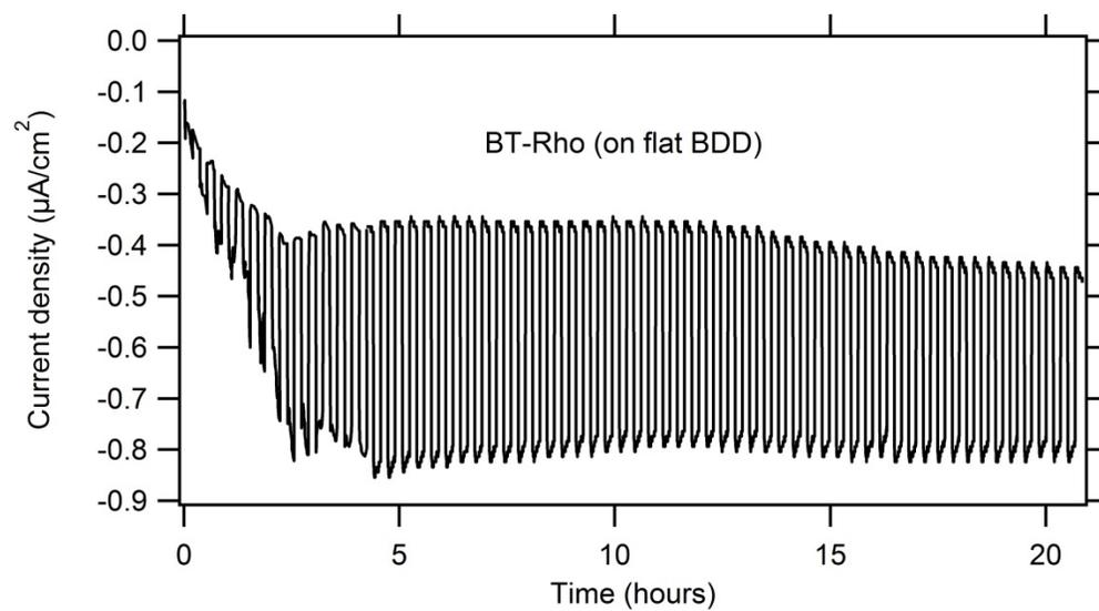
**Fig. S13** Long-term chronoamperometric measurement of a flat B-doped diamond electrode sensitized with **BT-Rho**. Chopped white light illumination ( $100 \text{ mW/cm}^2$ ; simulated AM 1.5G solar spectrum, 10 min dark/light interval). Electrolyte solution: 5 mM methyl viologen in 0.1 M  $\text{Na}_2\text{SO}_4$ . Applied potential bias:  $-0.3 \text{ V}$  vs. Ag/AgCl.
