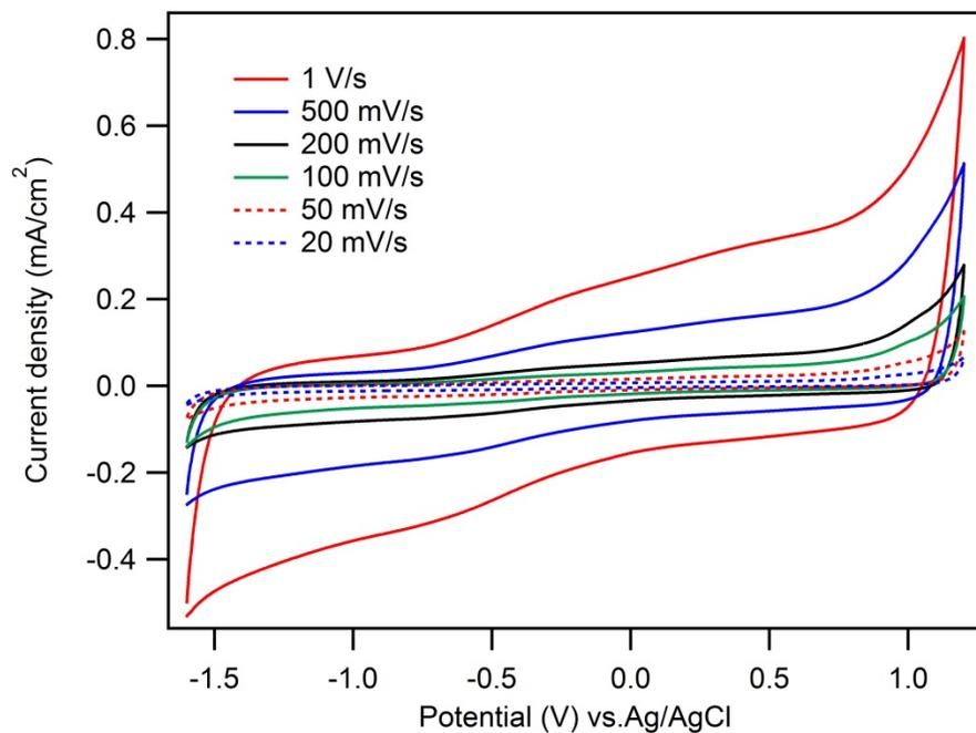
**Fig. S6** Cyclic voltammogram of a pristine BDD foam electrode in phosphate buffer pH 7 (Sigma Aldrich) at different scan rates (see annotation labels).
