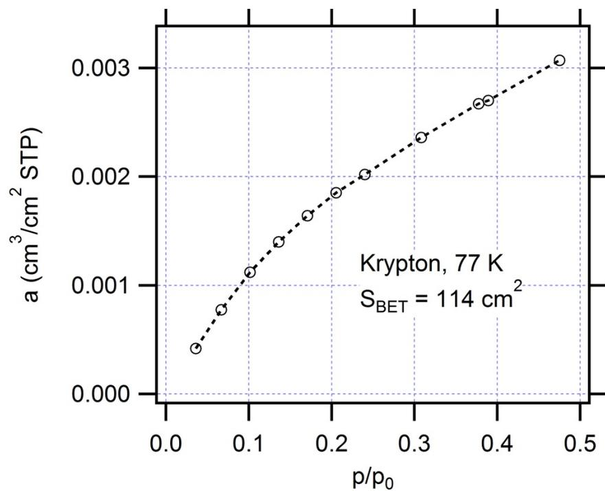
**Fig. S5** Adsorption isotherm of Kr at a pristine BDD foam electrode; geometric area 1 cm<sup>2</sup>. From the found S<sub>BET</sub> of the sample and its projected geometric area, the roughness factor,  $R_f$ , equals 114.
