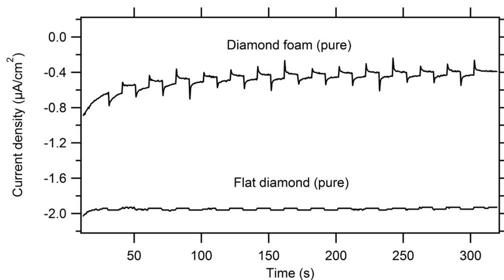
**Fig. S8** Chronoamperometric measurement on a pure (non-sensitized) diamond foam compared to that on a pure (non-sensitized) flat diamond film. Chopped white light illumination ( $20 \text{ mW}/\text{cm}^2$ ; simulated AM 1.5G solar spectrum). Electrolyte solution: 5 mM methyl viologen in 0.1 M  $\text{Na}_2\text{SO}_4$  pH 7. Applied potential bias: -0.3 V vs. Ag/AgCl.
