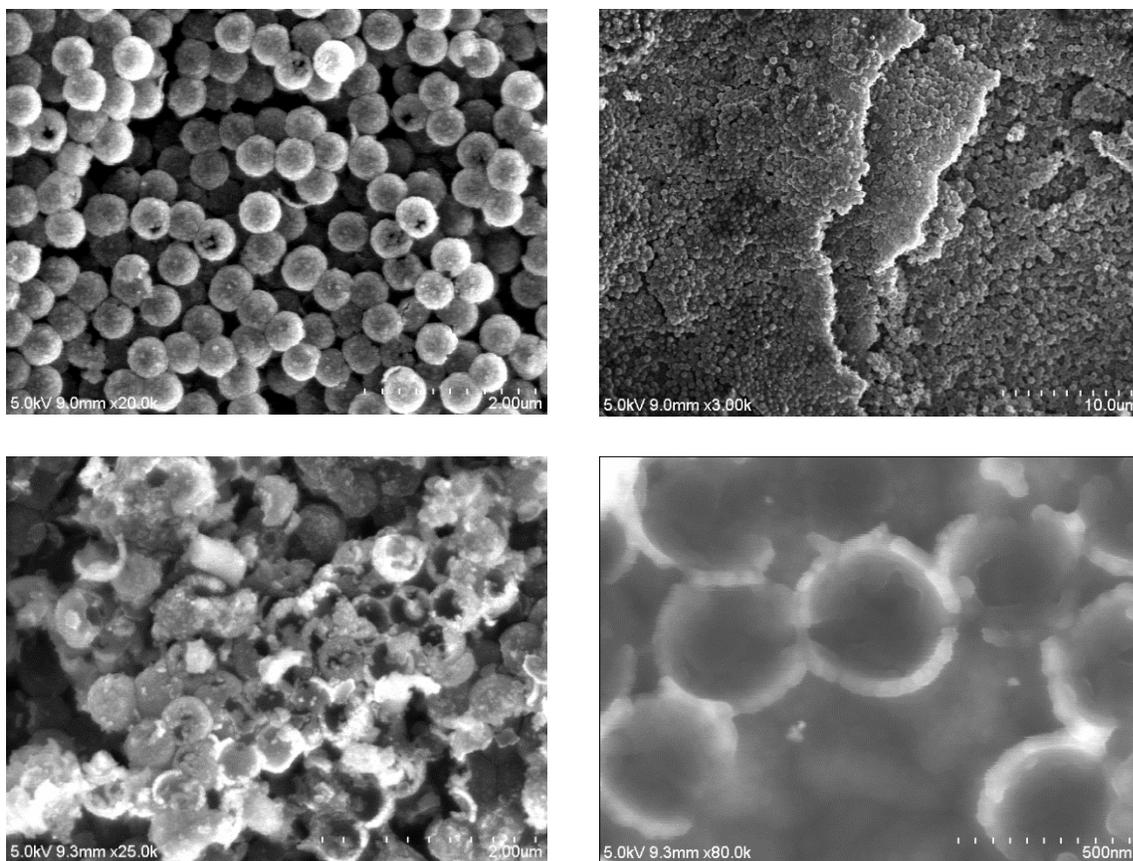
**Fig. S2** SEM images of B-doped diamond foam electrodes sensitized with **BT-Rho**. Holes in the diamond shell are obvious on the top-left image. Heavily damaged structures are seen on the bottom images. The multilayer morphology of the diamond foam electrodes is apparent from the top-right image.
