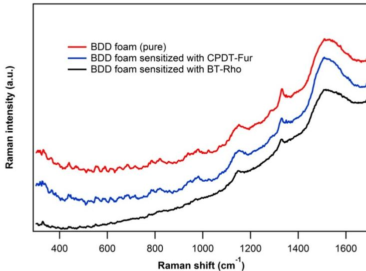
**Fig. S3** Raman spectra (at 458 nm excitation) of a pristine BDD foam electrode and those sensitized with **CPDT-Fur** and **BT-Rho**. The diamond peak is seen at 1330 cm<sup>-1</sup>. The main impurity peaks are *trans*-polyacetylene (1150 cm<sup>-1</sup>) and a broad G-peak of sp<sup>2</sup> carbon at ca. 1500 cm<sup>-1</sup>. The absence of features around 500 cm<sup>-1</sup> indicates removal of SiO<sub>2</sub> and low B-doping.
