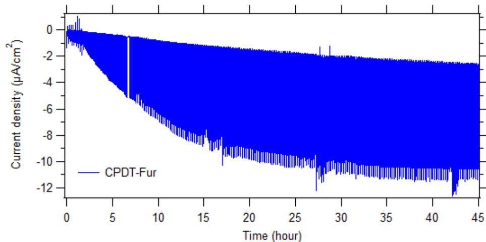
**Fig. S7** Long-term chronoamperometric measurement of the diamond foam electrode sensitized with **CPDT-Fur**. Chopped white light illumination ( $100 \text{ mW/cm}^2$ ; simulated AM 1.5G solar spectrum, 5 min dark/light interval). Electrolyte solution: 5 mM methyl viologen in 0.1 M  $\text{Na}_2\text{SO}_4$ , pH 7. Applied potential bias:  $-0.3 \text{ V}$  vs. Ag/AgCl.
