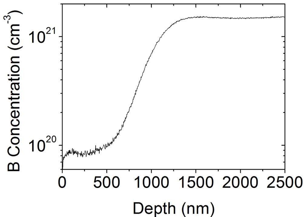
**Fig. S1** SIMS analysis of a BDD foam electrode (one layer). The concentration of B-atoms is between  $7$  and  $10 \cdot 10^{19} \text{ cm}^{-3}$  for the foam layer, which is about  $500 \text{ nm}$  thick (corresponding to one layer of templated hollow spheres). The compact layer underneath the porous film is highly doped to  $>10^{21} \text{ cm}^{-3}$ .
