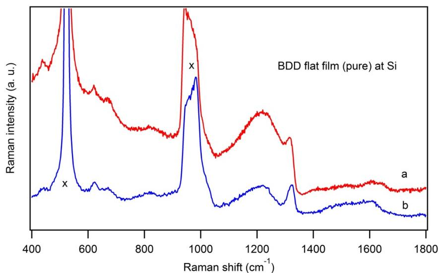
**Fig. S4b** Raman spectrum of a pristine flat BDD film electrode on a Si substrate. Excitation wavelengths 633 nm (a), 488 nm (b). The Raman features from the substrate are marked with an asterisk.
