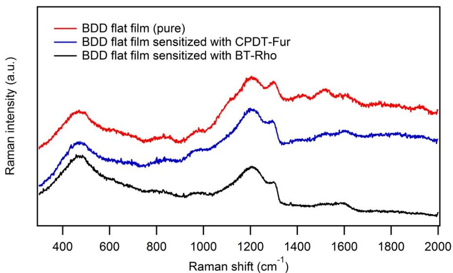
**Fig. S4a** Raman spectra (at 633 nm excitation) of a pristine flat BDD film electrode on a  $\text{SiO}_2$  substrate and those sensitized with **CPDT-Fur** and **BT-Rho**.
