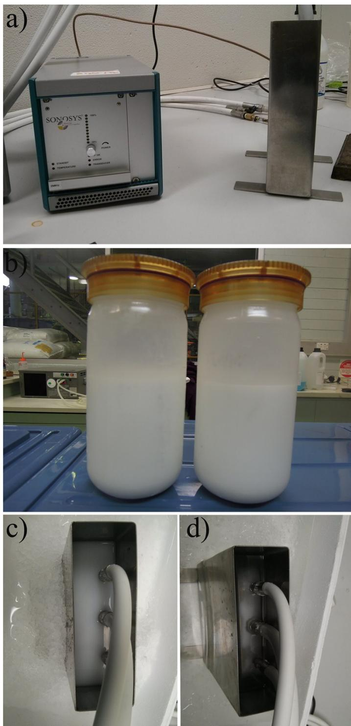
**Figure S7.** (a) Photograph of the megasonics unit using a 1L container for the separation and washing steps. (b) Image showing the Al-Fumarate solutions produced with the flow reactor (Salamander) that are employed for testing the megasonics technique. (c) Image of the initial MOF solution into the 1L stainless steel vessel before applying the high frequency. (d) Image after applying a 2 MHz frequency after 10 minutes.
