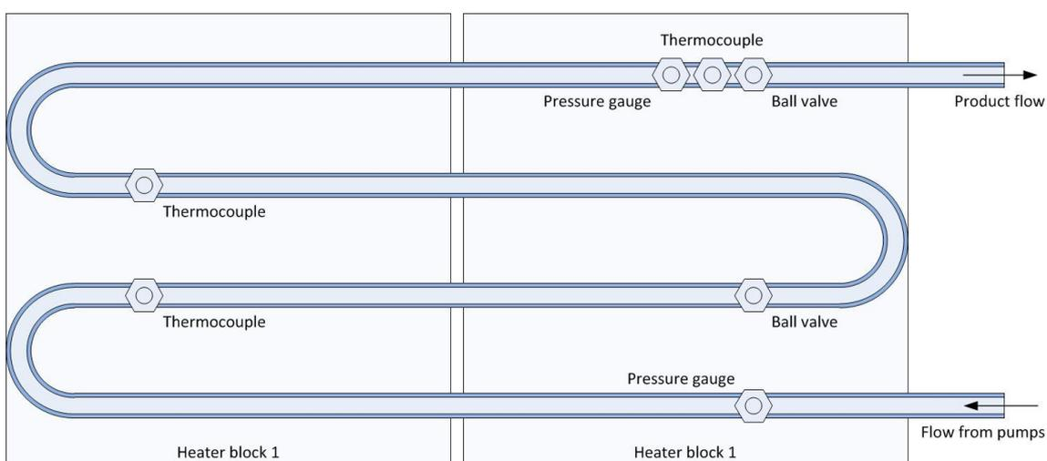
**Figure S1.** Photograph and schematic of the Salamander Flow Reactor (Cambridge Reactor Design) used for the large-scale production of the Al-Fumarate and MIL-53 MOFs. The system is comprised of two HPLC pumps (Gilson), a 108 mL stainless steel tubing reactor (0.6 mm i.d.), and custom static mixers throughout the length of tubing.
