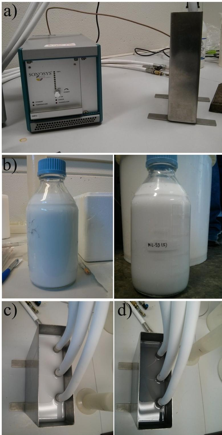
**Figure S8.** (a) Photograph of the megasonics unit using a 1L container for the separation and washing steps. (b) Image showing the MIL-53 solutions produced with the flow reactor (Salamander) that are employed for testing the megasonics technique. (c) Image of the initial MOF solution into the 1L stainless steel vessel before applying the high frequency. (d) Image after applying a 2 MHz frequency after 10 minutes.
