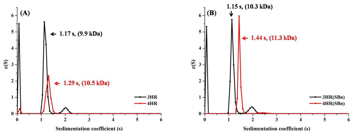
**Fig. S3.** Sedimentation velocity analysis of (A) 4HR and 3HR peptides and (B) 4HR(SBn) and 3HR(SBn).
