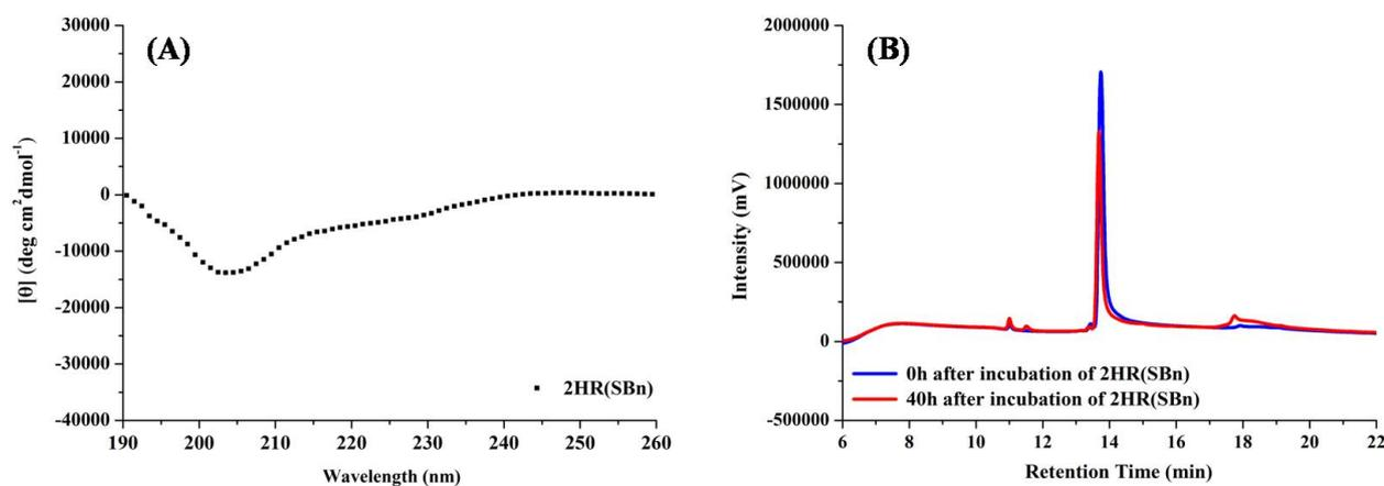
**Fig. S5.** (A) CD spectra of 2HR(SBn). (B) RP-HPLC traces of 2HR(SBn) at  $t=0$  and 40 h.
