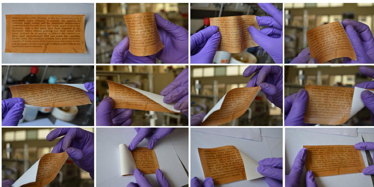
**Figure S24:** Mechanical Deformation of a Mg-NDI coated paper after printing content on it. It was observed that the contents remained clearly visible even after all kind of deformations applied to it.
