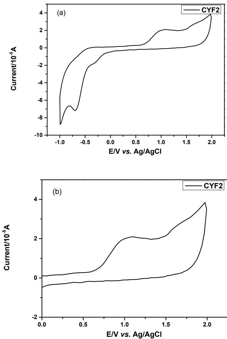
Figure S2. (a) Cyclic voltammograms and (b) partial cyclic voltammograms of **CYF2** on  $\text{TiO}_2$  in 0.1 M TBAPF<sub>6</sub> of CH<sub>2</sub>Cl<sub>2</sub> solution measured with a scan rate of 50 mV s<sup>-1</sup>.
