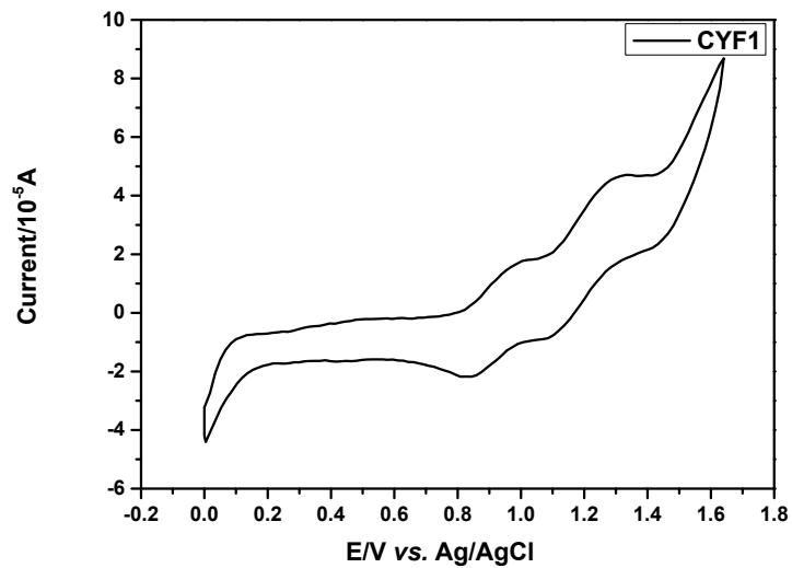
Figure S1. Cyclic voltammograms of **CYF1** on  $\text{TiO}_2$  in 0.1 M TBAPF<sub>6</sub> of CH<sub>2</sub>Cl<sub>2</sub> solution measured with a scan rate of 50 mV s<sup>-1</sup>.
