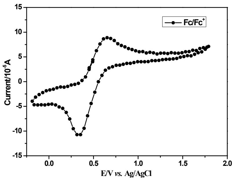
Figure S3. Cyclic voltammograms of  $\text{Fc}/\text{Fc}^+$  in 0.1 M TBAPF<sub>6</sub> of CH<sub>2</sub>Cl<sub>2</sub> solution measured with a scan rate of 50 mV s<sup>-1</sup>.
