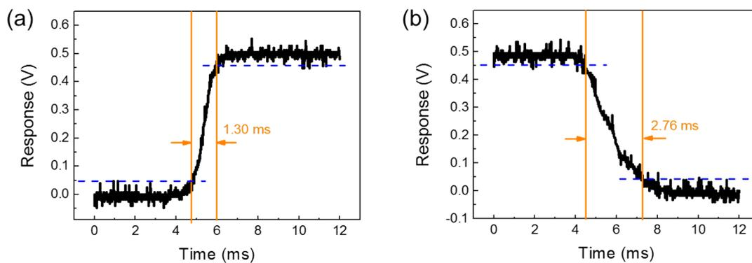
**Figure S5.** (a) Response and (b) recovery of the TiO<sub>2</sub>/graphene/Si device. The response and recovery times are confirmed as the time interval from 10% to 90% (90% to 10%) of its peak value.<sup>1,2</sup>
