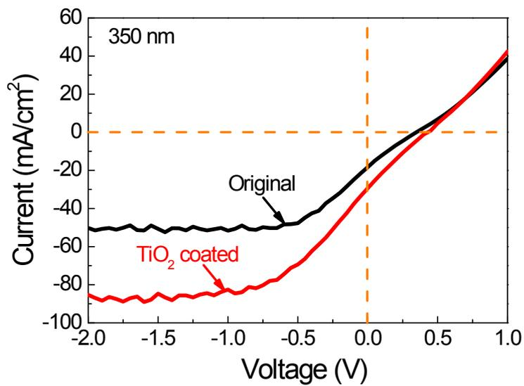
**Figure S3.** *I-V* characteristics of the device before and after TiO<sub>2</sub> coating, tested at 350 nm incident light.
