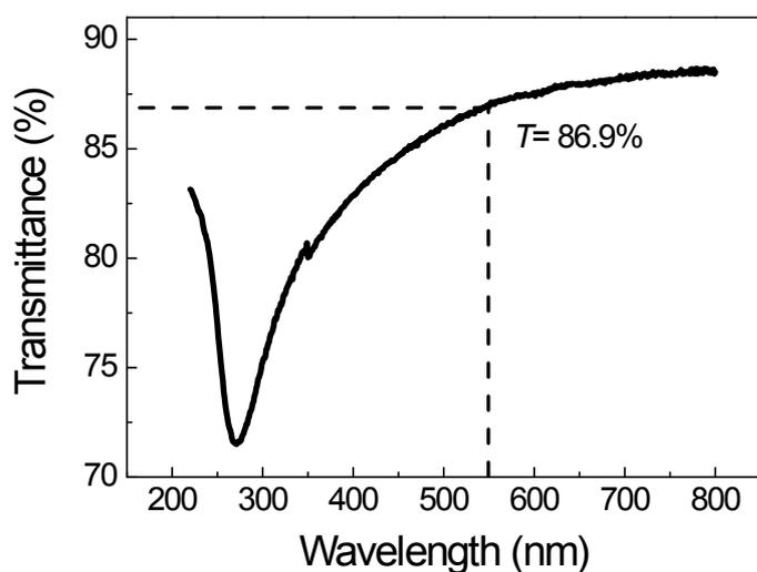
**Figure S1.** Transmittance of graphene. The transmittance is about 86.9% at 550 nm, corresponding to a thickness of ~2 nm (the number of layers is ~6).
