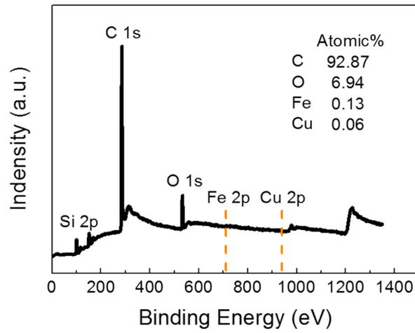
**Figure S2.** XPS of as-prepared graphene (on Si substrate). The contents of metallic impurities (*e.g.*, Fe, Cu) in graphene are quite low.
