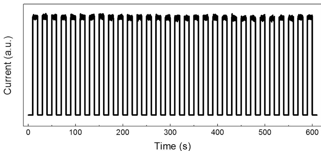
**Figure S4.** Response repeatability of the switching behavior of TiO<sub>2</sub>/graphene/Si device in 10 min.
