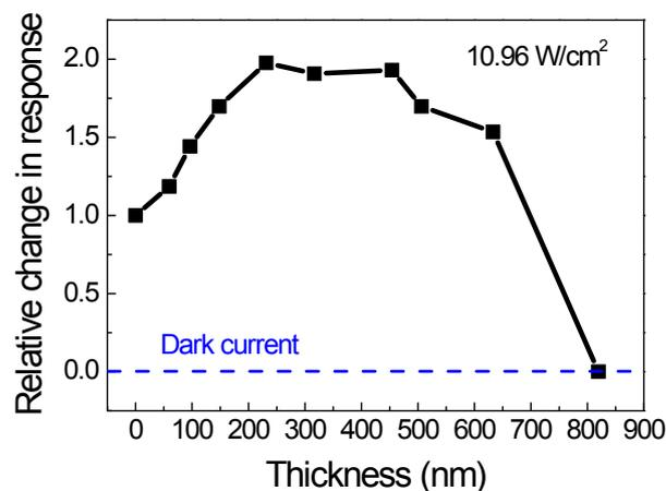
**Figure S6.** Relative change of the response current versus the thickness of TiO<sub>2</sub> layer.
