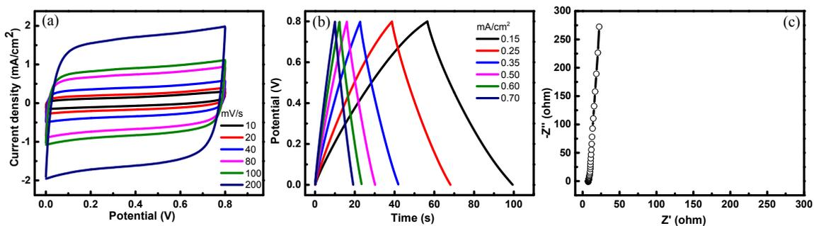
**Fig. S3** (a) CV and (b) CDs of symmetric PEDOT/Au/PEN//PEDOT/Au/PEN solid state device using PVA/H<sub>2</sub>SO<sub>4</sub> gel electrolyte. (c) Nyquist plot for the symmetric PEDOT solid state device.
