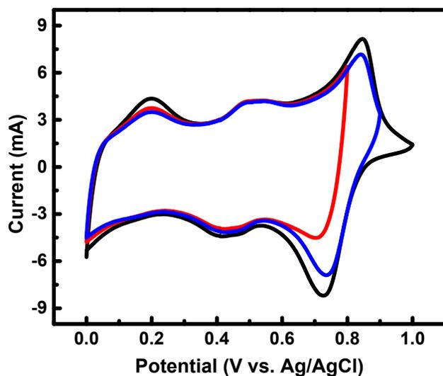
**Fig. S4** CVs of PANI in different positive potential windows at a scan rate of 80 mV/s. CV is getting narrow down above the potential of 0.8 V.
