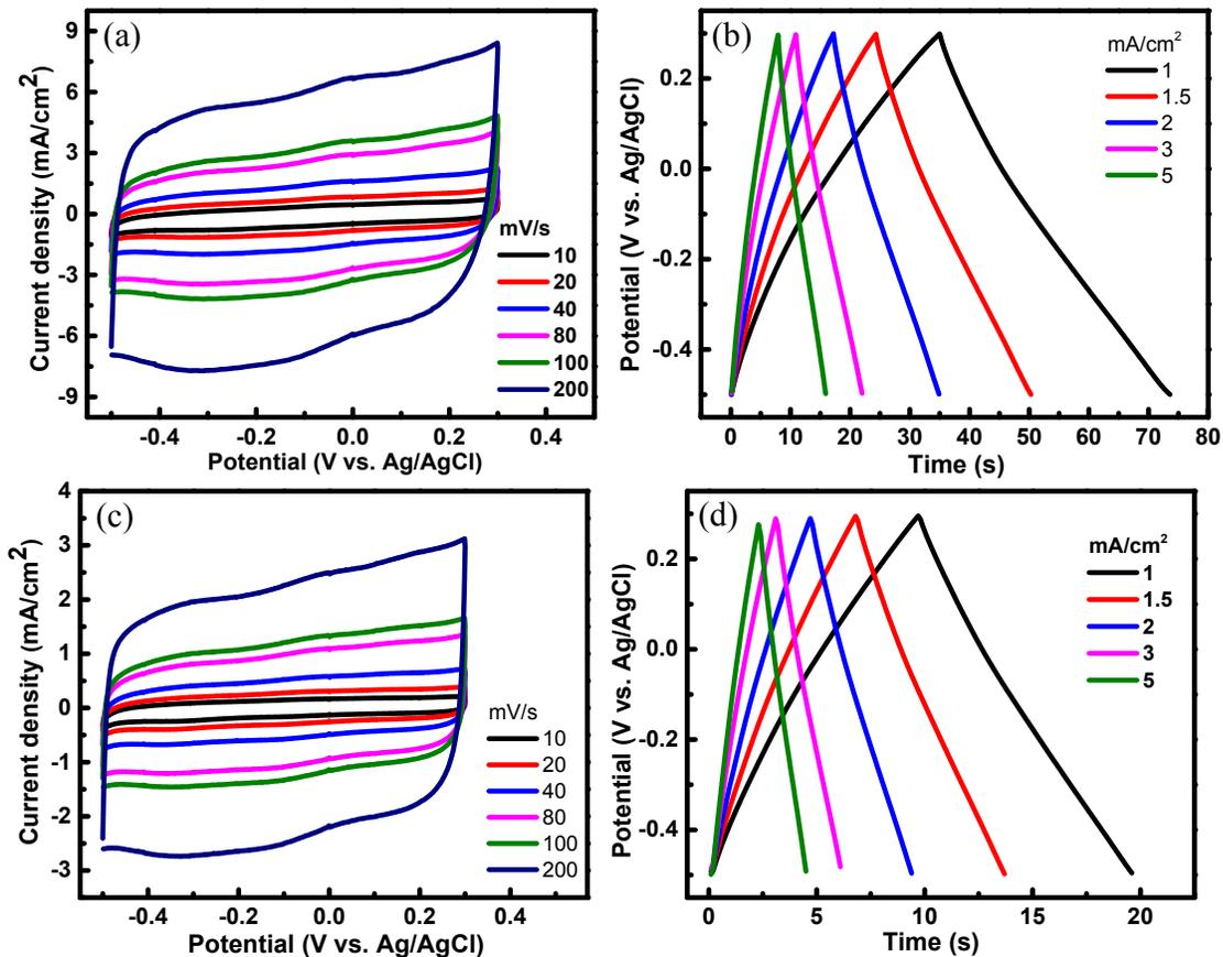
**Fig. S2** (a) and (b) CV and CD of 5 minute deposited PEDOT sample. (c) CV and (d) CD of 15 minute deposited PEDOT sample.
