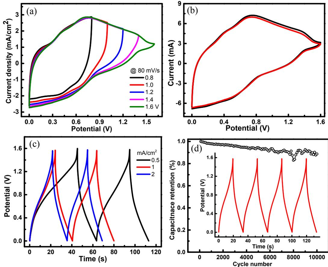
**Fig. S6** (a) CVs of ASC device at a scan rate of 80 mV/s in different potential windows. (b) CV scans at a scan rate of 80 mV/s and (c) CDs of ASC device at different current densities after 100 cycles of charging and discharging. (d) Cycling stability of the optimized PANI//PEDOT ASC solid state supercapacitor over 10,000 cycles. Inset shows the charge-discharge curves at a current density of 2 mA/cm<sup>2</sup>.
