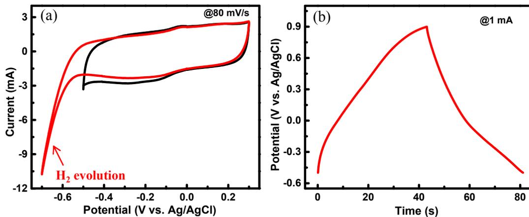
**Fig. S1** (a) CVs of PEDOT in different negative potential windows. (b) Charge-discharge curve for the PEDOT in a wide potential window of 1.4 V.
