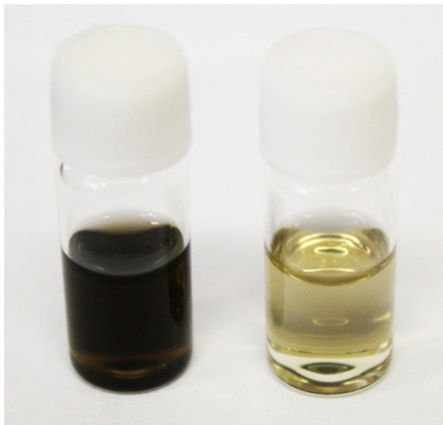
Figure S3. Dispersion of AZO-RGO in DMF. AZO-RGO hybrid ( 1 \text{ mg mL}^{-1} ) shows well dispersion after standing undisturbed for three month (left) and dilute dispersion with an initial absorbance 1.5 of AZO-RGO is used for photoisomerization measurements (right) without any precipitate.
