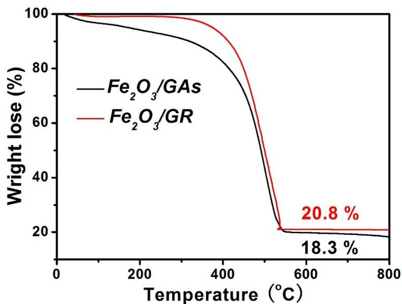
**Figure S1.** A typical TGA curve obtained for the Fe<sub>2</sub>O<sub>3</sub>/GAs and Fe<sub>2</sub>O<sub>3</sub>/GR under O<sub>2</sub> atmosphere.
