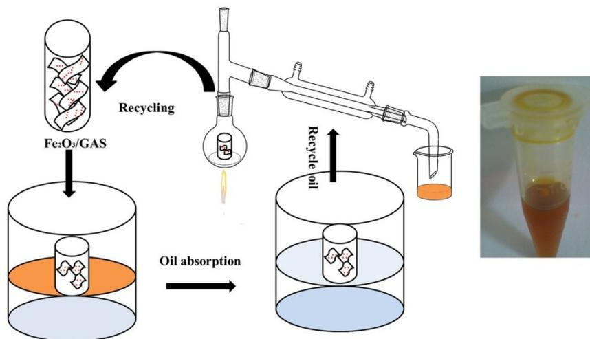
**Figure S6.** Schematic illustration of the recycle the Fe<sub>2</sub>O<sub>3</sub>/GAs and the oil by the one-step distillation method.
