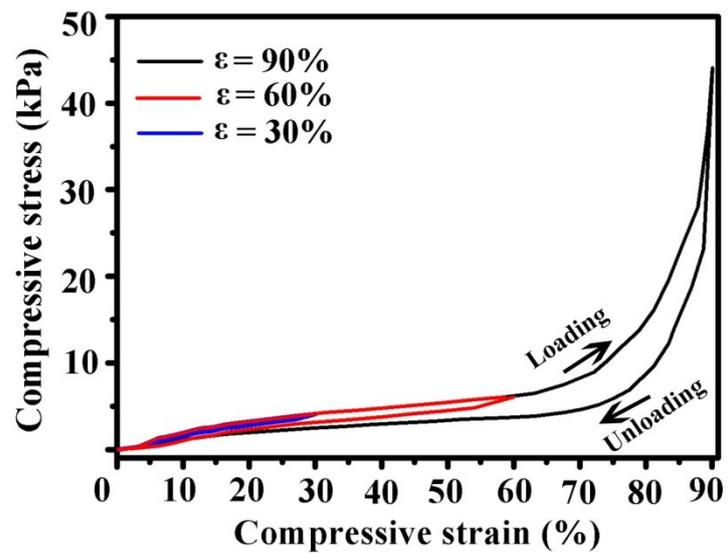
**Figure S5.** Compressive stress–strain curves of a CNF aerogel at different set strain  $\epsilon$  of 30, 60, and 90%.
