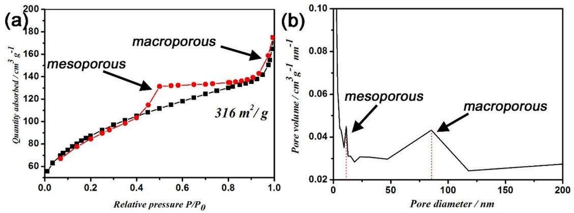
**Figure S2.** (a) Nitrogen adsorption-desorption isotherms of Fe<sub>2</sub>O<sub>3</sub>/GAs, and (b) its corresponding pore size distribution curves.
