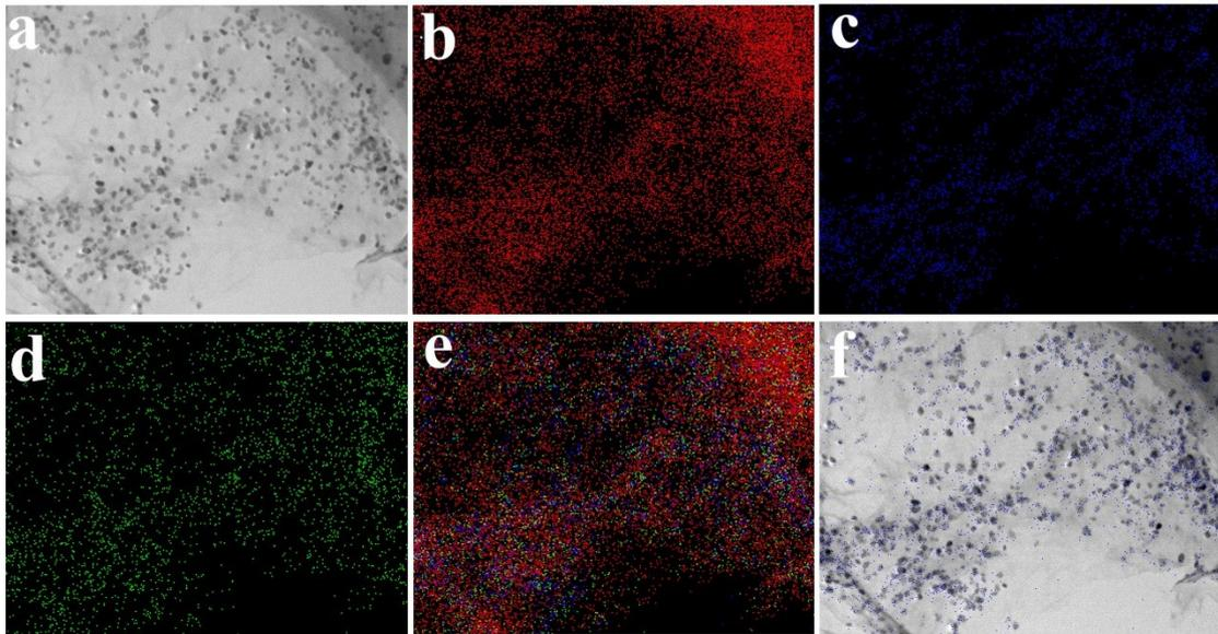
**Figure S3.** (a) The TEM image, (b) C element, (c) Fe element, (d) O element, (e) the overlapping of C, Fe and O elements, and (f) the overlapping of Fe and TEM image mapping images of  $\text{Fe}_2\text{O}_3/\text{GAs}$ .
