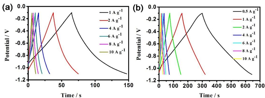
**Figure S10.** Galvanostatic (GS) charge/discharge curves of (A)  $\text{Fe}_2\text{O}_3/\text{GR}$  and  $\text{Fe}_2\text{O}_3/\text{GAs}$  hybrids at different current densities.
