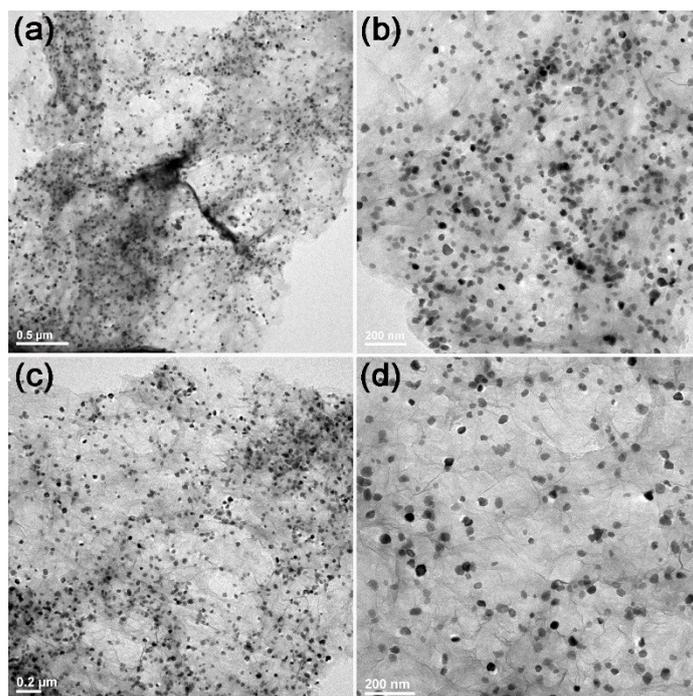
**Figure S8.** (a and b) TEM images of the Fe<sub>2</sub>O<sub>3</sub>/GAs after 5 times cycling test and (c and d) 10 times cycling test.
