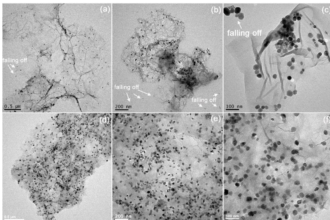
**Figure S4.** TEM images of (a)  $\text{Fe}_2\text{O}_3/\text{GAs}$  prepared by a direct hydrothermal method without a modified Stöber-like treatment, and (b)  $\text{Fe}_2\text{O}_3/\text{GAs}$  prepared by a modified Stöber-like pretreatment and followed by a hydrothermal treatment.
