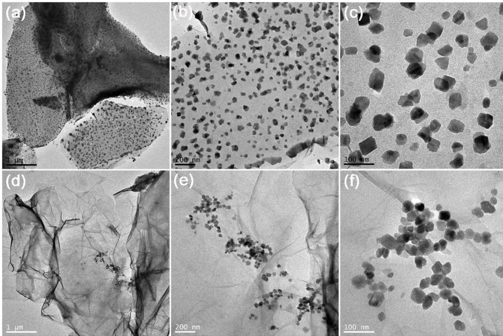
**Figure S7.** (a, b, and c) TEM images of 2D structured  $\text{Fe}_2\text{O}_3/\text{GR}$ , and (d, e, and f) its TEM images after 8 times cycling test.
