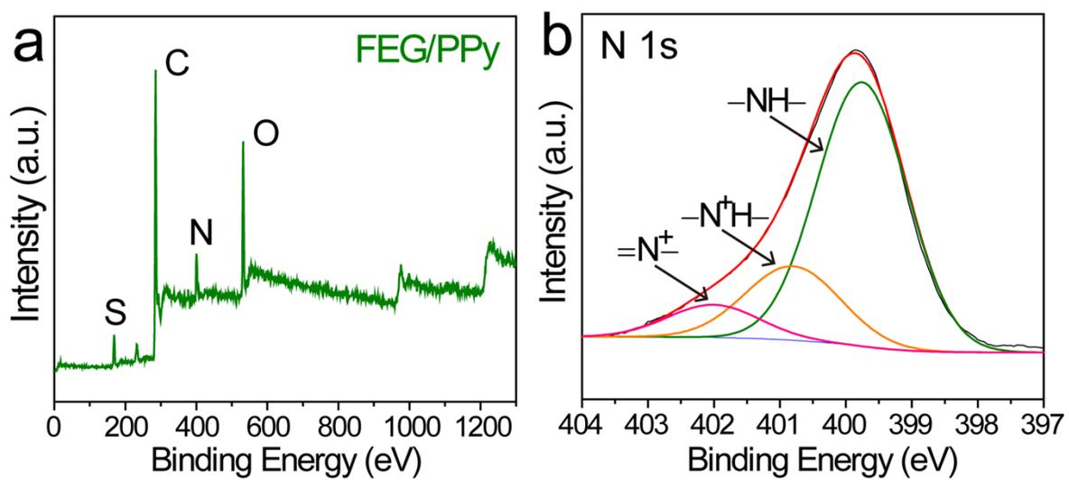
**Figure S2** XPS survey spectrum of FEG/PPy (a) and N 1s spectrum of FEG/PPy (b).
