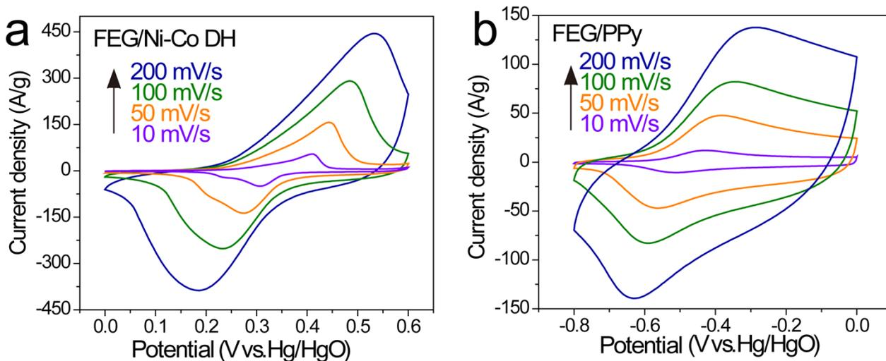
**Figure S3** CV profiles of FEG/Ni-Co DH and FEG/PPy hybrid electrodes.
