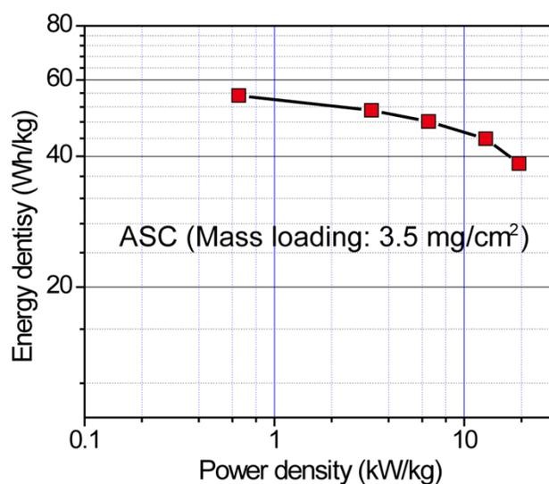
**Figure S9** Ragone plots of ASC with higher active mass loading of 3.5 mg/cm<sup>2</sup>.
