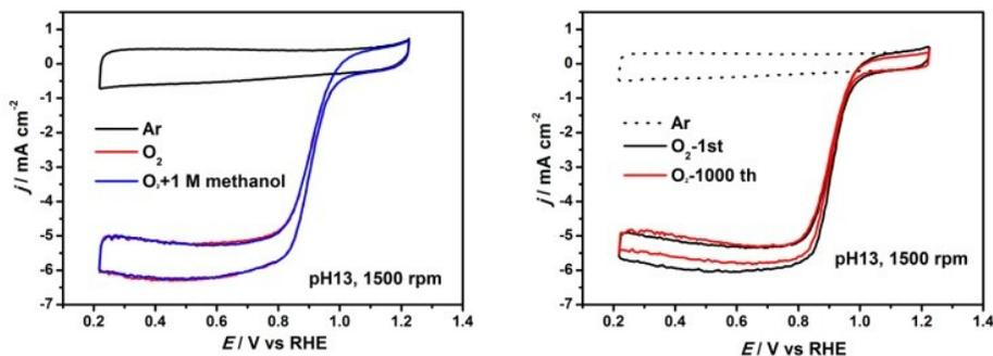
Figure S5 (a) the methanol tolerance effect and (b) stability test of Fe-N<sub>x</sub>/C-1 catalyst in alkaline medium (pH 13).
