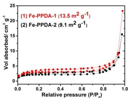
Figure S1 N<sub>2</sub> adsorption/desorption isotherm curves of Fe-PPDA polymers.
