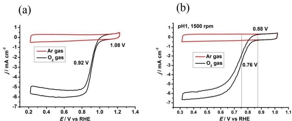
Figure S3 Original polarization curves of Fe-N<sub>x</sub>/C-1 catalyst recorded in (a) alkaline medium (pH 13) and (b) acidic medium (pH 1) saturated with O<sub>2</sub> (black line) and Ar gas (red line).
