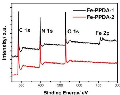
Figure S2 The XPS spectra of Fe-PPDA-1 and Fe-PPDA-2 polymers.
