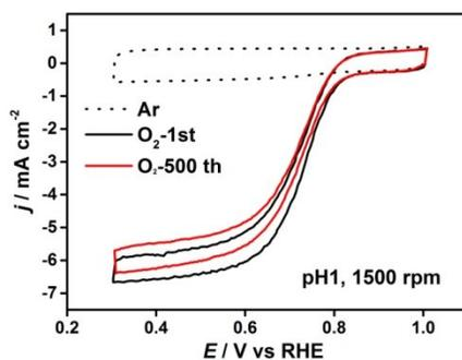
Figure S6 The ORR stability test of Fe-N<sub>x</sub>/C-1 catalyst in acidic medium (pH 1).
