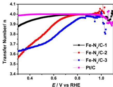
Figure S4 The calculated electron transfer numbers ( $n$ ) of different Fe-N<sub>x</sub>/C materials and commercial Pt/C from Figure 2 with the following equation:  $n = I_d / (I_d + I_r / N)$ .
