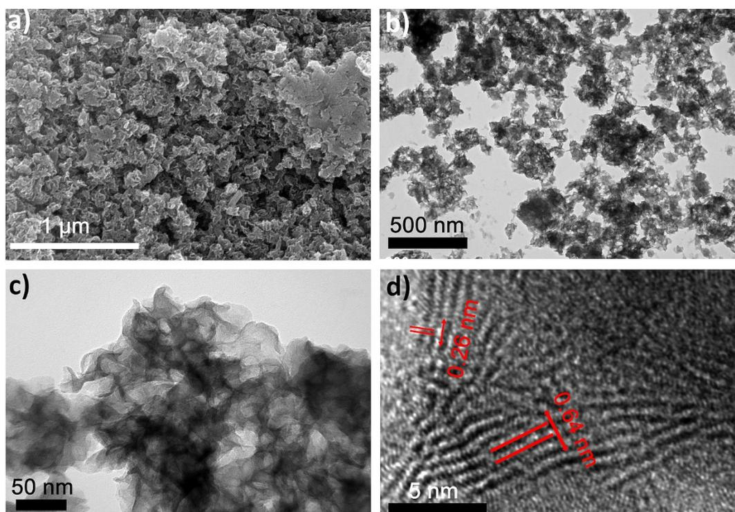
**Figure S5.** (a) SEM image of hydrothermal MoS<sub>2</sub> showing aggregated MoS<sub>2</sub> crystals. (b) and (c) TEM images of hydrothermal MoS<sub>2</sub>; (d) HRTEM image of hydrothermal MoS<sub>2</sub> with layered structures. Lattice spacing of 0.26 nm and 0.64 nm correspond to the (002) and (100) planes of MoS<sub>2</sub> crystals.
