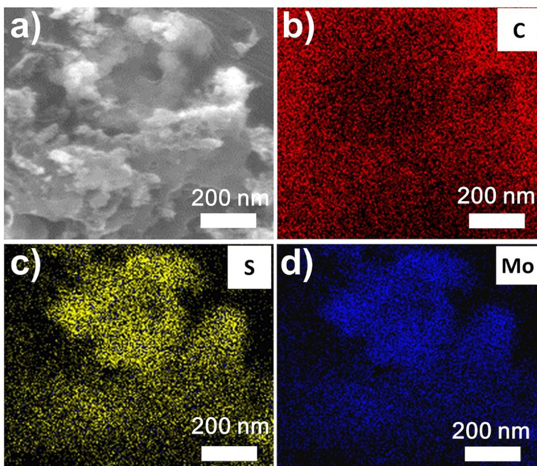
**Figure S3.** (a) SEM image of laser-induced MoS<sub>2</sub>/carbon hybrids; (b-d) Energy dispersive X-ray (EDS) elemental mapping images of elemental C, S, and Mo from the sample shown in (a)
