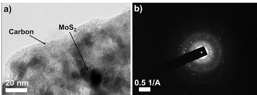
**Figure S4.** (a) TEM image and (b) Selected area electron diffraction (SAED) pattern of laser induced MoS<sub>2</sub>/carbon hybrids. In the electron diffraction pattern, the halo rings are due to amorphous carbon, and bright spots represent MoS<sub>2</sub> nanocrystals.
