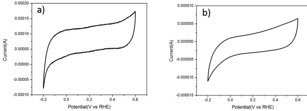
Figure S7. Cyclic voltammetry curves of (a) DLW MoS<sub>2</sub>/carbon hybrids and (c) hydrothermal MoS<sub>2</sub> in 0.5 M H<sub>2</sub>SO<sub>4</sub> vs. RHE at a scan rate of 50 mV/s.
