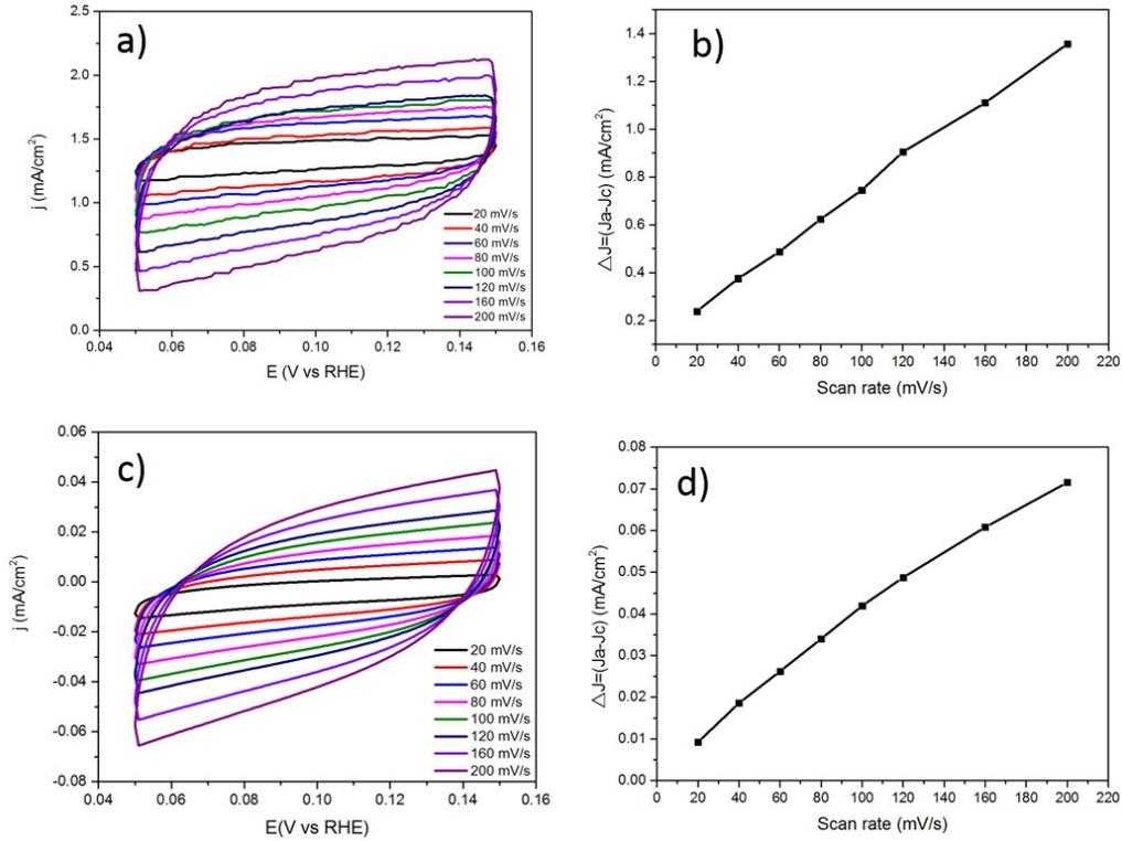
Figure S6. Cyclic voltammetry curves of (a) DLW MoS<sub>2</sub>/carbon hybrids and (c) hydrothermal MoS<sub>2</sub> at scan rates ( $V_b$ ) from 20 to 200 mV·s<sup>-1</sup>. Scan rate dependence of the current densities of (b) DLW MoS<sub>2</sub>/carbon hybrids and (d) hydrothermal MoS<sub>2</sub>.
