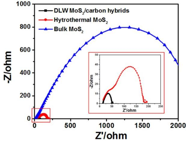
**Figure S9.** Comparison Nyquist plots of bulk MoS<sub>2</sub>, hydrothermal MoS<sub>2</sub>, and laser induced MoS<sub>2</sub>/carbon hybrids. Inset image is enlarged from the area indicated in the red rectangle. Laser-induced MoS<sub>2</sub>/carbon hybrids have the smallest charge transfer resistance, indicating the fastest HER kinetic process.
