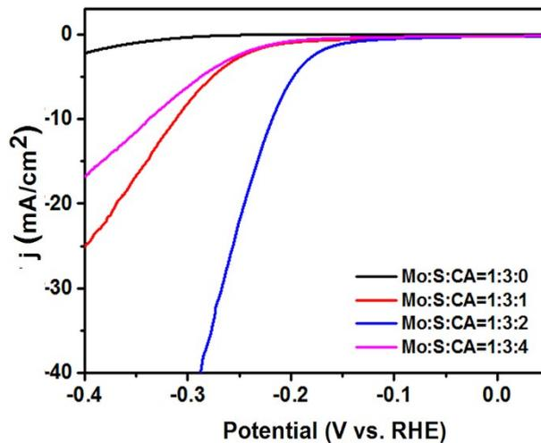
**Figure S8.** Polarization curves of laser induced MoS<sub>2</sub>/carbon hybrids obtained with the different mass ratios of citric acid in Mo: S: CA. The optimal ratio of Mo: S: CA is 1:3:2.
