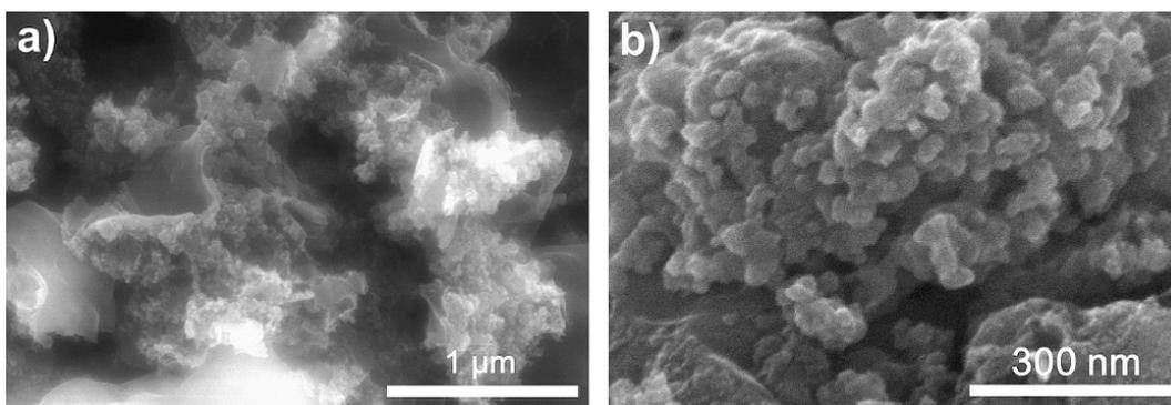
**Figure S2.** SEM images of laser-induced MoS<sub>2</sub>/carbon hybrids, which show that the size of granule is around 30 nm.
