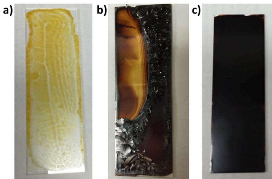
**Figure S1.** Optical images of precursor films with different molar ratios of Mo: S: CA. (a) Mo: S: CA ratio of 1:3:0; (b) Mo: S: CA ratio of 1:3:1; (c) Mo: S: CA ratio of 1:3:2.
