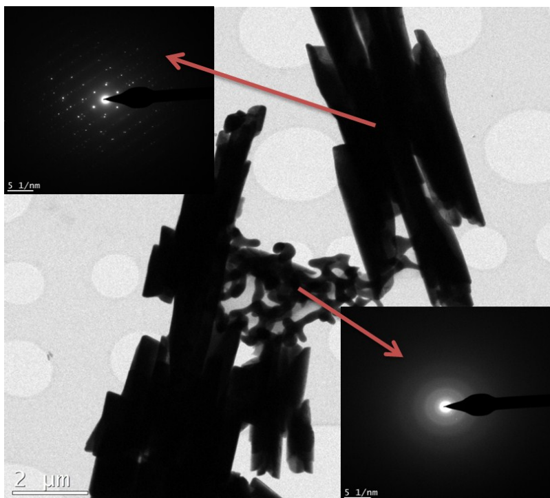
Figure S6. TEM and SAED images of \text{Sb}_2\text{S}_3 NCs, with an injection temperature of 220^\circ\text{C} and a reaction time of just 90s.
