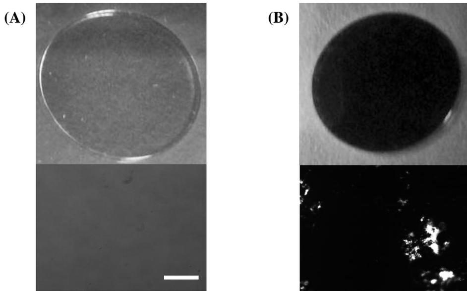
**Figure 4S. Macroscopic and microscopic images of PEG hydrogels with and without CNTs.** PEG hydrogel in the absence of CNTs is a transparent material (A); however, the dispersion of 0.20% w/v CNTs yielded a significant colorimetric difference (B). The microscope images were taken at 10x magnification and the scale bar is 200  $\mu\text{m}$ .
