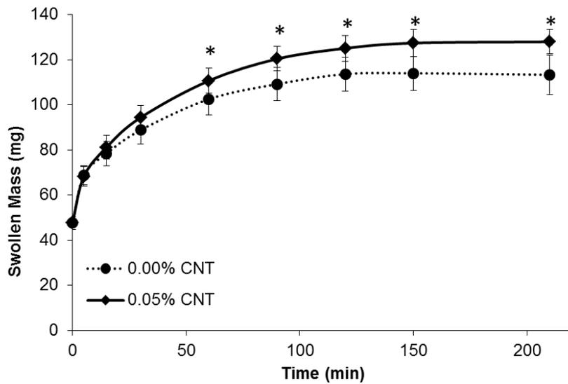
**Figure 2S:** Hydrogel swelling as a function of time for a hydrogel without CNTs (0.00% w/v) and with 0.05% w/v CNTs. Asterisks designate significant difference from the 0.00% w/v condition.
