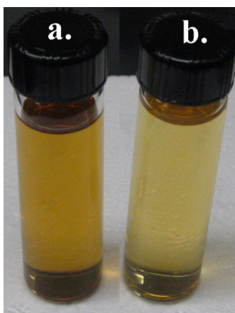
Figure S2. (a) Oleic acid-coated iron oxide nanoparticles are soluble in hexane; (b) oleic acid-free iron oxide nanoparticles are soluble in water after the treatment of our solvent-extraction approach.
