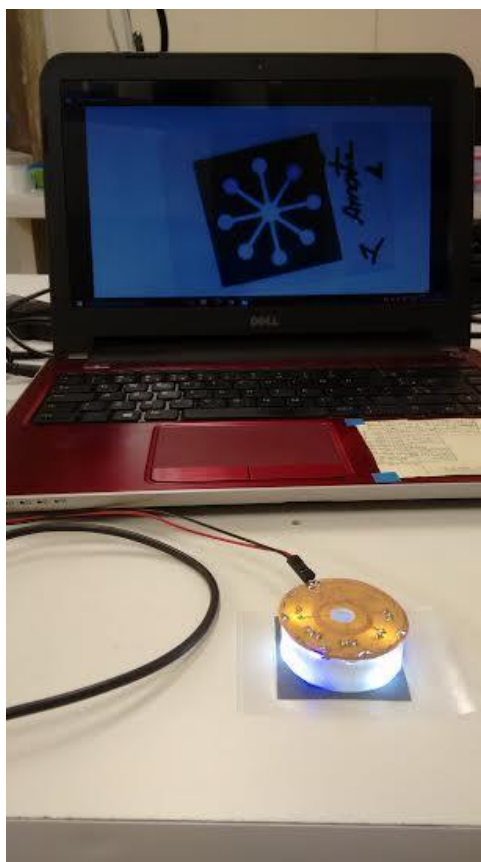
Fig. S1. Presentation of the portable instrumentation explored to promote the simultaneous decomposition with different light sources powered by a USB port from a personal computer.
