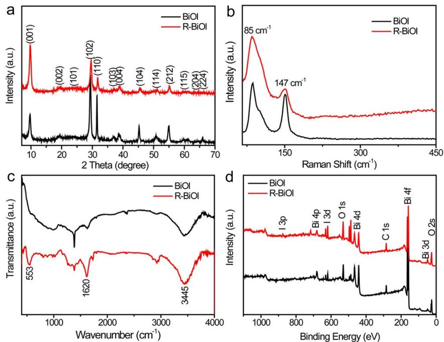
**Fig. S1** Characterization of the BiOI and R-BiOI nanosheets. (a) XRD profiles (b) Raman spectra (c) FT-IR spectra and (d) XPS survey spectra.
