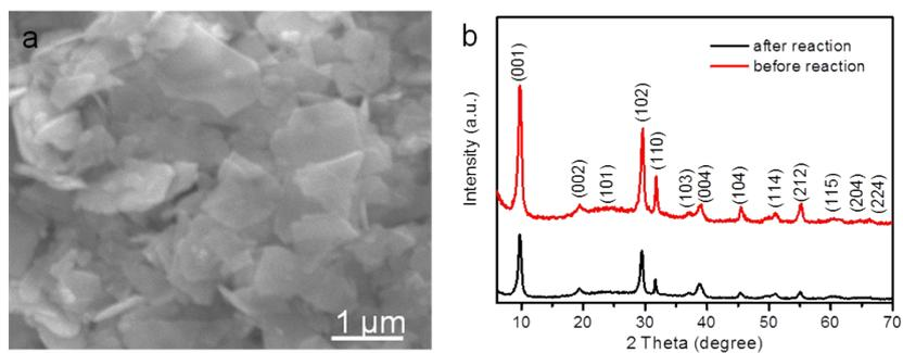
**Fig. S3** (a) SEM image of R-BiOI nanosheets after 5cycles. (b) XRD of R-BiOI nanosheets before and after reaction.
