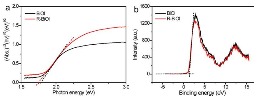
**Fig. S4** (a) plots of the  $(\alpha hv)^{1/2}$  vs photon energy ( $hv$ ) and (b) Valence band comparison of BiOI and R-BiOI.
