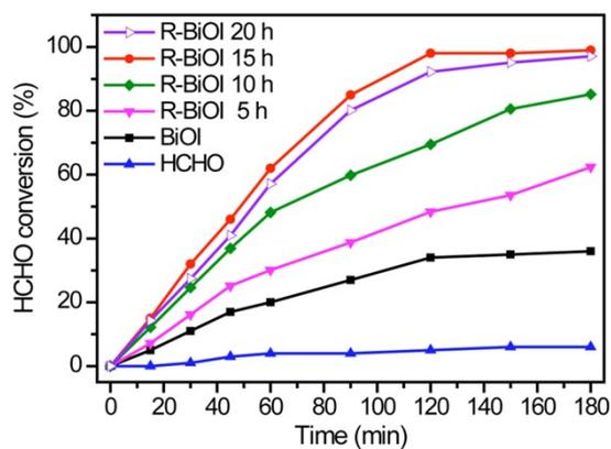
**Fig.S2** Photocatalytic performance of BiOI and R-BiOI samples for degradation of HCHO under visible light irradiation.
