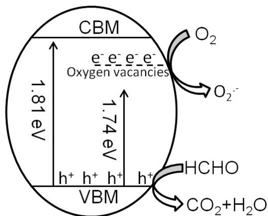
**Scheme S1** Photocatalytic mechanism scheme of R-BiOI catalysts under visible light irradiation.
