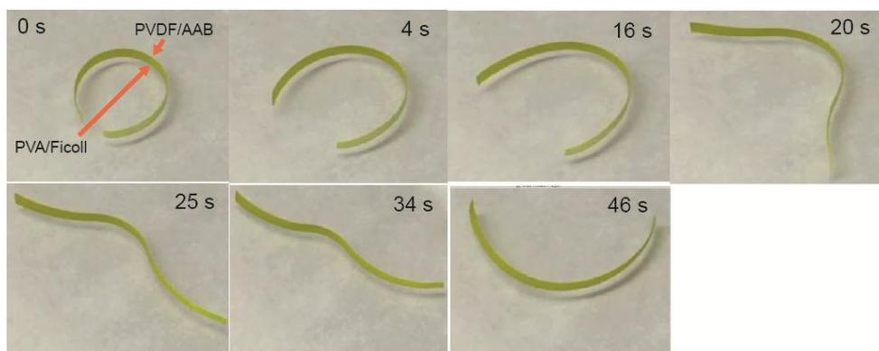
**Figure S3.** Snapshots of the curling of a bilayer strip induced by hydration. A bilayer that was curled by heat (panel labeled 0 s) was immersed in water at 22 °C. The film absorbs water and swells, whereupon it curls toward the PVDF/AAB layer. This curling process is very slow compared to the curling induced by heat.
