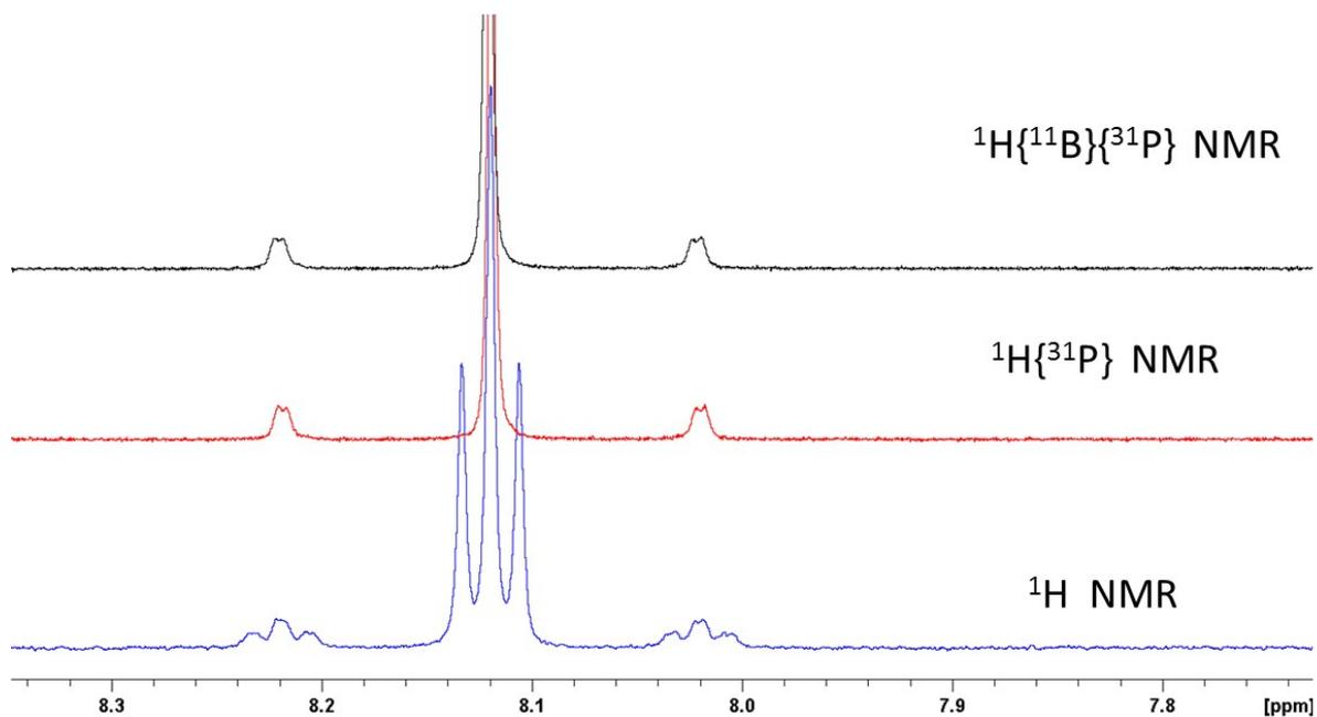
**Figure S4a.** From bottom to top:  $^1\text{H}$  NMR,  $^1\text{H}\{^{31}\text{P}\}$  NMR and  $^1\text{H}\{^{11}\text{B}\}\{^{31}\text{P}\}$  (298K,  $d_8$ -toluene, 500 MHz) spectra for crystals of **1**, showing that the hydride signal is coupling with two phosphorus atoms (see also  $^1\text{H}$ - $^{31}\text{P}$  HMBC experiment, Figure S5).
