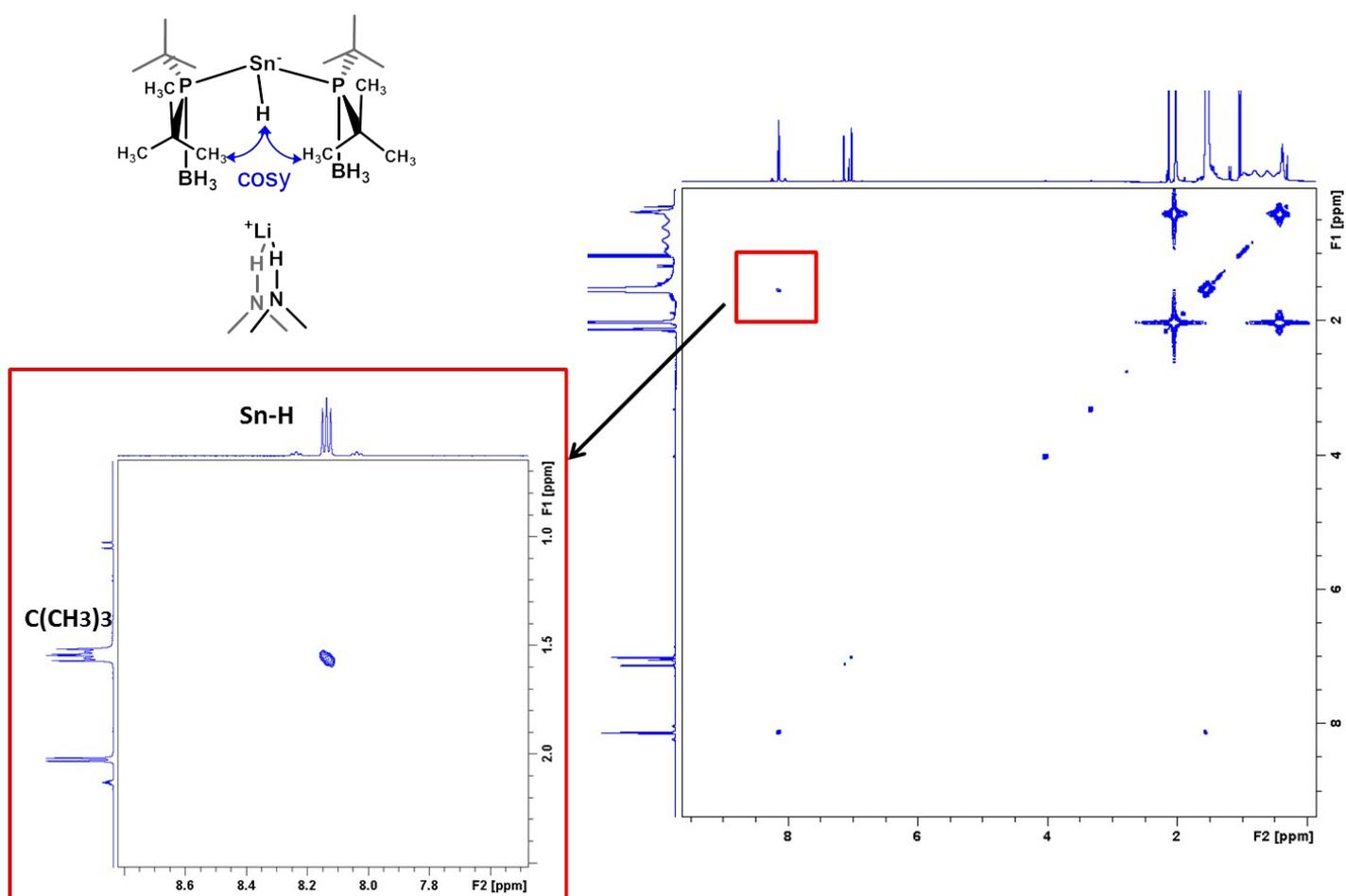
**Figure S8.**  $^1\text{H}$   $^1\text{H}$  COSY NMR (298K,  $d_8$ -toluene, 500 MHz) spectrum for crystals of **1**. Showing that the hydride is only weakly coupled to the  $^t\text{Bu}$  groups and appear as a triplet due to coupling to two phosphorus atoms (see Fig S4a and S5).
