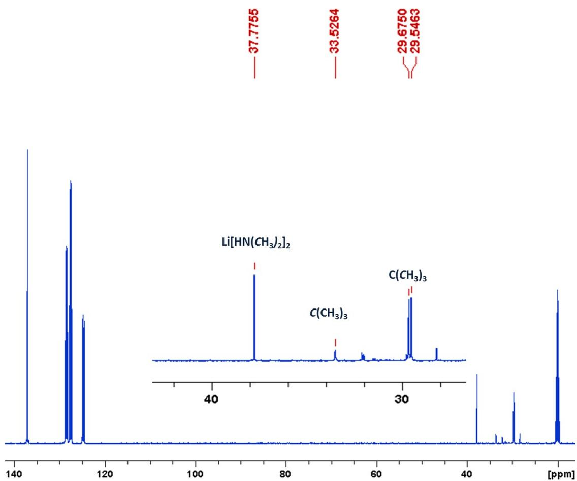
**Figure S6.**  $^{13}\text{C}$  NMR (298K,  $d_8$ -toluene, 125.65 MHz) spectrum for crystals of **1**. Toluene solvent signals at 140-120 ppm.
