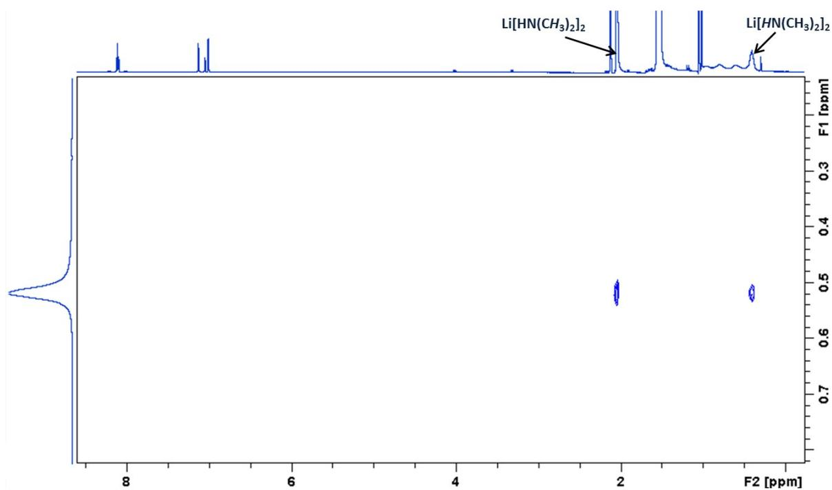
**Figure S14.**  ${}^1\text{H}$   ${}^7\text{Li}$  HOESY NMR (298K,  $d_8$ -toluene, 194.32 MHz) spectrum for crystals of **1**
