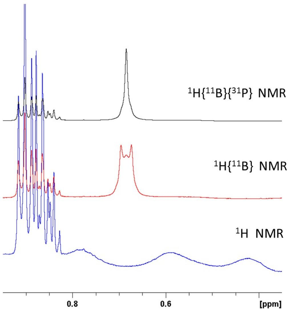
**Figure S4c.** From bottom to top:  ${}^1\text{H}$  NMR,  ${}^1\text{H}\{{}^{11}\text{B}\}$  NMR and  ${}^1\text{H}\{{}^{11}\text{B}\}\{{}^{31}\text{P}\}$  (298K,  $d_8$ -toluene, 500 MHz) spectra showing the P-BH<sub>3</sub> resonance for crystals of **1**, confirming the P-BH<sub>3</sub> linkage. Signals at around 0.85-0.90 ppm are due to decomposition and residual hexane.
