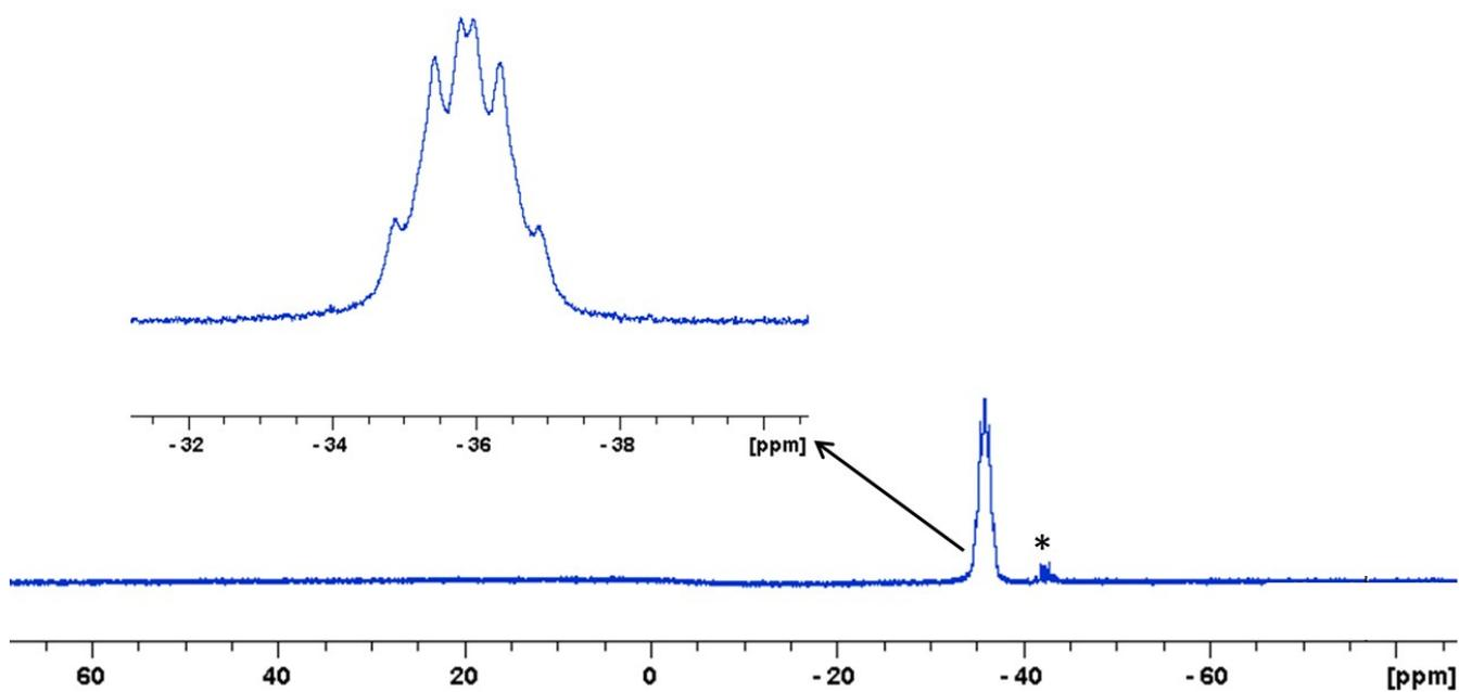
Figure S10.  $^{11}\text{B}$  NMR (298K,  $d_8$ -toluene, 160.35 MHz) spectrum for crystals of **1**. Asterisk (\*) is  $[\text{tBu}_2\text{PH}\cdot\text{BH}_3]$ .
