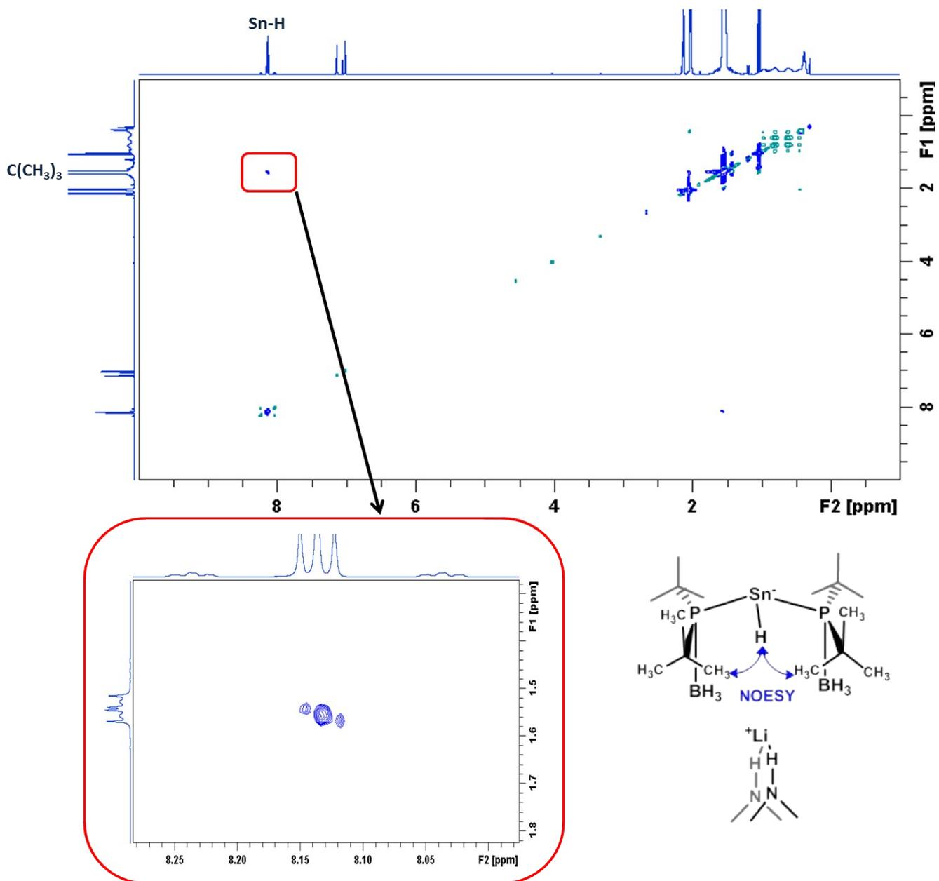
**Figure S9.**  $^1\text{H}$   $^1\text{H}$  NOESY NMR (298K,  $d_8$ -toluene, 500 MHz) spectrum for crystals of **1**, showing that hydride is in near proximity to the  $^t\text{Bu}$  groups.
