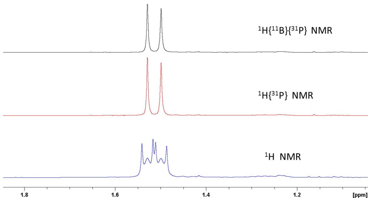
**Figure S4b.** From bottom to top:  $^1\text{H}$  NMR,  $^1\text{H}\{^{31}\text{P}\}$  NMR and  $^1\text{H}\{^{11}\text{B}\}\{^{31}\text{P}\}$  (298K,  $d_8$ -toluene, 500 MHz) spectra showing the  $^t\text{Bu}$  resonance for crystals of **1**, showing the complex coupling pattern due to phosphorus coupling. The two singlets in the  $^1\text{H}\{^{31}\text{P}\}$  NMR spectrum show two different environments for the  $^t\text{Bu}$  protons.
