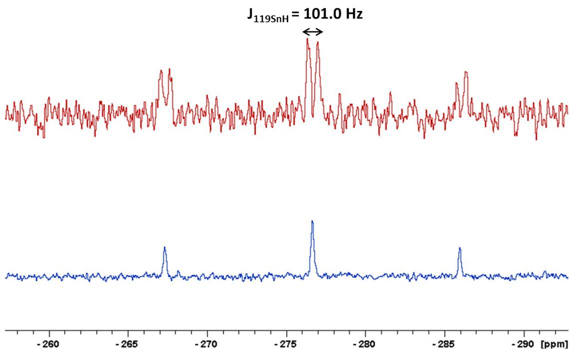
Figure S12.  $^{119}\text{Sn}$   $\{^1\text{H}\}$  and  $^{119}\text{Sn}$  NMR NMR (298K,  $d_8$ -toluene, 186.53 MHz) spectra for crystals of **1**.
