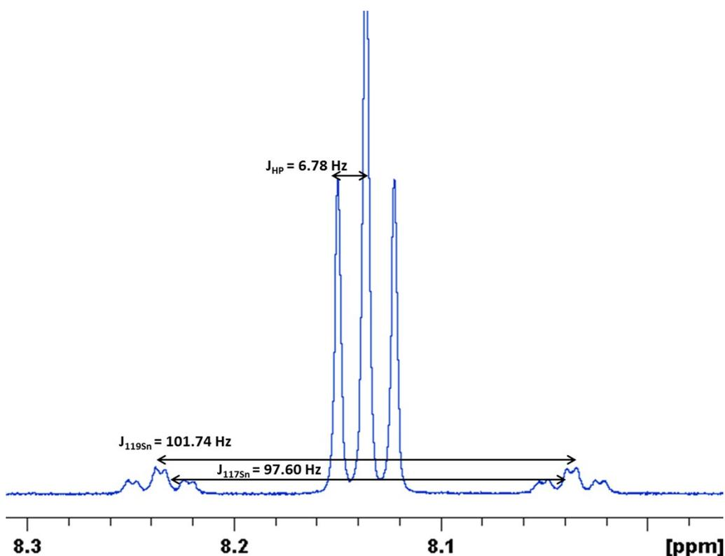
**Figure S3.**  $^1\text{H}$  NMR (298K,  $d_8$ -toluene, 500 MHz) spectrum for crystals of **1** showing the hydride resonance and the satellites due to  $^{119}\text{Sn}$  and  $^{117}\text{Sn}$  coupling,  $J_{117\text{Sn}} / J_{119\text{Sn}} = 0.959$ . The signal appears as a triplet due to  $^2J_{\text{P-H}}$  as confirmed by  $^{31}\text{P}$ - $^1\text{H}$  HMBC (see Fig S6) and  $^1\text{H}\{^{31}\text{P}\}$  experiments (Figure S4a).
