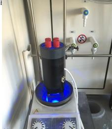
Fig. 1 Reaction apparatus. The blue LEDs photoreactor is equipped with a fan at the bottom to keep the
