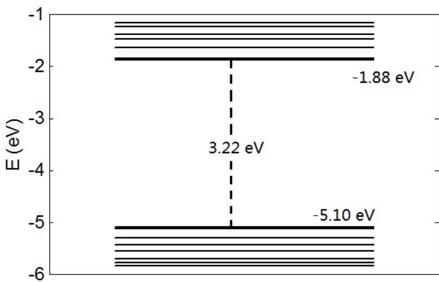
**Figure S5.** Energy diagrams of the frontier MOs of **5**.
