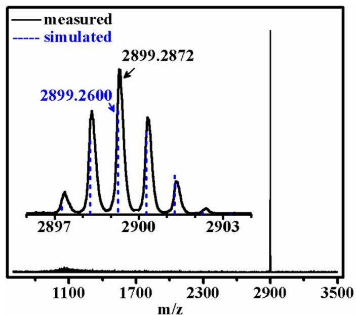
**Figure S1.** HR-MS (MALDI-TOF) and simulated data for compound 5.
