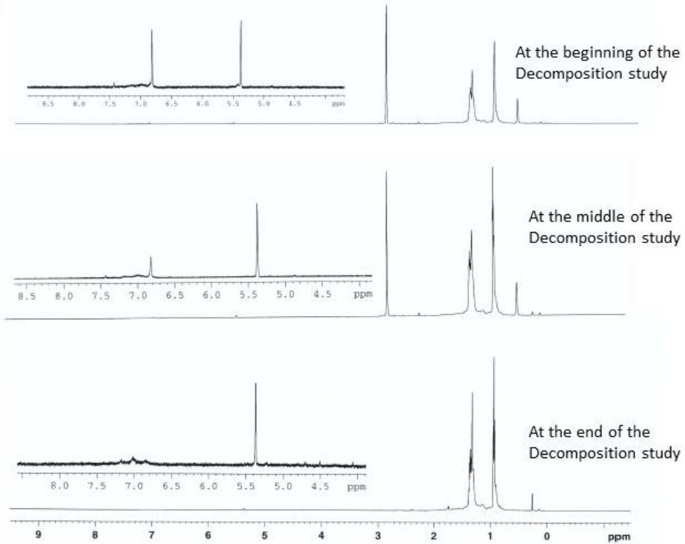
**Figure S9:** <sup>1</sup>H-NMR spectra of the intermediates produce during the decomposition of the  $[\text{WMe}_5^+ \text{B}(\text{C}_6\text{F}_5)_3\text{Me}^-]$  in  $\text{CD}_2\text{Cl}_2$  at  $-20^\circ\text{C}$ .
