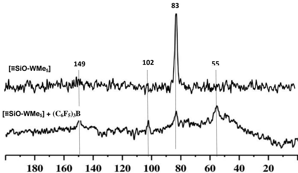
**Figure S8:** a)  $^{13}\text{C}$  CP/MAS NMR spectra of  $^{13}\text{C}$  labeled (50%  $^{13}\text{C}$ )  $[≡\text{SiO-WMe}_5]$ . b)  $^{13}\text{C}$  CP/MAS NMR spectra of  $[≡\text{SiO-WMe}_4^+ (\text{C}_6\text{F}_5)_3\text{BMe}^-]$ . Both spectra were acquired at 400 MHz with a 10 kHz MAS frequency, 1000 scans, a 4 s, repetition delay, and a 2 ms contact time and ambient sample temperature. An exponential line broadening of 80 Hz was applied prior to Fourier transform.
