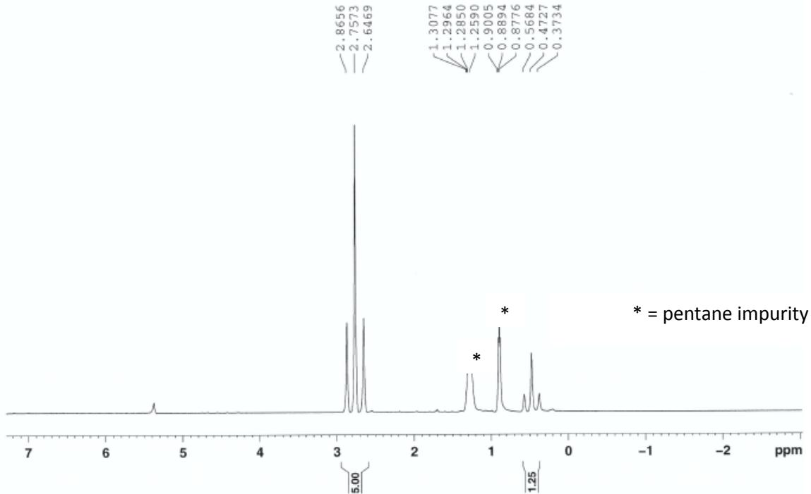
**Figure S6:**  $^1\text{H}$  NMR spectrum of partially  $^{13}\text{C}$  labeled  $[\text{WMe}_5^+\text{B}(\text{C}_6\text{F}_5)_3\text{Me}]$  in  $\text{CD}_2\text{Cl}_2$  (singlet peak at 2.76 ppm and 0.47 ppm is correspond for  $^{12}\text{C}$  coupling with H and a doublet at 2.86-2.65 ppm and 0.56- 0.37 ppm for  $^{13}\text{C}$  coupling with H)
