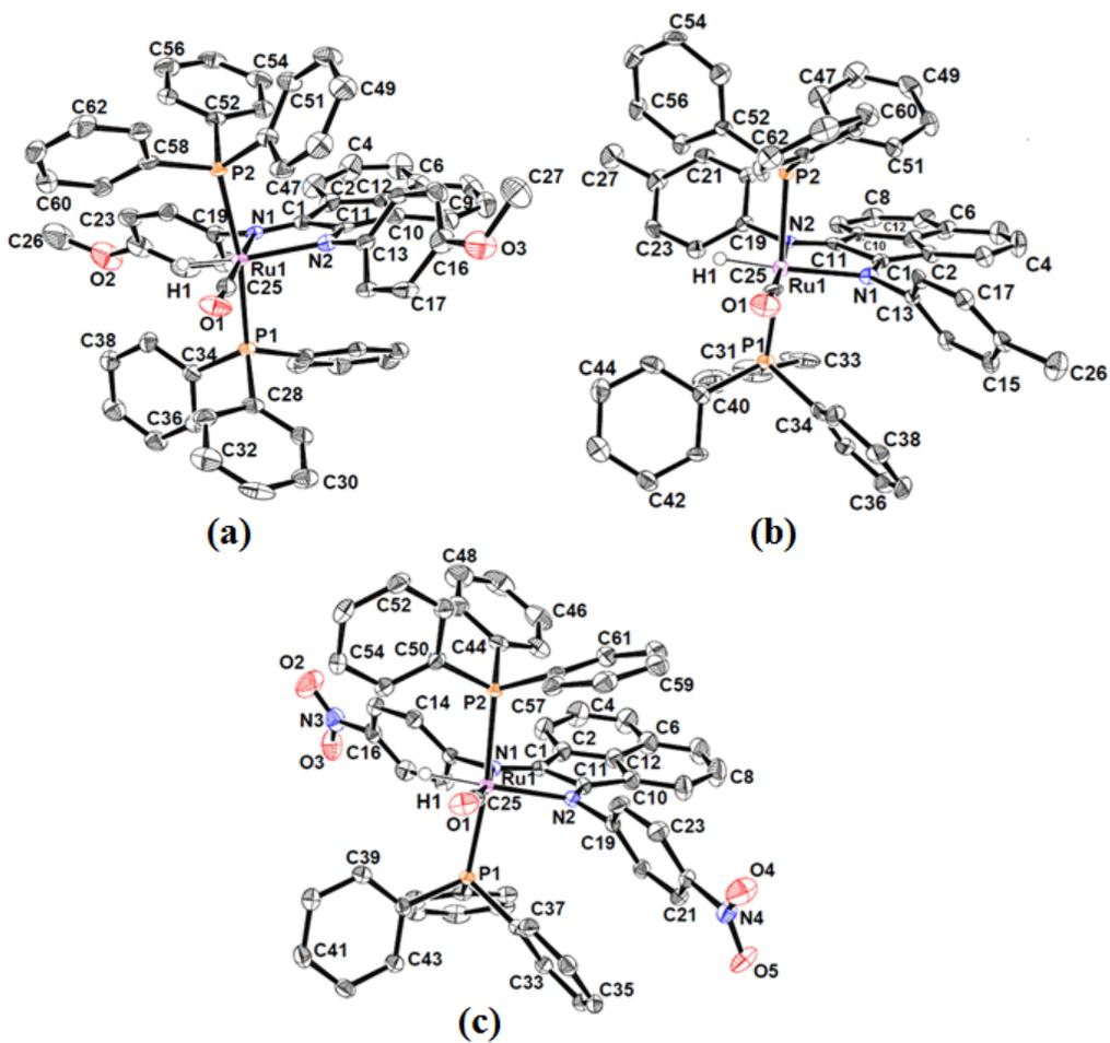
**Figure S6.** ORTEP diagrams of a) **[1a]**ClO<sub>4</sub>, b) **[1b]**ClO<sub>4</sub> and c) **[1e]**ClO<sub>4</sub>. Ellipsoids are drawn at the 50% probability level. Hydrogen atoms (except Ru–H) and ClO<sub>4</sub> anions are omitted for clarity.
