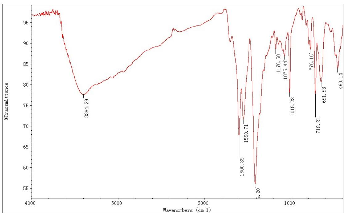
**Figure S4.** FT-IR spectrum of Ir-PMOF-1(Zr).
