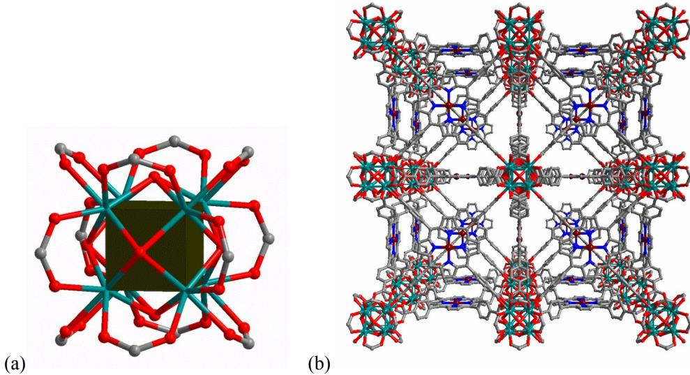
**Figure S6.** Crystal structures of Ir-PMOF-2(Zr): (a) the 12-connected  $Zr_8$  cluster; (b) the 3D framework nets (the axial Cl atoms are removed for clarity). Ir (dark red), Zr (teal), N (blue), O (red), Cl (bright green) and C (gray).
