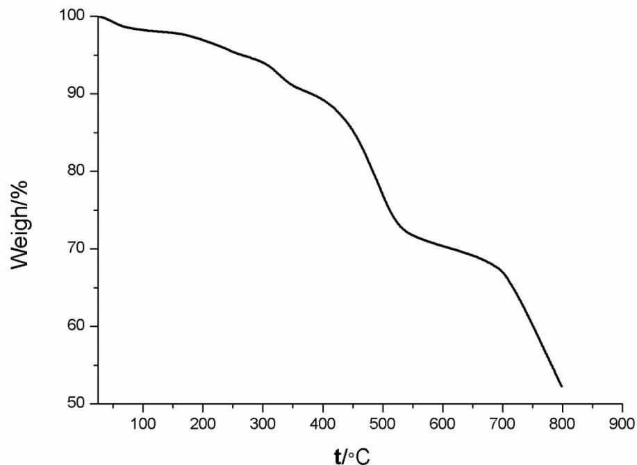
**Figure S7.** The TG curve of Ir-PMOF-1(Zr).
