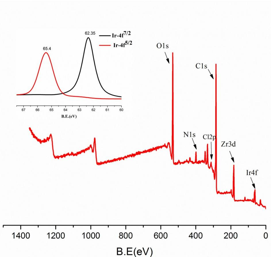
**Figure S3.** XPS spectrum of Ir-PMOF-1(Zr). The insert shows the peaks related to the Ir(III) atoms.
