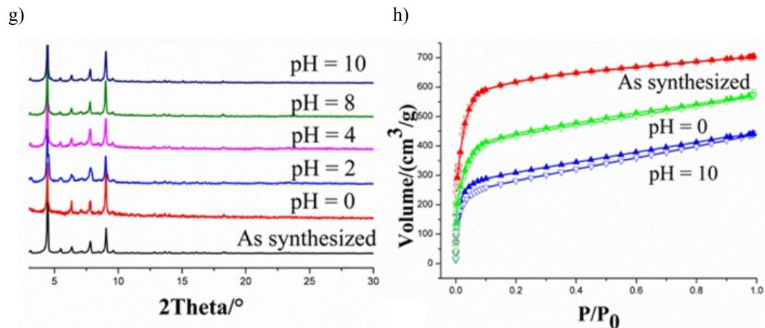
**Figure S8.** The chemical stability study of Ir-PMOF-1(Zr): The PXRD patterns upon treatments in different pH (0-10) aqueous solutions (g) and N<sub>2</sub> adsorption isotherms (h)
