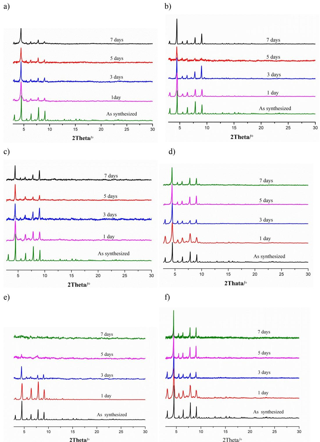
**Figure S8.** The chemical stability study of Ir-PMOF-1(Zr): The PXRD patterns upon treatments in different solvents for 1, 3, 5 and 7 days: a)  $\text{PrOH}$ ; b) acetonitrile; c) toluene; d) hexane; e) water; and f) DCM.
