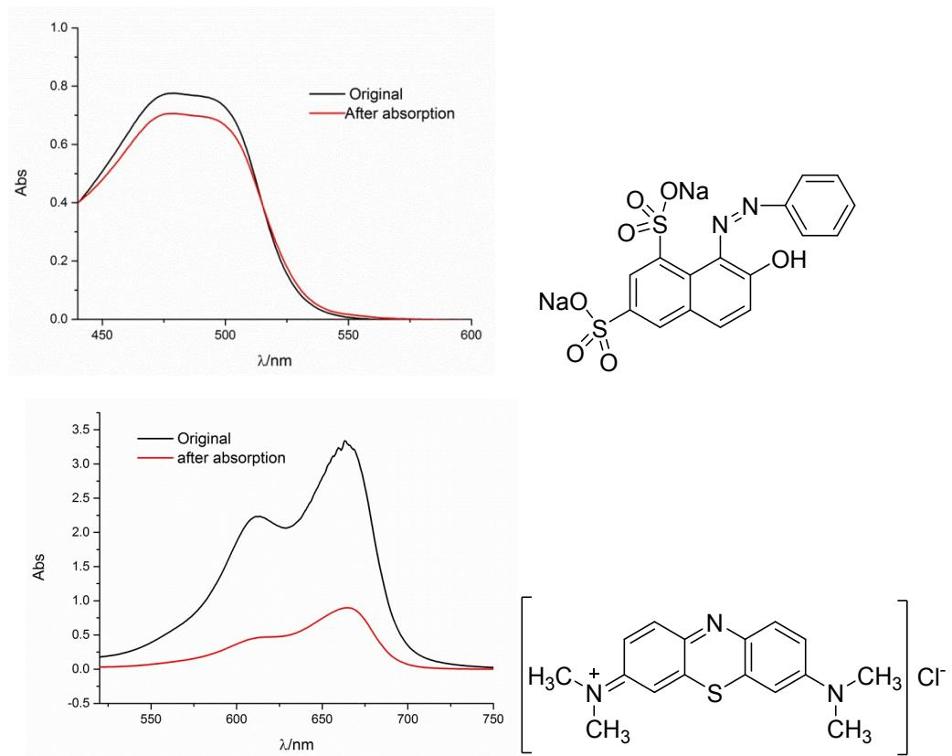
**Figure S9.** The UV-vis spectra for the dye uptake experiments of OG (up) and MB (down) for Ir-PMOF-1(Zr).
