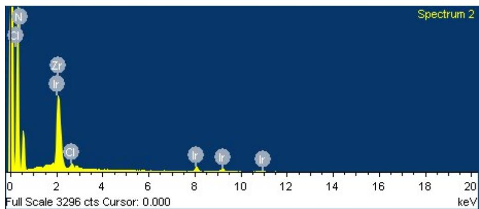
**Figure S2.** EDS spectrum of Ir-PMOF-1(Zr).
