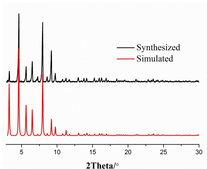
**Figure S5.** The experimental and simulated PXRD patterns of Ir-PMOF-1(Zr).
