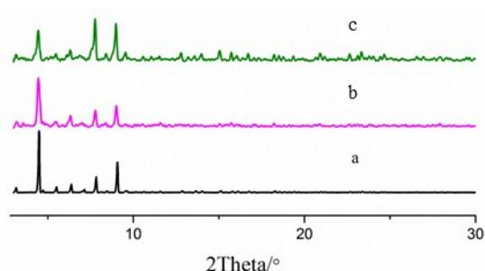
**Figure S10.** The PXRD patterns for Ir-PMOF-1(Zr) of as synthesized sample (a), after catalytic O-H insertion reactions (the first run (b) and the tenth run (c)).
