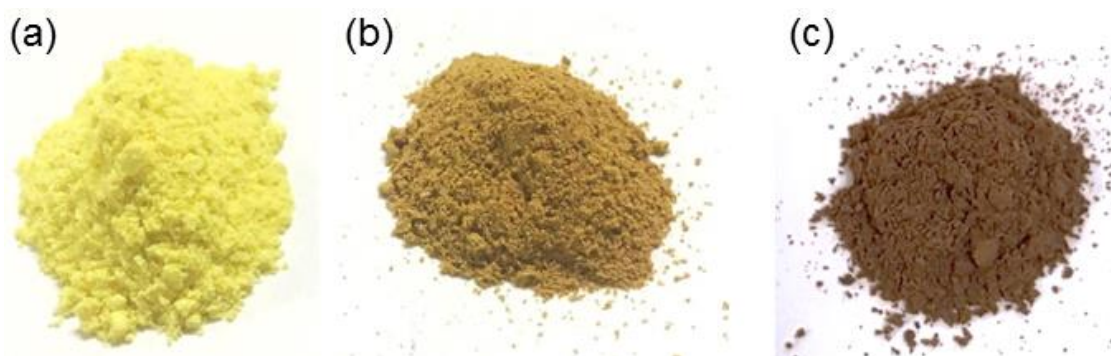
Figure S2: Photographs of thiol-modified MIL-53(Al) (Product B) before (a) and after addition of iodine (b) from chloroform solution and (c) from vapour.
