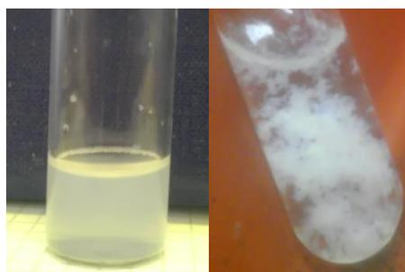
**Fig. S5.** pNIPAAm<sub>120</sub>-*b*-pAMPTMA<sub>30</sub>/Na-tbutPhC mixture with total charge concentration of  $2.0 \times 10^{-3}$  M and  $x^- = 0.50$  at 25 °C (left) and 35 °C after 8 hours (right).
